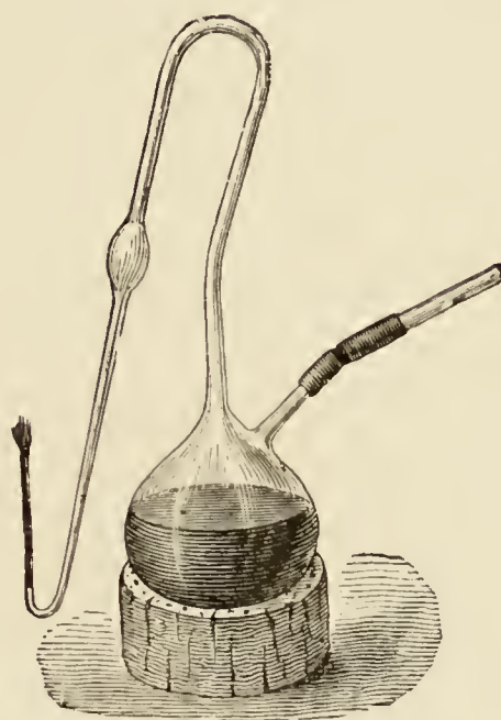
FIG. 161.—Pasteur Flask, with Hansen's improved modification by widening the swan-neck tube. About one-fifth natural size. (After Hansen.)
