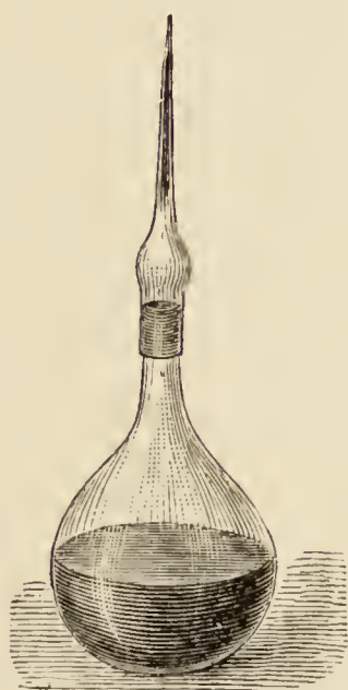
FIG. 160. Chamberland Flask. About one-fifth natural size. (After Hansen.)
