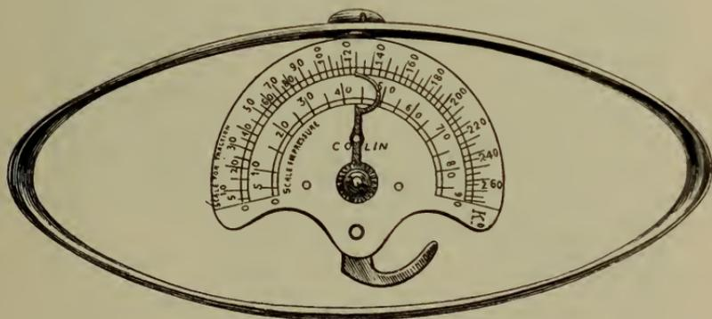
FIG. 17.—Dynamometer to determine the strength of the flexors of the forearm.
