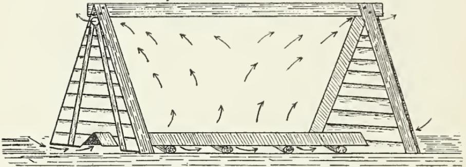
Frame of Potato House, Showing Ventilator in position.
