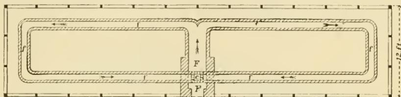
FIG. 4. Sweet-potato bed, with furnace and flues.
