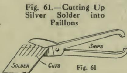
Fig. 61.—Cutting Up Silver Solder into Paillons
