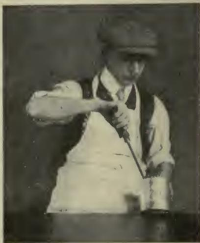
Fig. 21.—Soldering on Can Bottom Internally
