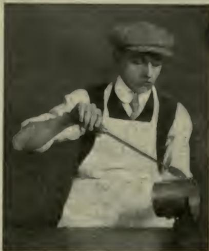
Fig. 22.—Soldering Can Externally
