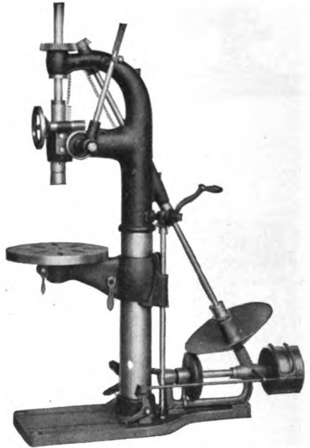
No. 2—Will drill 1\frac{1}{4} in. hole in cast iron 1 inch deep in one minute, with wheel feed.
