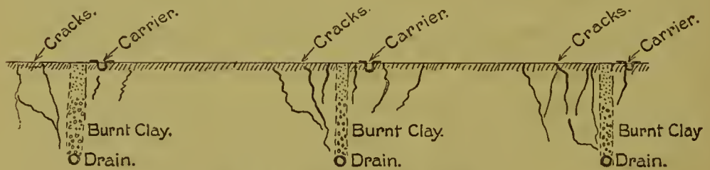
Fig. 11.—Cracking of clay soils.
