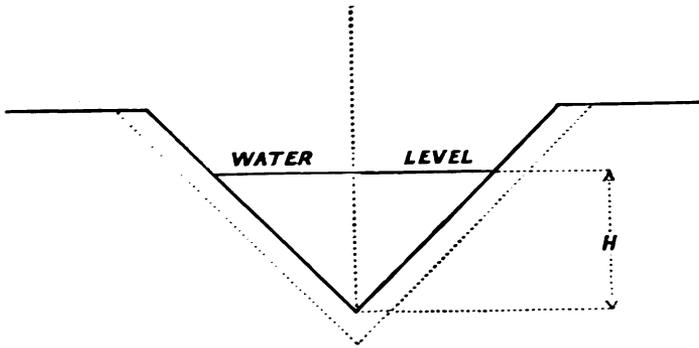
in a V notch is as the square of the height from the vertex, and the volume discharged as the  $\frac{5}{2}$  power of that height. The formula is
