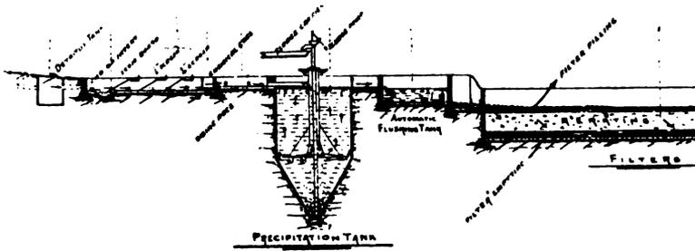
FIG. 21. PLAN SHOWING SETTLING TANK AND DORTMUND TANK FOR PRECIPITATING BEFORE FILTRATION.
