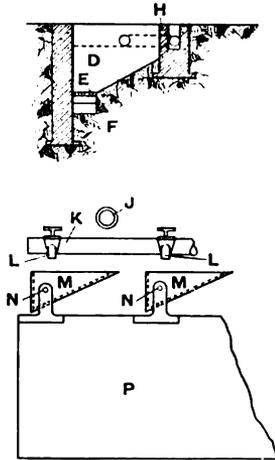
A, Raw Sewage inlet; B, Grit chamber; D, Cultivation tank; H, Outlets to channel J; P, Nitrifying trays; M, Tipplers.
