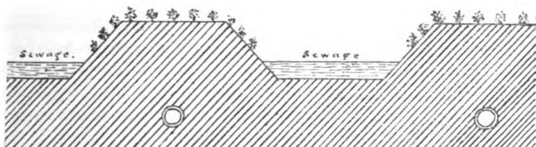
FIG. 14.—SECTION SHOWING UNDERDRAINS IN IRRIGATION.
