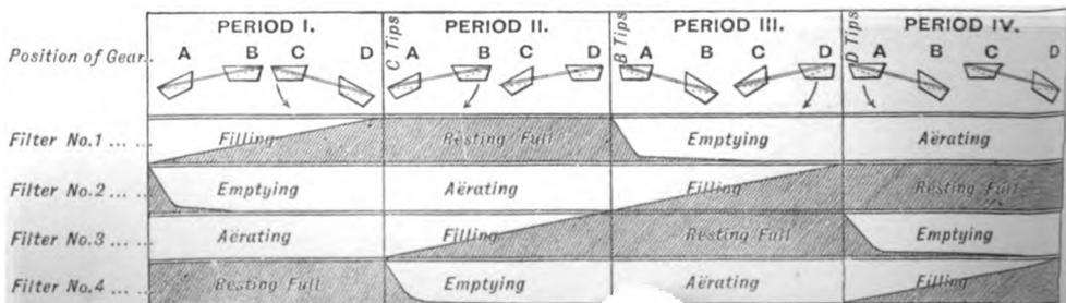
FIG. 34.—WORKING OF CAM AND GEAR.
