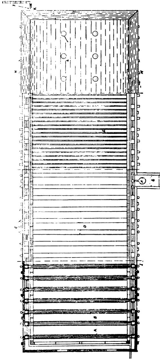
FIG. 28.—SECTIONAL PLAN OF DUCAT'S FILTER.
