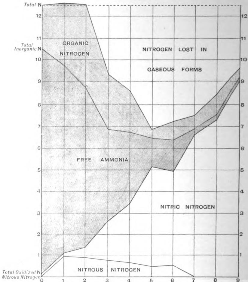
FIG. 39.—CHANGES OF NITROGEN IN OXIDIZING TRAYS
