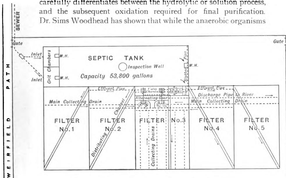
FIG. 35.—PLAN OF BELLE ISLE SEWAGE WORKS, EXETER
