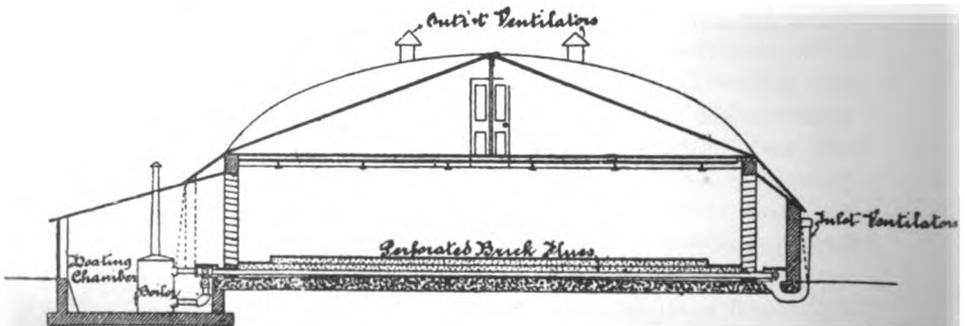
FIG. 25.—SECTION OF DUCAT'S BACTERIAL SELF-ACTING FILTER.
