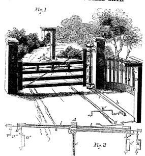
pending. A person advancing from either catch and rod, so that when the catch is side of the gate, can, by pulling one of these weights, cause the gate to open, and by doing the same when through, the gate will close behind him, there being no necessity that he should dismount if on horseback.
