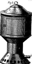
Among the numberless applications of coal, | view, and Fig. 2 a section,) is intended for this and other gas to the comfort and use of man, there is not one superior to gas as a heater. It is so cleanly, so easily lighted, so cheap, and gives so much warmth, that any device for radiating all the heat given out in combustion must be acceptable.
