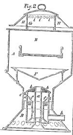
purpose, and its peculiar features we will now describe. In the perspective view, only the external parts are seen, which are: D, a conical shaped base, perforated with holes to admit the amount of external air necessary for the combustion of the gas; h, a pipe of F carries it round to D'; the passage is lustrations (of which Fig. 1 is a perspective having a door, and H, a more or less closed
