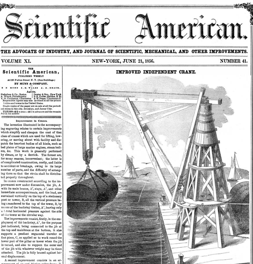
rangement of an anti-friction roller frame, D, in combination with the foot piece, C, so as to reduce friction, and prevent the binding of the foot piece against the tower.
