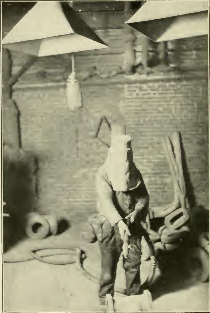
FIG. 15. A SPECIAL CHAMBER FOR SAND-BLASTING.
