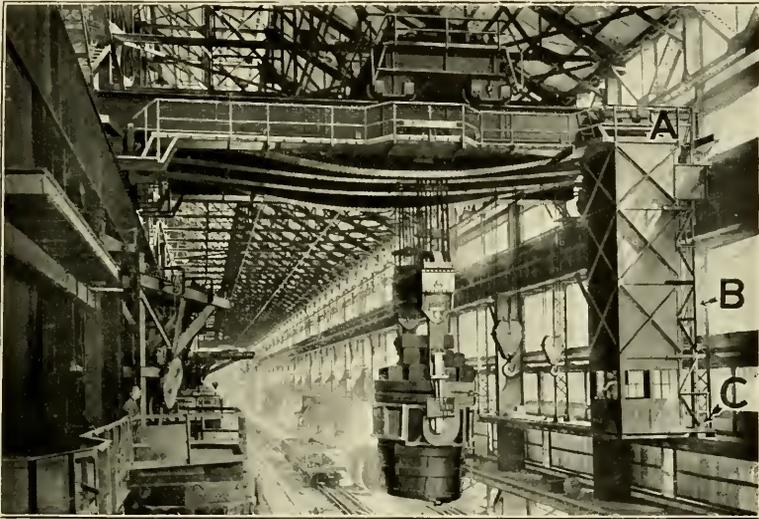
FIG. 11. SAFEGUARDS ON A LARGE LADLE CRANE.
