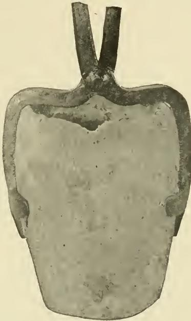
FIG. 10. TONGS PROPERLY APPLIED TO A CRUCIBLE, FOR REMOVING IT FROM A STATIONARY FURNACE.
