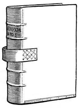
Fig. 4.—Showing Strap for Pulling Heavy Books from the shelf, and also METAL SHOE at the bottom of the boards to protect the leather.
