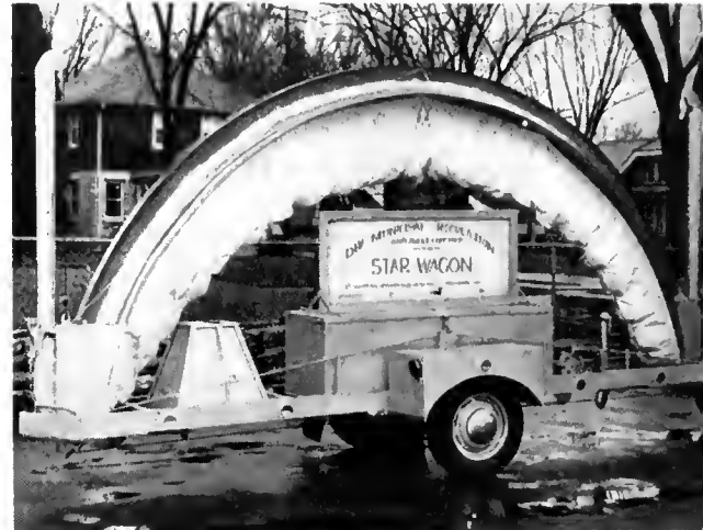
The twenty-one-foot-long Starwagon is placed in position for raising and opening its foldup dome.
