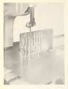
Figure 14.--Smear remover space guide attached to the power saw.
