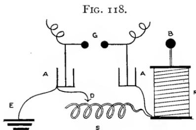
Showing connections for resonator.
