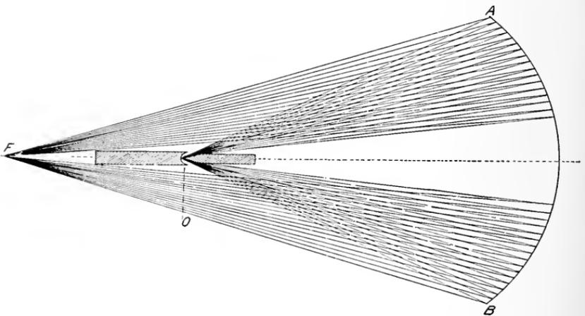
Illustrating loss of light for reflectors by the interposition of the carbons.
