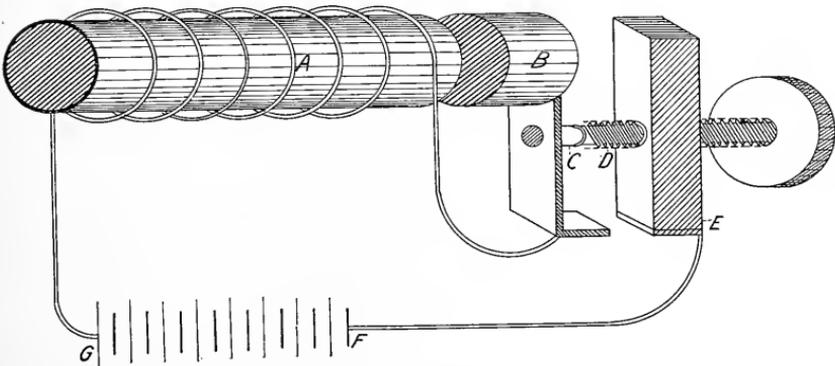
Showing detail construction of primary coil, with vibratory interrupter.
