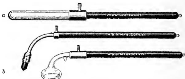
Vacuum electrodes: *a*, glass cone filled with metal filings coated with silver upon the inner surface; *b*, carbon point for single spark.
