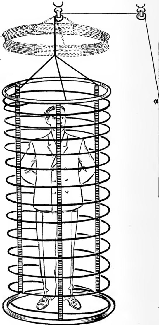
Cage solenoid for autocondensation.
