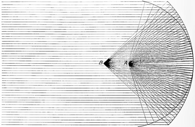
Showing the determination of strength of concentration for reflectors of the same size, but different curvature.
