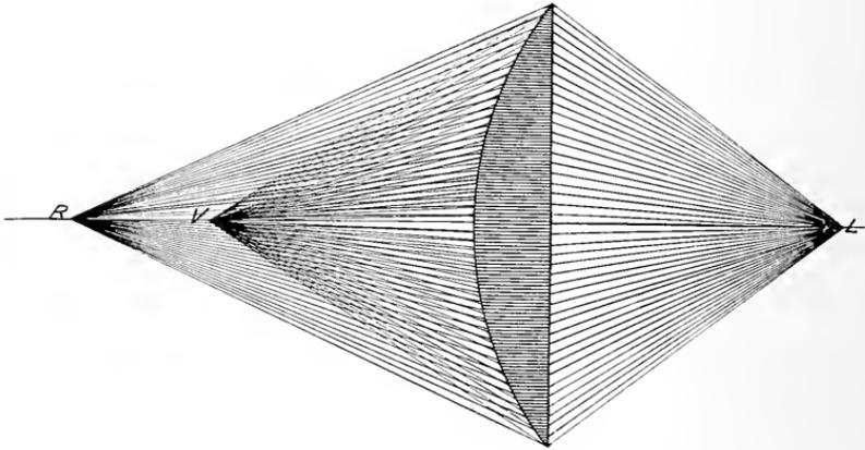
Illustrating the different foci of chemical rays (*V*) and the heat-producing rays (*R*).
