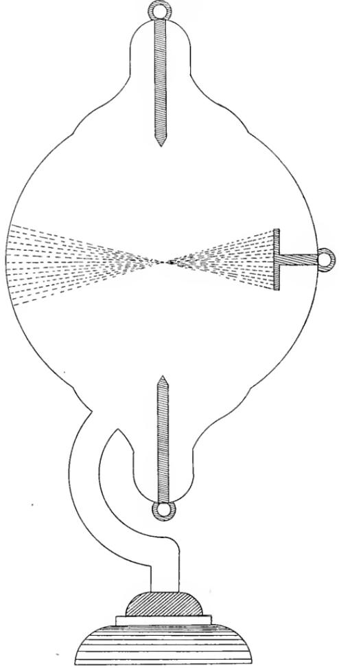
Crookes' tube of a higher vacuum.
