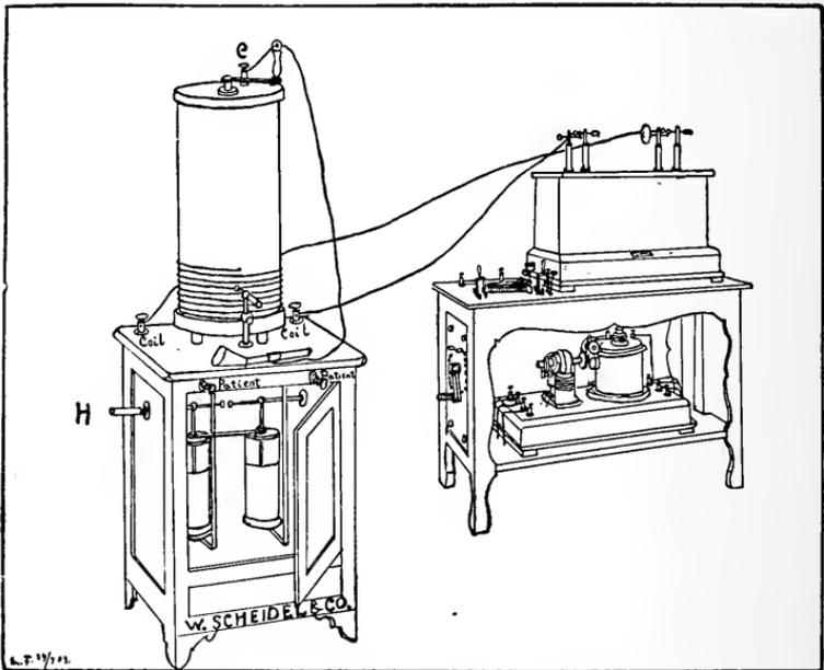
Oudin type of resonator operated by coil.
