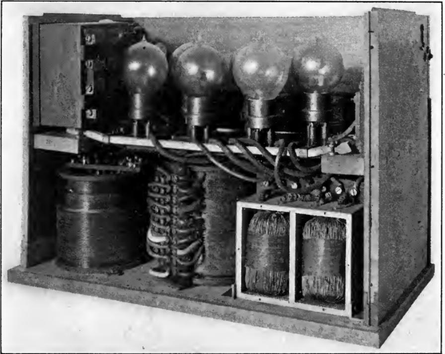
**Plate 10.**—A typical undamped wave two-way set of French design. Note that the six vacuum tubes used as detector, oscillators and amplifiers are all identical. The amplifier iron core transformers are seen at the lower right hand corner, and at the left are the transmitting and receiving inductances.
