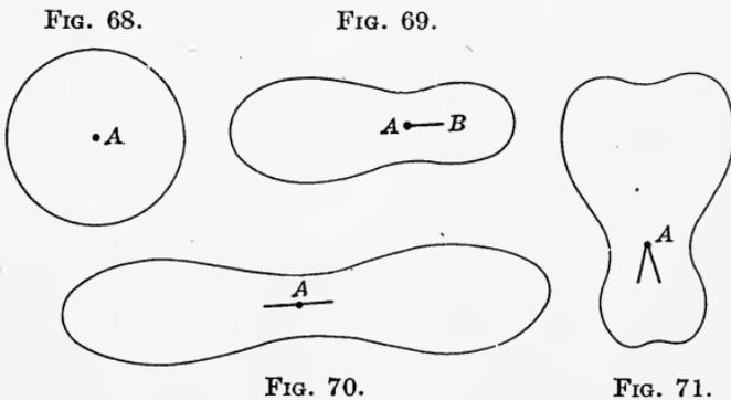
antenna. Assume also that each one of these receiving circuits has some device which permits of measuring the current induced in it when the antenna circuit *A* is oscillating. Now if the observers move toward or away from the antenna *A* until they all obtain the same current reading in their receiving circuit, they will finally find themselves on a circle having *A* as its center. This shows that a vertical wire antenna radiates with equal strength in all directions.
