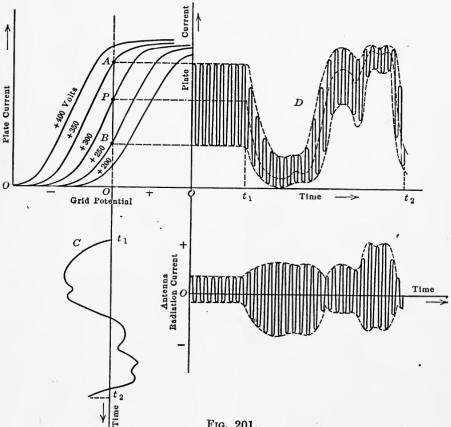
power vacuum tube, modulate these oscillations by means of a similarly low-power vacuum tube modulator, such as described above, and then amplify the modulated high frequency oscillations by a vacuum tube cascade or pyramid radio frequency amplifier before impressing them upon the antenna circuit. The important factor here is obviously that the oscillations be amplified without distortion. This consideration is taken up in a later section of this chapter.
