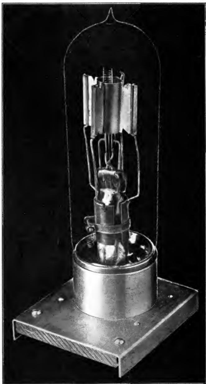
**Plate 4.**—Three-electrode vacuum tube used as high power oscillator and modulator. The plate has been forced downward to expose the grid and filament axially mounted. Note the cooling flanges on the plate. Signal Corps tube type VT-18.
