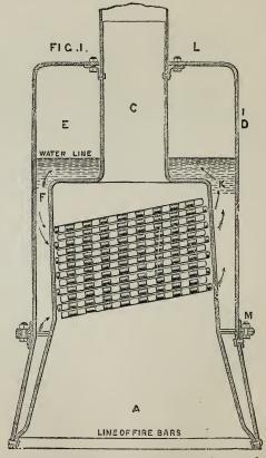
proved to 300 lbs., and the engines may be worked with the greatest safety at a pressure of 150 lbs. on the square inch.
