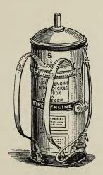
The fire-exterminator appears outwardly as shown by the engraving, and is arranged so that it can be speedily and easily carried on a man's back. There are various details as to the inner structure which need not be given here, but in brief it has inside it a solution of carbonic acid gas. It may be called a large soda-water bottle charged with gas and incombustible chemicals under great pressure.
