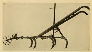
Fig. 9.—V-shaped cultivator with five rather large teeth or shovels. This type of cultivator is especially valuable where the weeds have gotten a start in the plantation.
