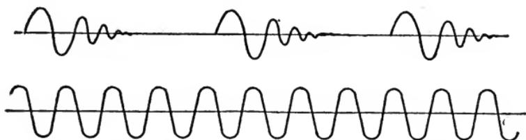
**A schematic comparison between damped and undamped waves. The damped waves, shown above, consist of wave groups or wave trains, while the undamped or CW waves are of uniform height and wave length and without a break.**
