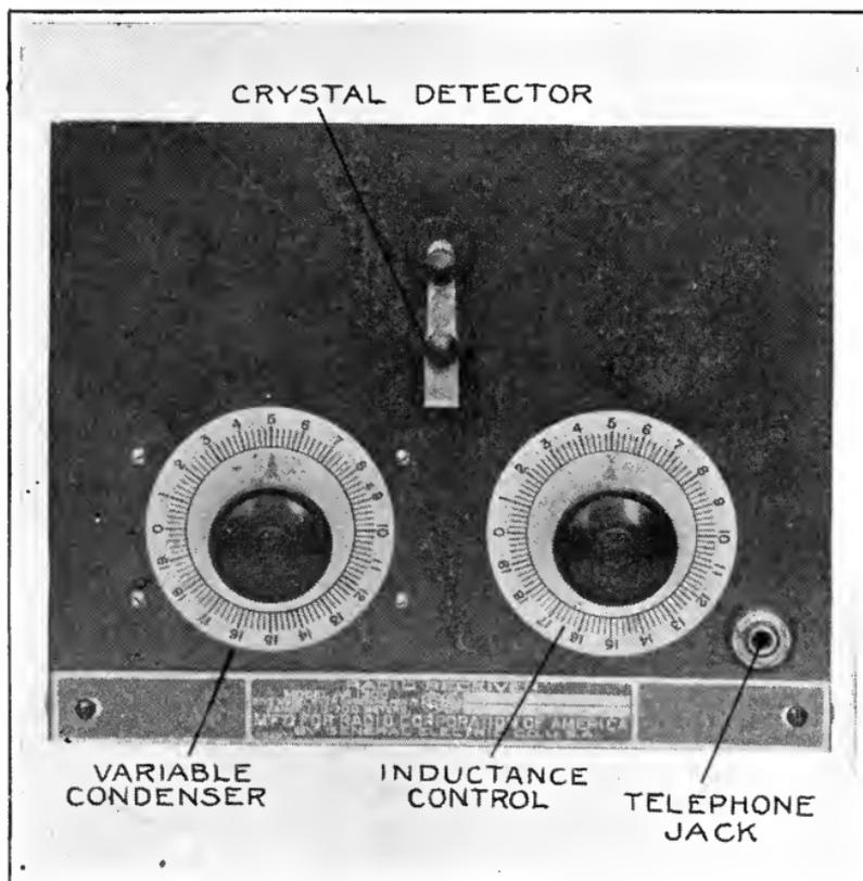
Front view of receiving set shown on page 127. The cabinet of this set is made of metal instead of the usual wood.
