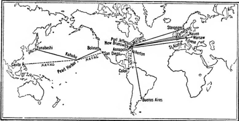
**Our American scheme for world-wide radio communication. Every station shown in this map is either in operation or under construction, and by far the greater portion of the stations are those already in operation.**
