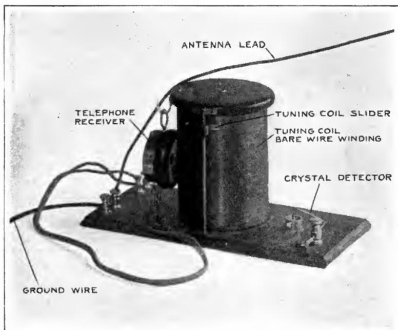
**Receiving set of simple construction, making use of a tuning coil with single slider, a crystal detector, and a single telephone receiver. This set may be used for short distances.**
