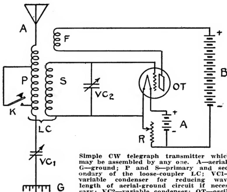
Simple CW telegraph transmitter which may be assembled by any one. A—aerial; G—ground; P and S—primary and secondary of the loose-coupler LC; VC1—variable condenser for reducing wave length of aerial-ground circuit if necessary; VC2—variable condenser; OT—oscillating tube; A—filament battery; R—filament rheostat; B—filament battery; F—feed-back or tickler coil.
