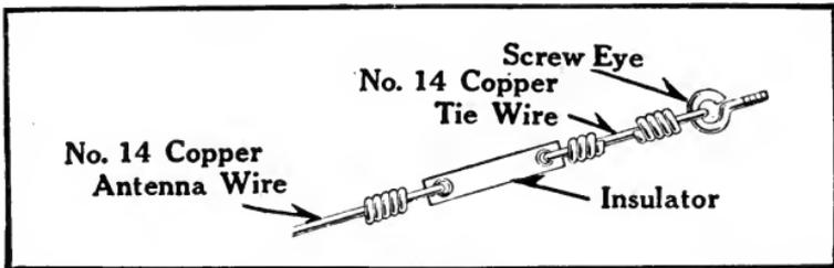
Simple way to insulate and fasten the farther end or free end of a single wire antenna.
