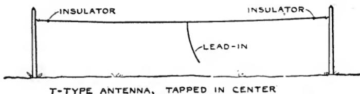
**Arrangement of a T-type single wire antenna. When the antenna runs longer than 150 feet, it may be desirable to tap it in the center for the lead-in, provided the lead-in can be dropped straight down to the receiving apparatus.**
