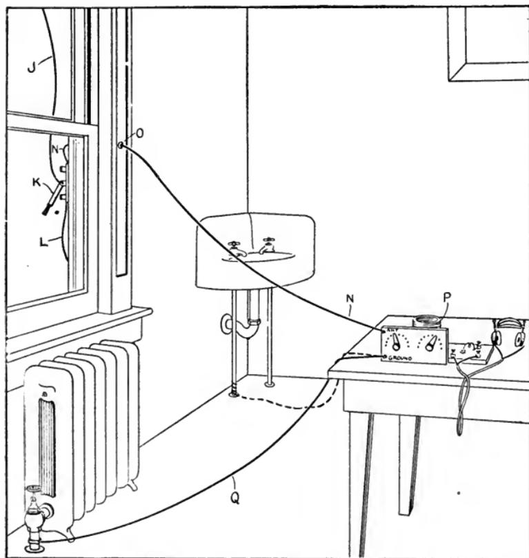
**Fig. 2.**—Arrangement of receiving instrument and connections with antenna and ground.. J—lead-in wire; K—lightning switch; L—ground wire; N—lead to receiving set; O—insulating tube; P—receiving set; Q—ground for receiving set.
