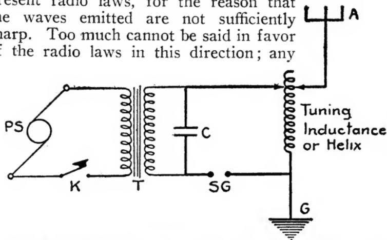
Simple transmitter arrangement for producing fairly sharp waves of the damped variety. PS—power source; K—telegraph key; T—transformer; C—condenser; SG—spark gap; A and G—aerial and ground; and the tuning inductance or helix.
