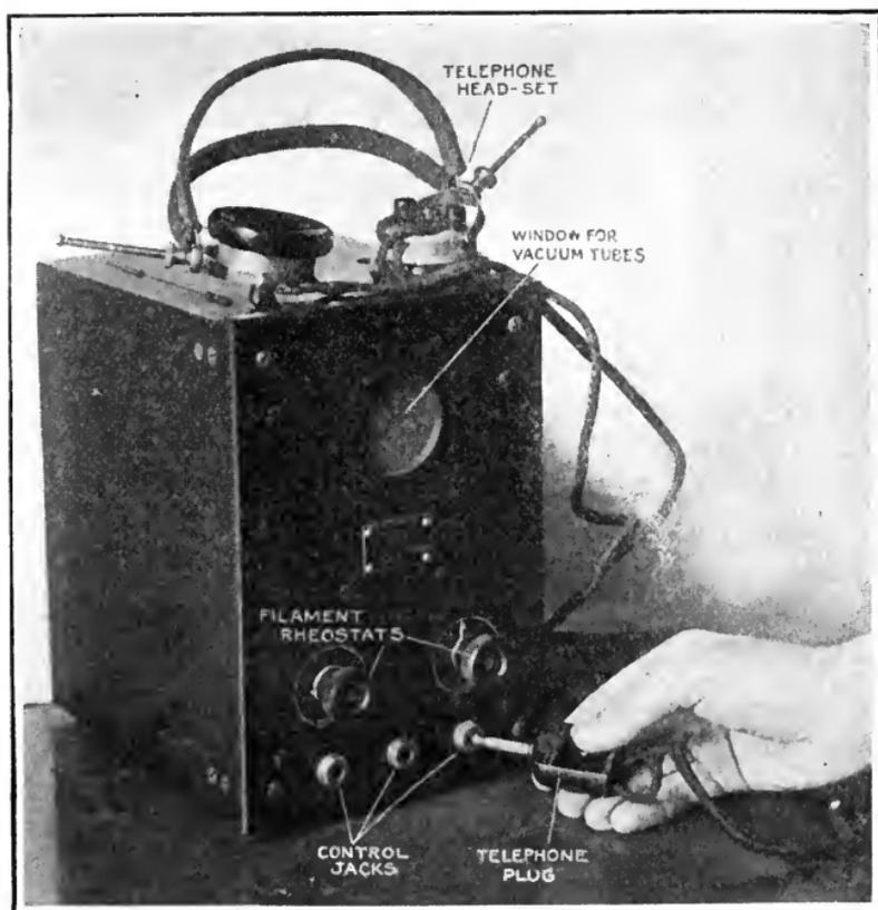
Companion unit to tuner shown on preceding page. This unit is the vacuum tube detector and two-stage amplifier. The two knobs are the rheostat controls for the detector and amplifier tube filaments. The telephone plug may be inserted in one of three holes or jacks, if detector only, one stage or two stages of amplification are desired.
