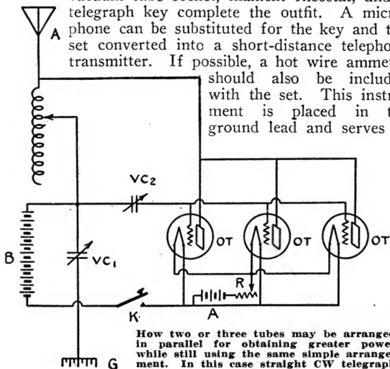
How two or three tubes may be arranged in parallel for obtaining greater power while still using the same simple arrangement. In this case straight CW telegraph is obtained.
