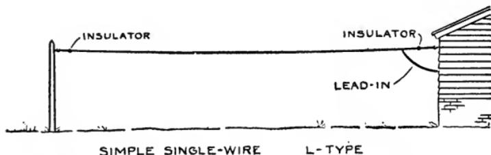
**How the L-type single wire antenna is installed. Such antennae should not be shorter than 60 feet and not longer than 150 feet for best results in the reception of short waves such as are used in amateur and radio-phone work.**
