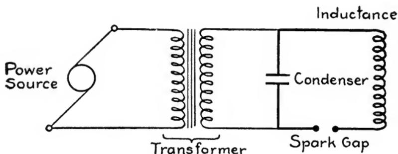
The simplest kind of damped radio wave generator, consisting of a power source, an induction coil or transformer for stepping up the current, a condenser, a spark gap, and an inductance. The charging and discharging of the condenser through the inductance and across the spark gap sets up the oscillations or radio waves.
