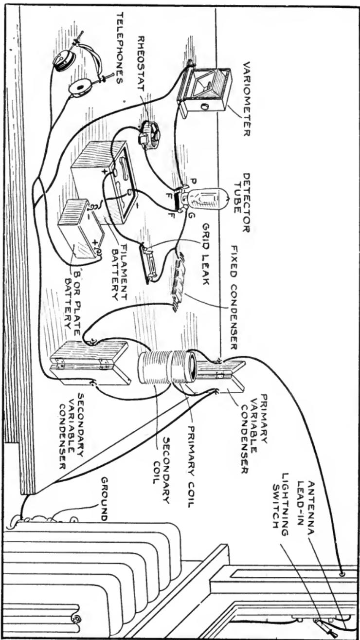
Graphic presentation of the simple regenerative receiving set as it appears when assembled and wired. It is left to the constructor's ingenuity to assemble the units in a neat cabinet for the sake of compactness especially if bought variometer and condensers are employed.
