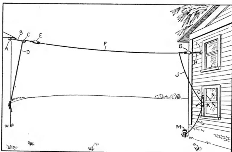
**Fig. 1.**—Construction of antenna for reception purposes. A—screw eye; B—rope; C—pulley; D—rope; E—insulator; F—antenna; G—Insulator; H—rope; I—screw eye; J—lead-in wire; K—lightning switch; L—ground wire; M—ground pipe; N—lead to receiving set; O—insulating tube.
