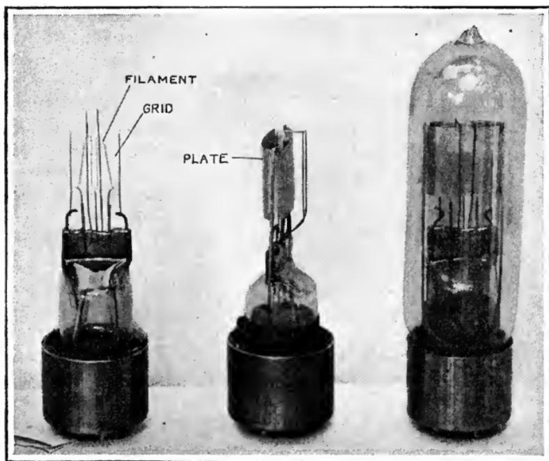
A 50-watt transmitting tube, showing its principal elements. Like the amplifier and detector tubes, it comprises a filament, grid, and plate.
