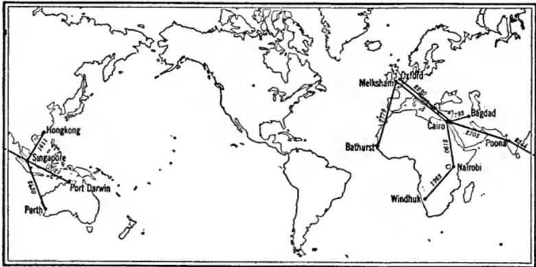
**British Imperial scheme of 1919 for radio communication.** This is a less ambitious but more practical scheme than that of 1913. London is connected with distant points by means of short spans and relays, so that the distances are entirely feasible.
