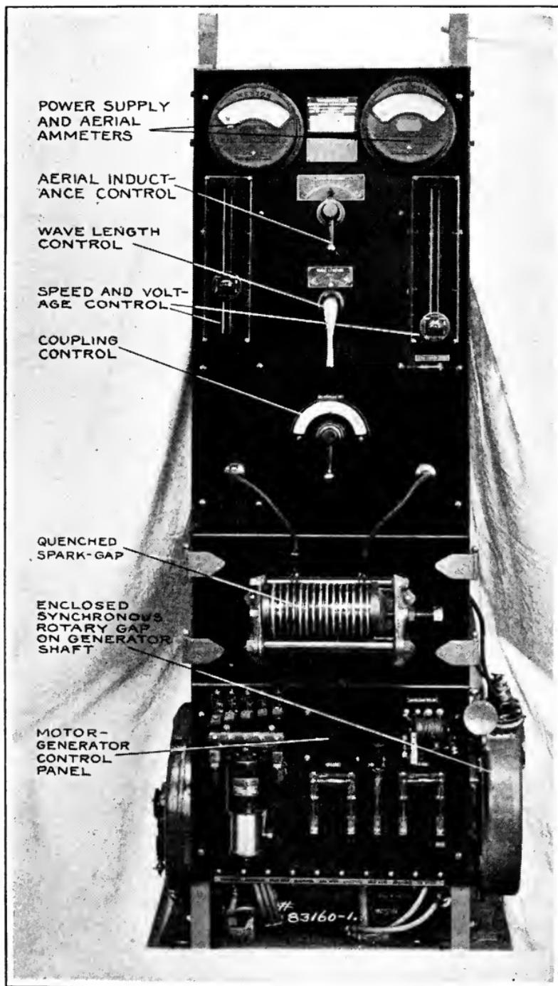
Another type of damped wave transmitter, such as is used on board ship. In this instance there are two methods of obtaining the oscillations or waves. There is the quenched gap mounted on the front of the panel, and the synchronous rotary gap mounted at the right.
