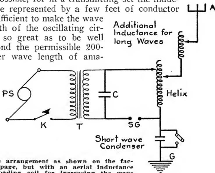
Same arrangement as shown on the facing page, but with an aerial inductance or loading coil for increasing the wave length, and a ground series condenser for reducing the wave length, of the aerial-ground circuit.
