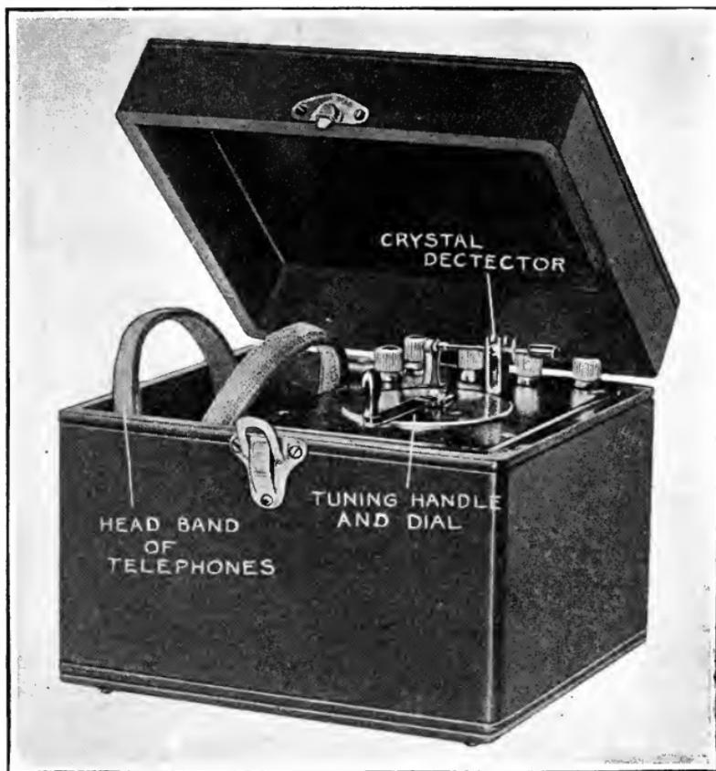
Inexpensive receiving set making use of a variometer tuner and a crystal detector. Such a set is good for a range of 25 miles, perhaps a little more, when receiving radio-phone programs|
