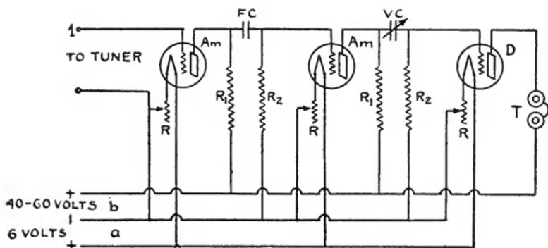
**Resistance type of radio-frequency amplifier.** The set of wires *b* are for the plate battery current, with the polarity indicated, while the *a* set indicates the filament battery current. The wire marked 1 is the grid wire from the tuner. *R* are the filament rheostats; *R*<sub>1</sub>, 2 are resistances; *Am* are amplifier tubes; *D* is the detector tube; *FC*—fixed condenser; *T*—telephones; *VC*—variable condenser.
