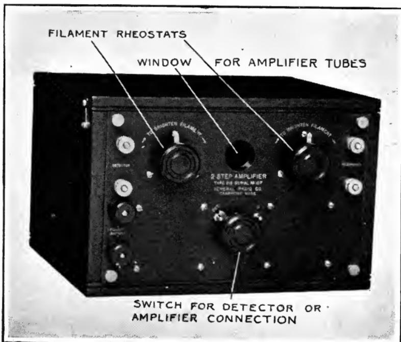
**Two-stage audio frequency amplifier, with filament rheostat handles, switch handle for connecting the detector alone, or one stage or two stages of amplification into the circuit, as well as the input, output, and filament current binding posts mounted on the front panel.**
