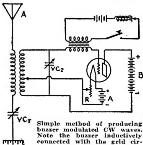
Simple method of producing buzzer modulated CW waves. Note the buzzer inductively connected with the grid circuit. A—aerial; VC1—variable condenser in aerial-ground circuit; VC2—variable condenser in oscillating circuit; R—filament rheostat; A—filament battery; B—plate battery.
