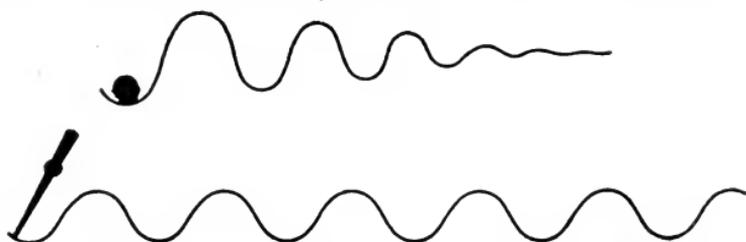
**The difference between damped or discontinuous waves, and undamped or continuous waves in water. Dropping a pebble into water causes damped waves, while using a paddle steadily produces continuous waves.**
