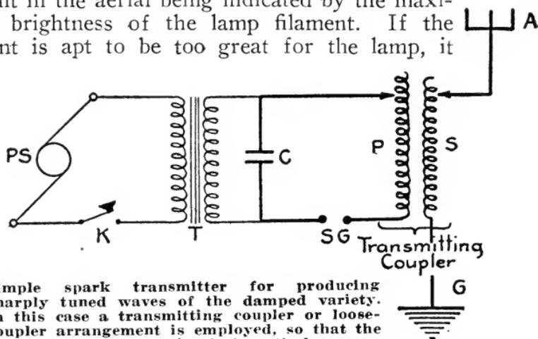
Simple spark transmitter for producing sharply tuned waves of the damped variety. In this case a transmitting coupler or loose-coupler arrangement is employed, so that the oscillating or closed circuit is entirely separated from the open or aerial-ground circuit. The primary P and the secondary S comprise the transmitting coupler.
