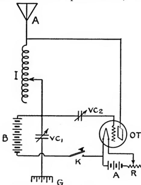
A simple continuous wave telegraph transmitter, making use of a single 5-watt tube. This set transmits straight CW. A—aerial; I—aerial inductance; B—high voltage battery; VC1—variable condenser; G—ground; K—telegraph key; VC2—grid condenser; OT—oscillating tube; A—filament battery; R—filament rheostat.
