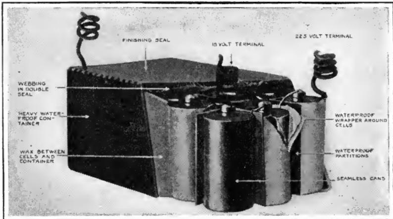
**The construction of a "B" battery, showing the separate cells, the waterproof partitions, the special insulation, the terminals, and the method of sealing the entire battery.**
