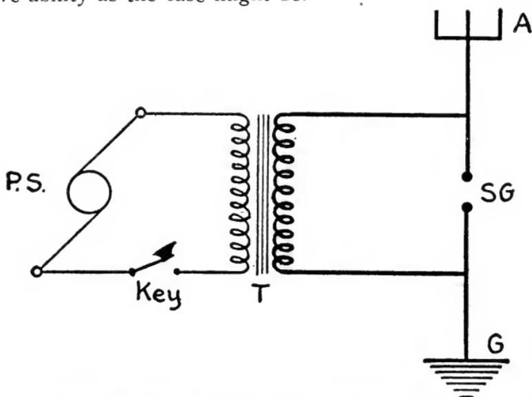
The simplest form of damped radio transmitter, consisting of a power source, telegraph key for making long and short signals of the radio code, a transformer for stepping up the current, a spark gap, and the aerial and the ground. In this arrangement, known as the plain aerial transmitter, the aerial and ground comprise the condenser.
