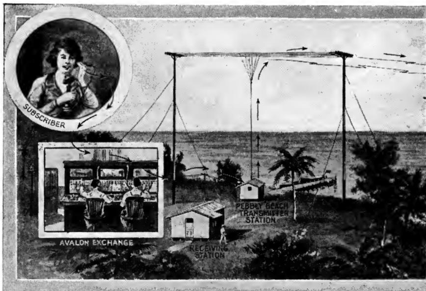
**General scheme of the radio link as used between the California main phone system with that of the Santa Catalina Island and making arrangement, so that two messages can be**
