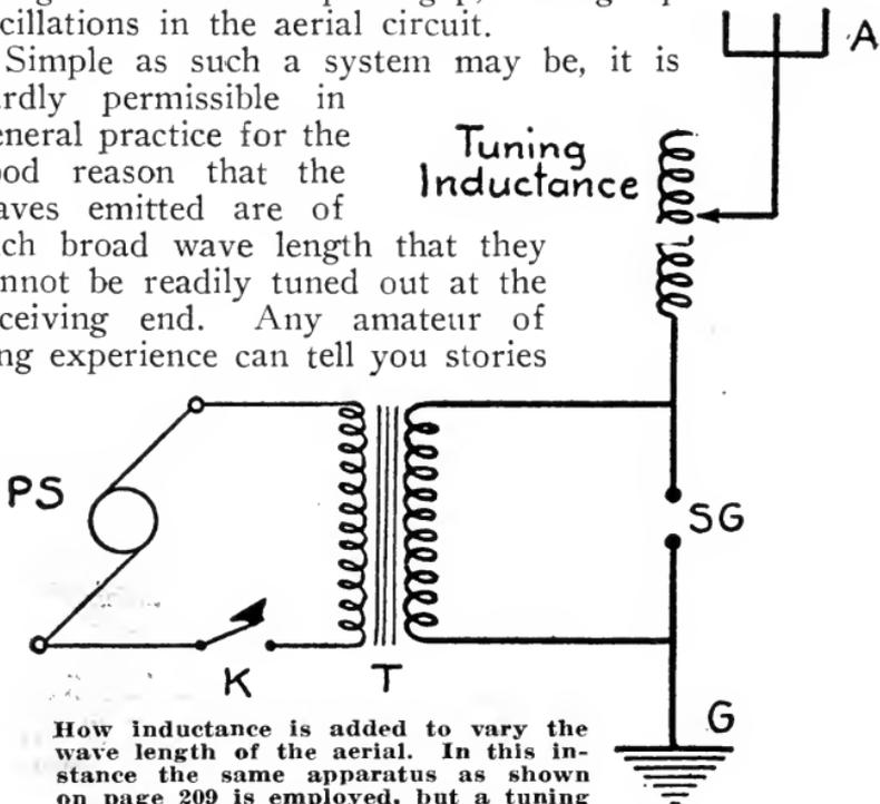
How inductance is added to vary the wave length of the aerial. In this instance the same apparatus as shown on page 209 is employed, but a tuning inductance, known as an aerial inductance or loading coil, is added.
