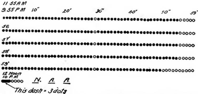
Diagrammatic explanation of the official Navy time signals as sent out by the Arlington station. These signals are re-transmitted by several of the broadcasting stations. Each black dot represents a transmitted dot, while the white dots represent spaces. The time signals start five minutes before 12 o'clock noon and 10 o'clock P. M. and follow the schedule here depicted, terminating with a dash on the hour, followed by a four dot space and the call letters "N A A."
