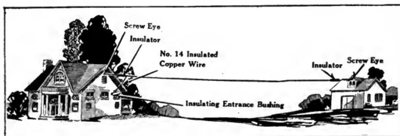
How a receiving antenna may be installed in the country. The single wire may be run from the house to a barn, tree, clothes pole or other support.
