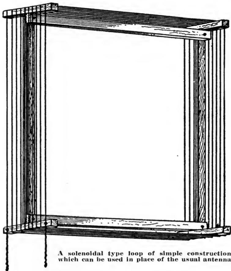
A solenoidal type loop of simple construction, which can be used in place of the usual antenna.
