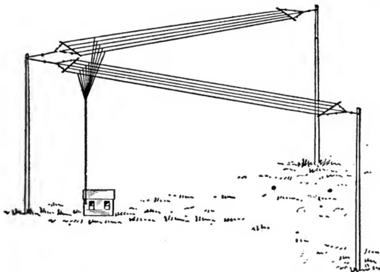
**The V-type aerial—a rare type which should only be employed when a sufficient span cannot be obtained, thus making a double aerial of this kind desirable.**
