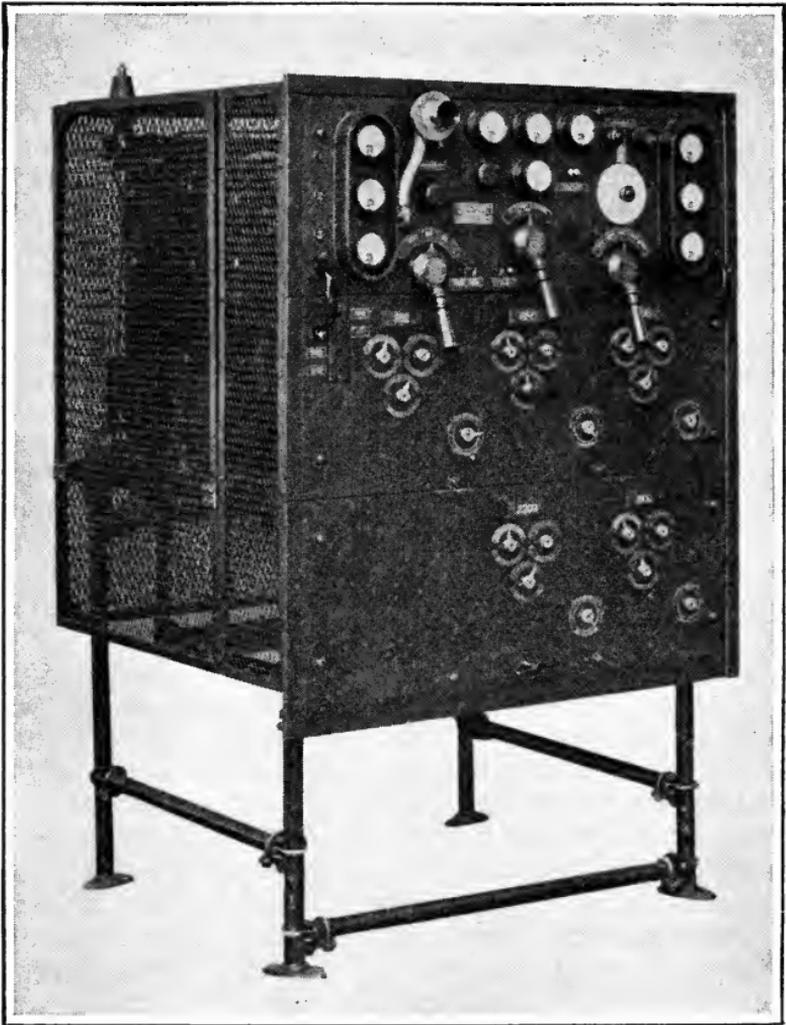
CW telegraph and radio-phone transmitter of the panel type, with the various controls and meters mounted on the front face. Transmitters of this type are being used in several of the radio-phone broadcasting stations.
