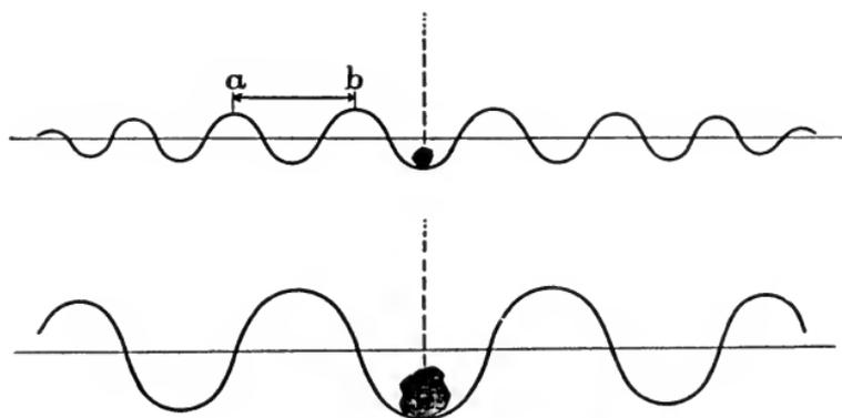
**What happens when a pebble and a large stone are dropped in still water. Note how the pebble causes small waves, and the large stone large waves. Measured from crest to crest, such as  $a-b$ , we obtain the wave length of the waves.**
