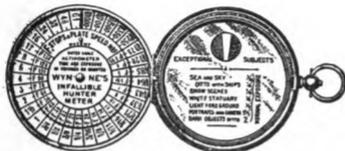
On the right hand side of the open case is the Actinometer with standard tints and sensitive paper. On the left hand side of the case are the two scales for the calculation of the exposures. The top dial is interchangeable so that scales according to either F, U S, or specially divided scales for Autochrome exposures can be instantly substituted for one another.
