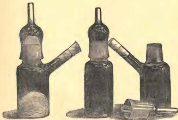
FIG. 3. Flasks in which yeast cultures (i) can be sent through the post, or (ii) in which cultures may be developed or (iii) preserved.
