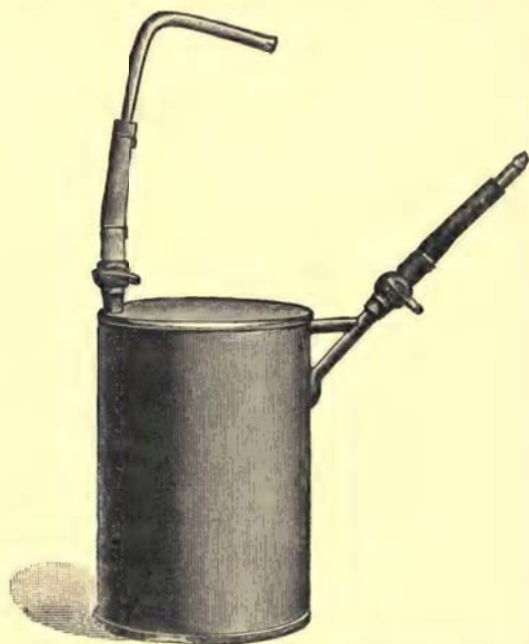
FIG. 10. Travelling can for the despatch of pure cultures of yeast.
