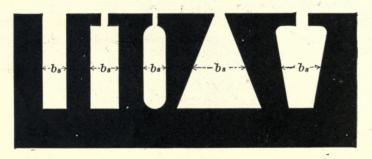
Fig. 49.-Various Types of Slots for Toothed Armatures.
