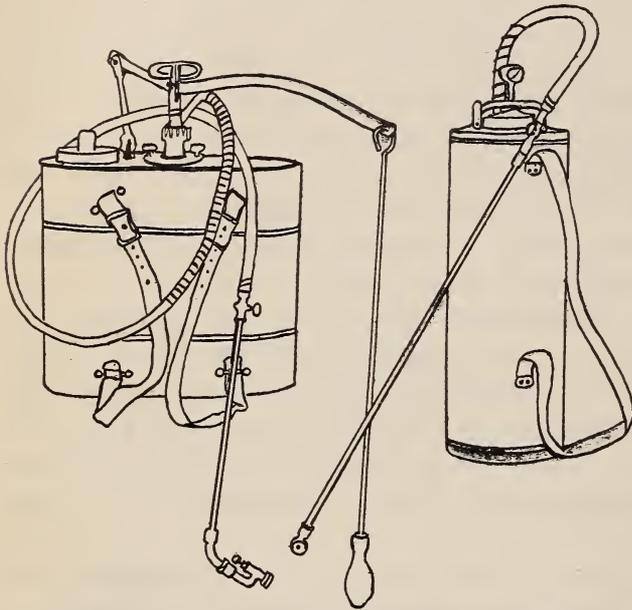
FIG. 3.—Desirable types of hand sprayers, with extension rods permitting thorough underspraying of the foliage.
