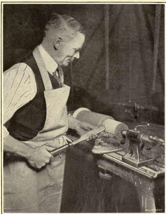
Fig. 11. Method of using Gouge for Rough-turning
