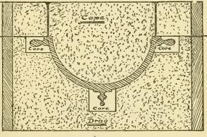
Fig 51 Gross section through flask showing metal & cores
