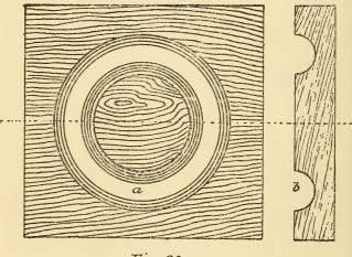
Fig 32 Maner of turning core box for Fig 30
