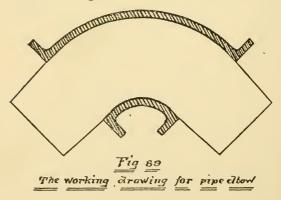
this pattern, take a piece of stuff of proper dimensions and into the face turn a semicircular
