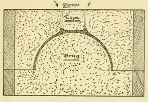
Fig 5 Cross section through mould
