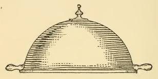
for the handles and finial. Make suitable core boxes for these prints, which core boxes should
