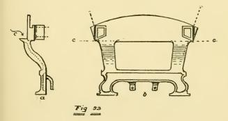
of the casting, the parting is made without any trouble. As an example of a pattern of this kind the aisle end for a car seat has been selected. This pattern was arranged in such a manner as to be divided in the middle, so that the upper portion is cast separate from the leg and used for the wall end of the seat. (See Fig. 53, a and b.) The first step in this case was to make up the follow board (Fig. 54), on which the aisle
