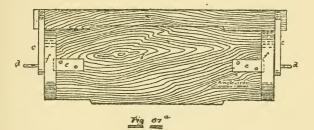
the front of an engine, usually termed "the smoke box door." It was required to cast hinges on this door, together with some other minor projections not necessary to illustrate. The first thing
