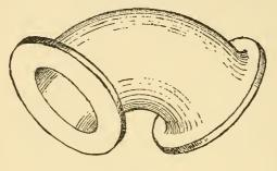
Fig 88 A double flanged steam pipe clbow
