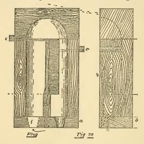
make the vent holes c c c, Fig. 75, which let the steam out into the bell of the whistle.
