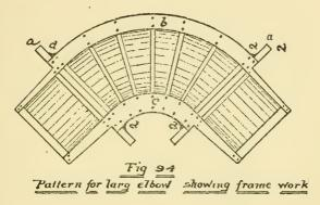
have a problem in construction which should be solved in the following manner: Get out the two circular flanges, *a a*, Fig. 94, which should each be
