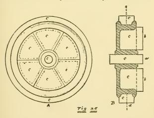
in an inverted position and filled about half full, or within about two inches of the top, and the sand smoothed down solid. The pattern is then turned with the spoke side up and pushed down hard into the sand. It is then taken out to see that the impression is perfect, and a parting is made at i. The pattern is then put back in its place and the parting c-d and e-f is made. The sand is then filled in to g-h and a second parting is made at c-g n-f. Now the drag is put in place
