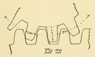
Let it be assumed of a gear wheel of any convenient size, that it is 21 inches in diameter at the pitch line, with any convenient number of teeth, say 44. For all practical purposes an accurate measurement of the circumference of this wheel would be accepted as 66 inches<sup>1</sup> at the pitch line, and the pitch  $66 \div 44 = 1.5$  inches.
