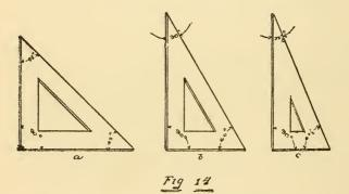
miter joint. The second one contains angles of  $30^{\circ}$ ,  $60^{\circ}$  and  $90^{\circ}$ . This square is employed to lay off the hexagon, or bisect the angles of the hexagon in order to obtain the hexagon miter. The third one contains angles of  $22\frac{1}{2}^{\circ}$ ,  $67\frac{1}{2}^{\circ}$  and  $90^{\circ}$ , and is used to bisect the angles of the octagon, obtaining the octagon miter (see *a b c*, Fig. 14). Some few extra large wooden set
