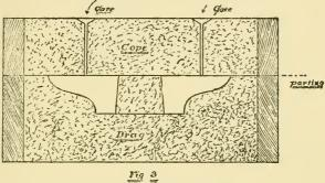
Cross section through finished mouild
