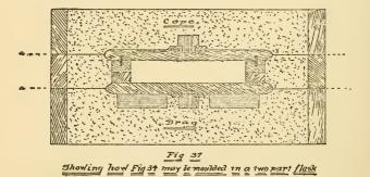
the line c d i e f, is now removed, as is also the pattern from the line a b upwards. The flask should then be put together and turned over,
