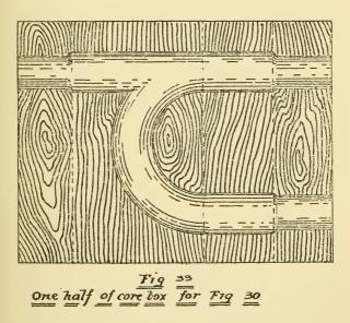
cores marked b b, Fig. 35, B, and a circular core box turned into the face of a plank (see Fig. 39, a and b), which will mould half of the core d shown in Fig. 35, B.
