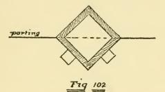
Such a pattern would not draw if divided in the ordinary manner; but the work becomes simple enough when parted as shown in Figs. 102 and 103. The projections for receiving the ends
