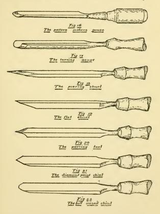
The parting tool, Fig. 20, is used for cutting deep grooves and for cutting off work in the lathe. The diamond point, Fig. 21, and the bull-nosed chisel, Fig. 22, are used for turning both the outside and inside surfaces of hollow patterns, such as the piece shown in cross-section in Fig. 23.
