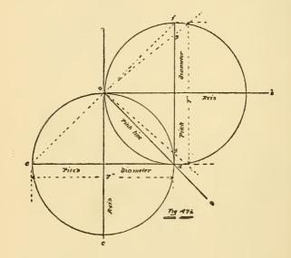
will be 22 inches<sup>\*</sup> and the circular pitch at this point 1 inch. Hence by measuring in 4 of an inch at a right angle from the pitch line a-a, and a-f at the pitch diameter, the profile of a cone is obtained to which the teeth or cogs may be
