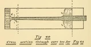
study of Fig. 60. A round core is also required for the center hole. The center stake should be turned up of proper size so that when drawn out or driven down it will leave a print for the center core.
