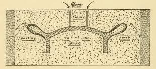
Gross section through fire extinguisher top & mould
