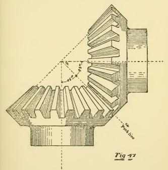
of the pitch from the axis of the wheels. To change the angle of the axis from a right angle would also determine the angle of the pitch line. To more fully illustrate the manner of laying out Fig. 47, see Fig.  $47\frac{1}{2}$ . Here *a b* and *a c* represent the axis on which the gear revolves and a a the pitch line. Assuming, for convenience of calculation, that the pitch diameter d-e and d-f are 7 inches in length and the number of teeth 22, the circumference at the pitch diameter
