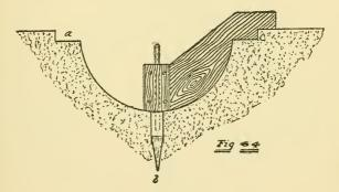
A much more difficult operation is one where the casting is of such a form that it is impossible to lift the cope from the outside. (See Fig. 62.) In this instance a hole is swept into the drag—or foundry floor, as the case may be—having the form of the inside of the casting. (See Fig. 64.) The cope is then placed in position, rammed up and removed. The second sweep is then placed on the stake and the sweeping continued until a
