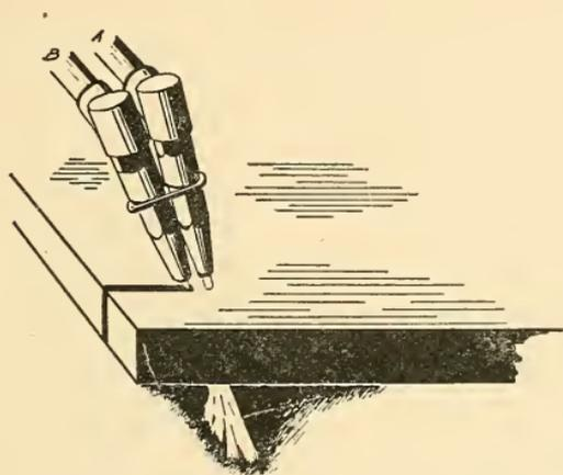
FIG. 84.—Method of Cutting with Two Welding Torches. Torch *A* is Adjusted so that a Neutral Flame will do the Preheating, while a Fork in the Oxygen Line Supplies Oxygen only to Torch *B*, and it does the Cutting.
