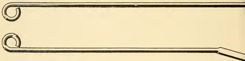
FIG. 77.—“Puddle-sticks” for Welding Aluminum.
