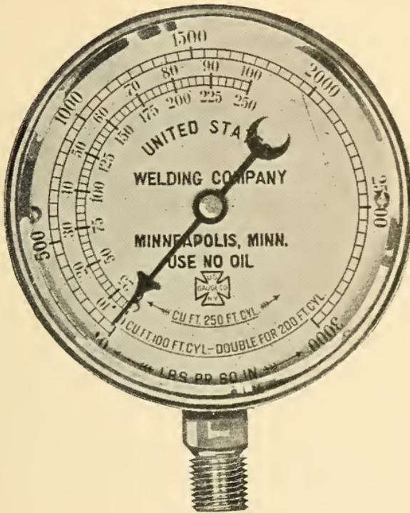
FIG. 35.—A 3000-pound High-pressure Oxygen Gauge.
