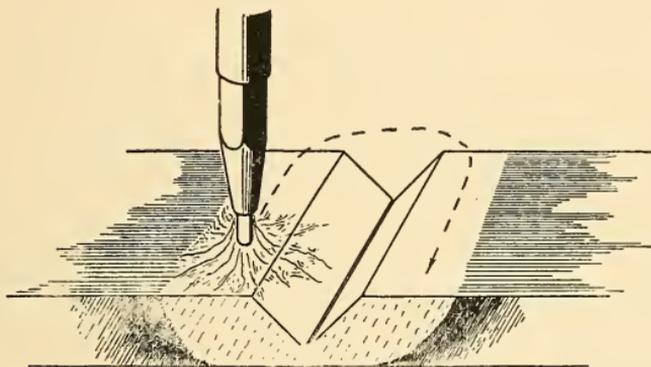
FIG. 57.—Preparing and Heating Steel before Welding.
