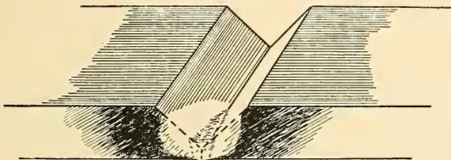
FIG. 45.—Starting a Cast-iron Weld.
