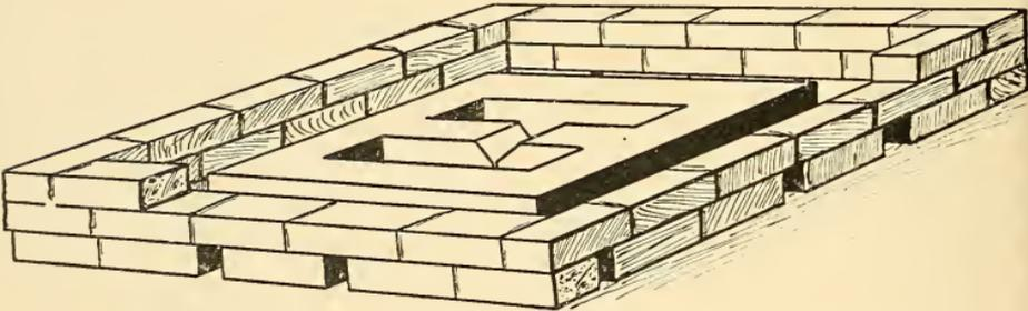
FIG. 39.—Temporary Preheating Oven, Built of Fire Brick.
