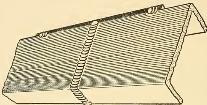
FIG. 64.—A Good Method of Reinforcing a Weld on an Automobile Frame is Here Shown. The Patch as Pictured Here is only "Tacked On." It Should be Welded Securely to the Bottom of the Frame on all Four of its Edges.
