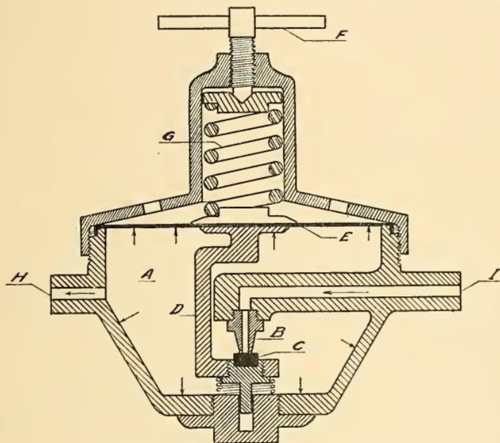
FIG. 16.—Cross-section of Regulator.
