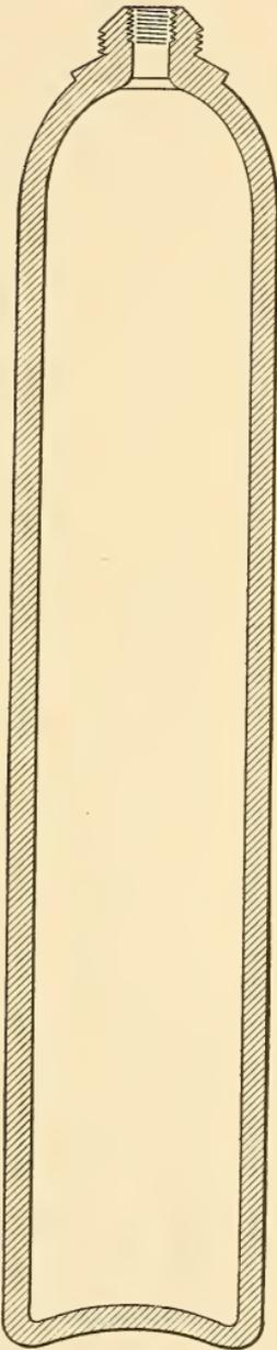
FIG. 17.—Sectional View of Oxygen Cylinder without Valve.
