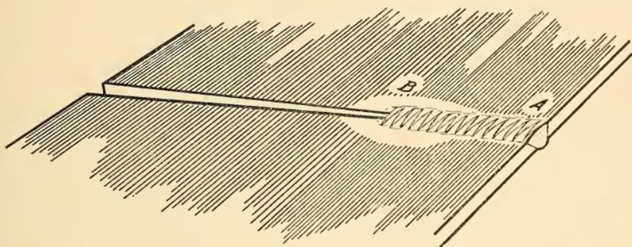
FIG. 63.—This Illustration Shows how the Open Ends of Thin Cast-iron Pieces Spread apart as the Weld Progresses. To Close the Edges together, Jump the Torch Flame from *B* to *A*; as *A* heats up, *B* Cools and the Lever-like Action Closes the Opening.
