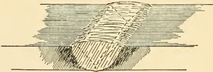
FIG. 46.—Reinforcing a Cast-iron Weld.
