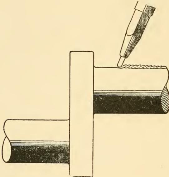
FIG. 65.—Building Up Worn Shafts.
