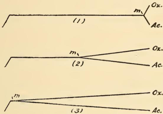
FIG. 15.—Location of Mixing Chambers in Welding Torches.
