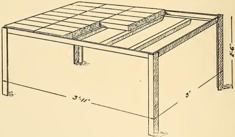
FIG. 29.—A Fire-brick Table for Welding.
