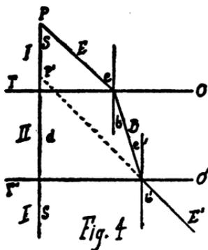
in practice, and which is represented in Fig. 4. The plate with plane parallel faces of the substance II lies imbedded in the medium I. The incident ray  $E$ , which lies in a plane perpendicular to both refracting planes, makes with the first plane the angle of incidence  $e$  and the angle of
