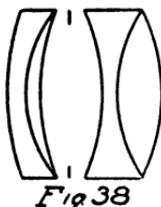
also can be constructed with a normal glass-pair, so that anastigmatic flatness of field can also be attained with two old achromats. This variety, however, does not exist in any commercial lens.
