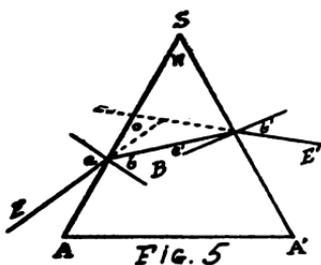
form any given angle with one another. The space which lies between two such planes is called *prismatic*, and a body thus bounded is named a *prism*. We represent the prism diagrammatically by a section in the plane of the
