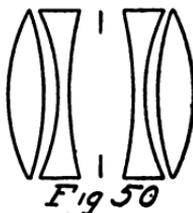
assistance of suitable changes of thickness and distance, and the chromatic correction is effected by a suitable choice of glasses. If we unite two objectives thus calculated (Fig. 50), we obtain a four-lens symmetrical objective, which is corrected in the usual way for,
