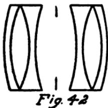
cemented surfaces is reversed, and the bi-convex lens of the heaviest barite crown is placed in the center. This objective was announced by von Höegh as a second form of his double anastigmat; it has been made for many years by Watson
