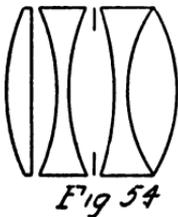
of a cemented collecting surface in the last lens of a triplet. It thus consists of four glasses, of which the first two are separated by an air lens which has the form of a collecting lens and therefore disperses. Therefore, while in the *Unar* both cemented surfaces of the four-lens *Protar* are opened, the *Tessar* has lost only the dispers-
