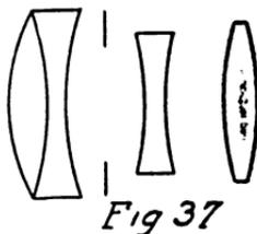
possible to increase the efficiency of the lens within certain limits, but only by sacrificing the possibility of increasing the size of field by stopping down.
