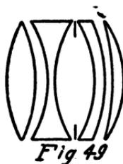
astigmatic, we must again have an opposition of the air lenses in the two halves, one of which must have the form of a collecting, and the other that of a dispersing lens. It may easily be seen that the number of possible elements of construction (radii, thicknesses, and kinds of glass) is considerably increased, and, therefore, we are able to obtain better corrections in such a lens than are possible in the Protars, which consist of cemented lenses.
