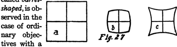
front diaphragm. If, on the other hand,  $m$  increases simultaneously with  $y$ , the image of the square has its sides concave. We observe this *cushion-shaped* distortion when we place the stop behind the lens. These phenomena become especially striking if we move the stop away from the lens, and thus modify the path of the rays.
