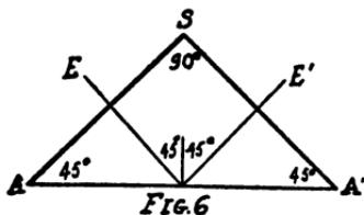
constructed of the most transparent possible crown glass. If a ray  $E$  falls perpendicularly on one face,  $SA$ , of the prism, its two angles before and after total re-
