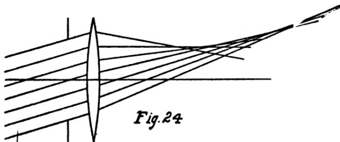
this case there is no kind of symmetry. The ray falling on the upper edge of the objective is most strongly refracted and, in general, corresponding in character to a spherical under-correction, cuts its neighboring ray at a shorter distance than this its next neighbor. We thus obtain instead of an image point, a *caustic curve* which produces a very serious unsharpness on the ground glass.
