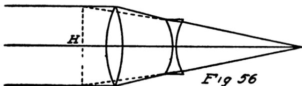
herein lies one of its great advantages compared with ordinary objectives, the distance of the ground glass from the lens is *less* than the equivalent focus of the whole teleobjective. With short cameras pictures can thus be taken on a larger scale than with ordinary lenses of the same focal length. The image of a distant object produced by the teleobjective  $f$  is, compared
