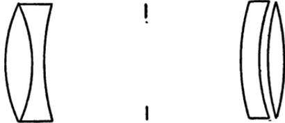
contains two separated lenses, flint before crown. In order to obtain a better spherical correction, the objective is now constructed according to the proposal of J. H. Dallmeyer in 1866, with the crown before the flint in the rear combination, but still with the separated lenses. It is completely unsymmetrical in both cases. The very long con-
