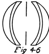
curvatures, as in the anastigmatic meniscus, are very great, so that the spherical aberration is very large, because of the absence of a dispersing cemented surface. This wide-angle lens, therefore, can only be used with a small stop, but then covers a field of  $110^\circ$ , which is surpassed only by the Hypergon. The chromatic correction of the Pantoscope is good, and thus a difference of chemical focus is avoided.
