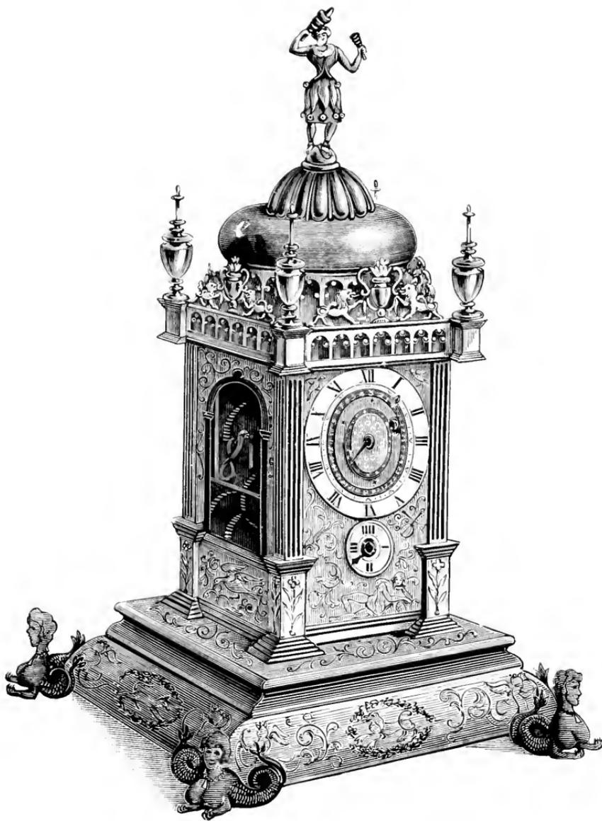
FIG. 102.—Clock with early balance spring.
