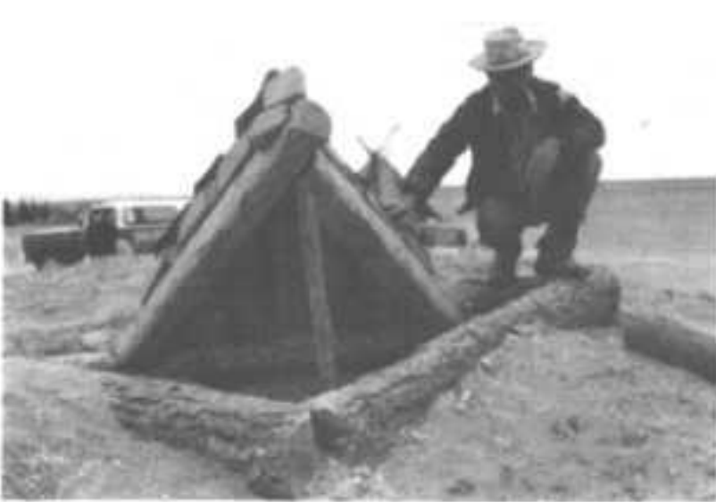
Fig. D.16. Blast-tested triangular blast door made of hand-hewn pine poles, notched and nailed together. This door closed on a triangular pole base that is concealed in this photo by two of the three blast-protector logs that also withstood 53-psi blast effects.
