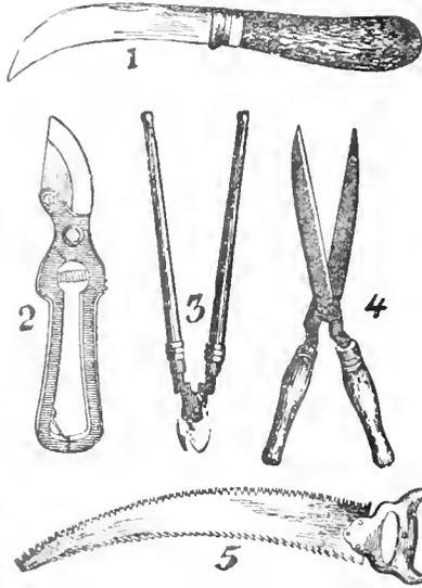
1. Hawkbill knife for small trees and larger branches. 2. Hand pruner shears for still larger branches. 3. Lopping shears for pruning hedges. 4. Shears for pruning hedges. 5. A very desirable form of pruning saw.
