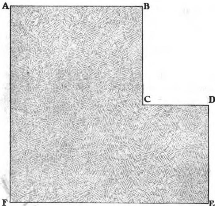
This picture is the plan of a lot drawn to the scale, 1 inch to 12 feet. This means that an inch on the drawing stands for a distance of 12 feet in the lot. Using the scale named, measure and give the following distances in the lot.
