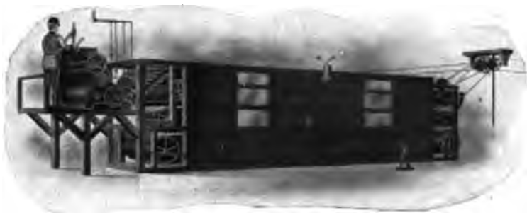
FIG. 164.—Automatic Continuous Crusher and Dryer.
