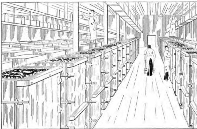
FIG. 80.—Frame-room, Frames Filled by Trough System.
