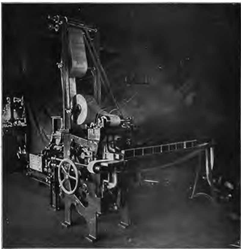
FIG. 118.—Automatic Soap-wrapping Machine.
