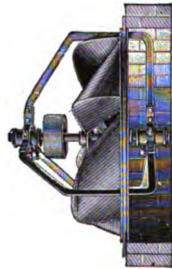
FIG. 98.—Disc Fan Set in the Side Wall.
