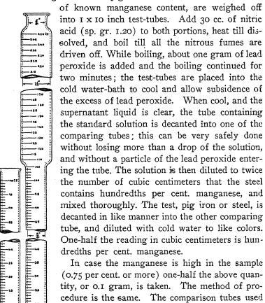
(0.75 per cent. or more) one-half the above quantity, or 0.1 gram, is taken. The method of procedure is the same. The comparison tubes used are represented in the accompanying drawing. The color tubes used show plainly their advantages over the ordinary tubes.
