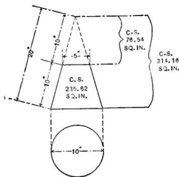
Fig. 30. — Convex Surface of Frustum of Right Cone.
