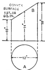
Fig. 25.—Convex Surface of Frustum of Cylinder.
