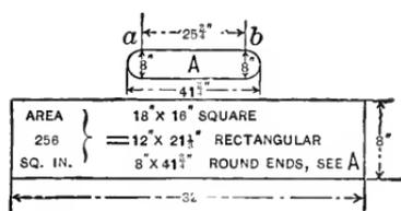
Fig. 43.—Pipes Equal to Rectangular Pipe.
