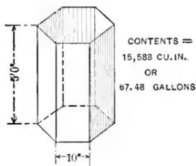
Fig. 33.—Contents of Hexagonal Prism.
