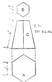
Fig. 31. — Convex Surface of Frustum of Right Pyramid.
