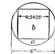
Fig. 6.—Finding Length of Side of a Square to Be Inclosed by a Given Circle.
