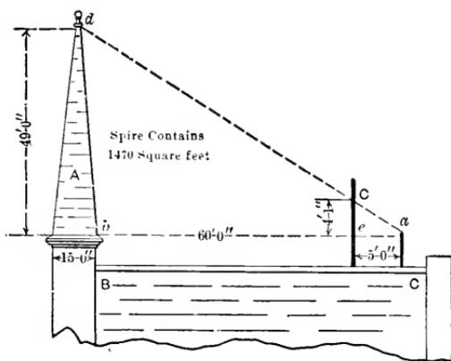
Fig. 62.—Finding Height of Inaccessible Point.
