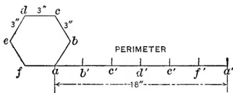
Fig. 3.—Finding Length of Perimeter of a Hexagon.
