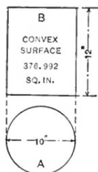
Fig. 24.—Convex Surface of Cylinder.
