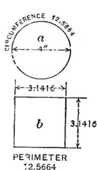
Figs. 4 and 5.—Finding Square and Circular Sections of Pipe of Given Dimensions.
