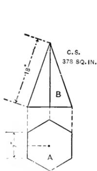
Fig. 29. — Convex Surface of Right Pyramid.
