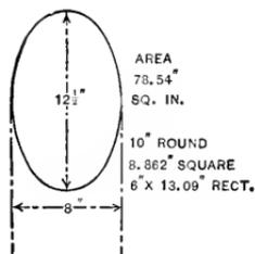
Fig. 50.—Elliptical Pipe.
