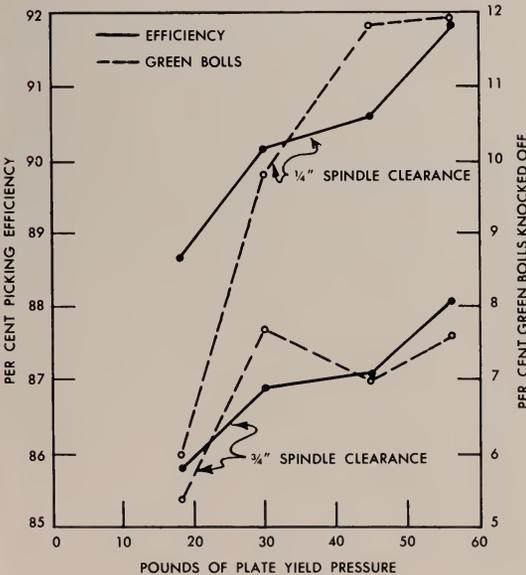
Fig. 11. Graph showing the effect of different pressure-plate settings on picking efficiency and green-boll loss.
