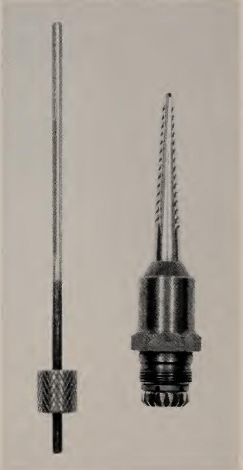
Fig. 9. Cotton picker spindles. *Left*: smooth rod; *right*: barbed cone.
