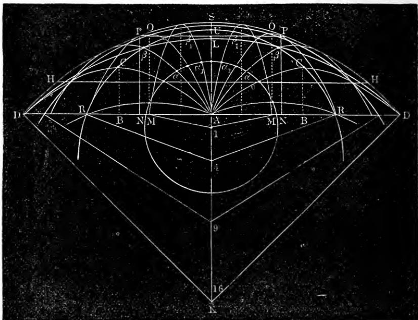
A bunch of jets rising from  $A$  in all directions would be enveloped by the paraboloid generated by the revolution of the envelope  $D P S P D$  about  $AS$ . If  $t$  is the time in which a body rising in a parabola describes the arc  $AO$ , Fig. 76, the co-ordinates of which are  $AM = x$  and  $MO = y$ , we have
