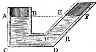
Hence it follows that the water in the communicating tubes  $A B C$  and  $D E F$ , Fig. 594, will stand at the same height, when in equilibrium, or that the surfaces  $A B$  and  $E F$  will be in the same horizontal plane. In order to preserve the equilibrium it is necessary that the layer of water  $H R$  shall be pressed downwards by the column of water  $E R$  above it as much as it is pressed upwards by the mass of water below it. Since in both cases the
