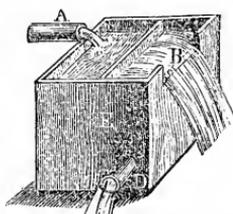
regulated by means of a lever and a float  $K$ , so that the same quantity of water is discharged through  $B$  as through  $F$ .
