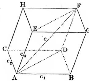
In case the velocities do not lie in the same plane, the resultant can also be found by repeated application of the parallelogram of velocities. The resultant  $AF = c$  (Fig. 68) of three velocities  $AB = c_1, AC = c_2$  and  $AE = c_3$ , not in the same plane, is the diagonal of a parallelepipedon whose sides are equal
