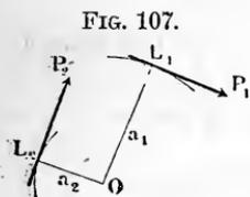
In adding the moments, we must pay attention to the positive and negative signs. If the forces  $P_1$  and  $P_2$  act in the same direction around  $O$ , as in Fig. 107, if, e.g., the direction of the forces coincide with the direction of motion of the hands of a watch, they and their moments are said to have the same sign, and if one of them is taken as positive, the other must also be considered as positive. If, on the contrary, the two forces, as in Fig. 108, act in
