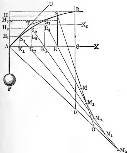
We have already found (§ 217) the deflection for a prismatic body  $A S B$ , Fig. 385, fixed at one end  $B$  and loaded at the other  $A$ , to be
