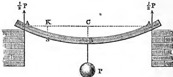
bent exactly in the same way as in the case just treated, but in this case we must substitute for the force acting at  $A$ ,  $\frac{1}{2} P$
