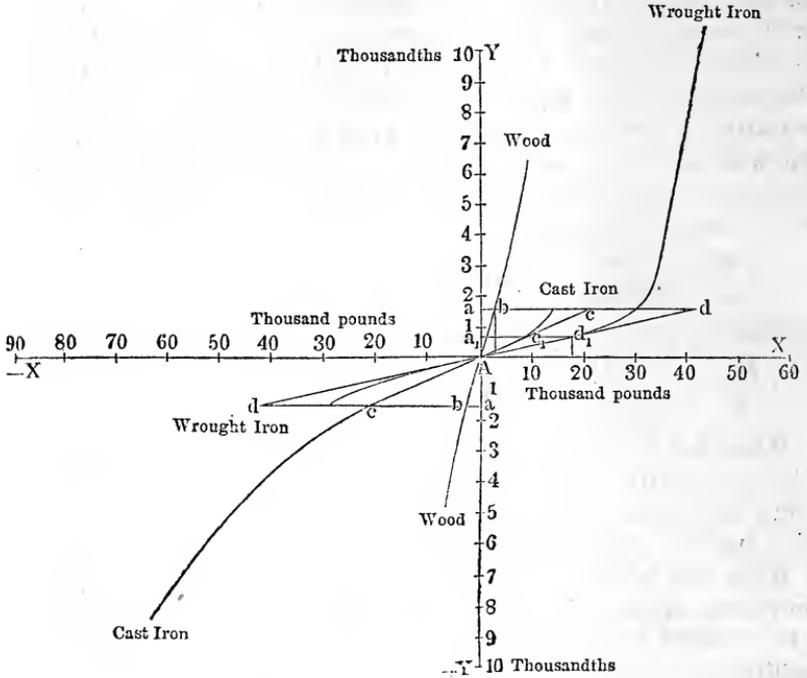
The modulus of resilience  $A = \frac{1}{2} \sigma T$  for the limit of elasticity is expressed by the triangles  $A a b$ ,  $A a_1 c_1$  and  $A a_1 d_1$ , the bases of which are the small ratios of extension  $\sigma = A a = \frac{1}{600}$  and  $\sigma = A a_1 = \frac{1}{1500}$  (approximately).
