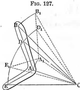
$A_1 C E_1$  and  $A C E$  are equal to each other, and the same thing can be proved for every other point rigidly connected with  $A B$ . We can, therefore, consider any small motion of a surface or of a solid body rigidly connected with  $A B$  as a small rotation about a centre, which is determined by the point of intersection  $C$  of the perpendiculars to the spaces  $A A_1$  and  $B B_1$ , described by two points of the body.
