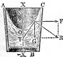
the surface of the revolving water forms a hollow  $A O C$ , whose cross-section through the axis is a parabola. If  $\omega$  is the angular velocity of the vessel and of the water in it,  $G$  the weight of an element  $E$  of the water, and  $y$  its distance  $M E$  from the vertical axis, we have the centrifugal force of this element
