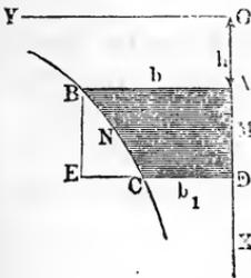
edge be  $A B = b$ , that of the lower edge,  $C D = b_1$ , and the height of the orifice,  $A D = a$ . Horizontal lines at the distance  $\frac{a}{n}$  from each other will divide this orifice into strips of equal height, and the discharge  $\frac{Q}{n}$  through each of them should be the same. For the upper strip, whose width is  $b$  and for which the head is  $h$ , we have
