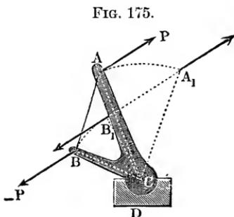
a body  $ACB$ , Fig. 175, is rigidly fastened at  $C$ , and if the direction of the force forms the angle  $BAP = \alpha$  with the line  $AB$  passing through the two points of application, a rotation  $ACA_1 = \beta = 180^\circ - \alpha$  is necessary to annul the moment of the couple ( $P, -P$ ); the same is also true of a body rigidly fastened in an axis and acted upon by a couple, whose plane is perpendicular to this axis.
