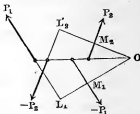
No finite force acting at a finite distance can balance a couple, but two such couples can balance each other. Let  $P_1$  and  $-P_1$  and  $-P_2$  and  $P_2$ , Fig. 115, be two such couples, and  $O L_1 = a_1$ ,  $O M_1 = O L_1 - L_1 M_1 = a_1 - b_1$ ,  $O L_2 = a_2$  and  $O M_2 = O L_2 - L_2 M_2 = a_2 - b_2$  their arms measured from a certain point  $O$ , then, when equilibrium exists, we have
