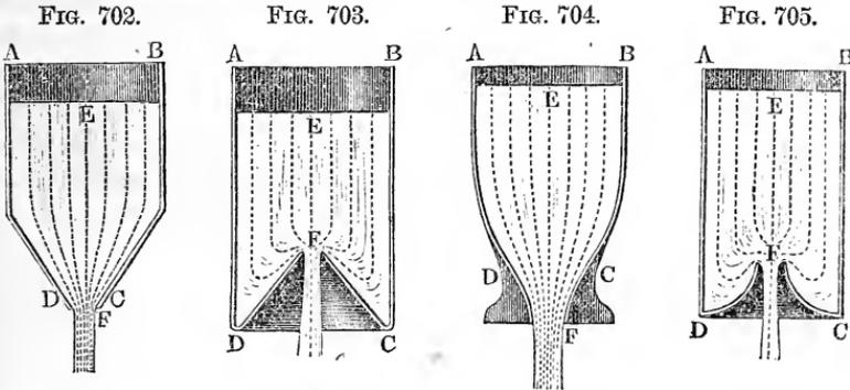
order to reach the orifice. Both cases are represented in Figures 704 and 705. In the first case the coefficient of efflux is nearly 1, viz. : 0,96 to 0,98, and in the second case, according to the measurements of Borda, Bidone and of the author, its mean value is = 0,53.
