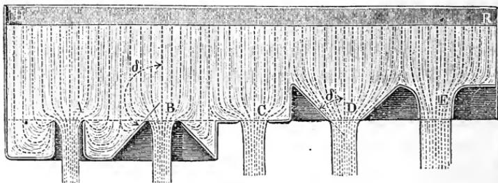
with that of the molecules of water which flow in from the side, is a right angle  $\left(\frac{\pi}{2}\right)$ ; when the orifice *A* is formed by the thin edge of a tube, this angle  $\delta$  is two right angles ( $\pi$ ); when we have a conical divergent mouth-piece *B*,  $\delta$  is between  $\frac{1}{2} \pi$  and  $\pi$ ; when the discharge takes place through a conical convergent
