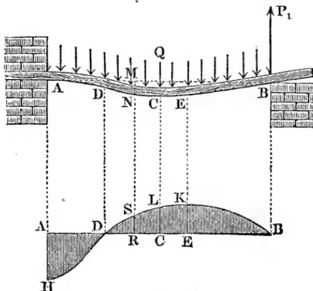
manner as the last, is uniformly loaded, as we have previously generally supposed, with a certain weight  $q$  upon the running foot of the girder, we can determine the reaction  $P_1$  at the support  $B$  in the following manner. If the length of the beam is  $l$ , the entire load is  $Q = l q$  and the moment of the force in reference to a point  $M$ , at a distance  $B M = x$  from the point of support  $B$ , is
