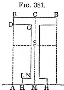
Let the entire height of the beam be  $AB = h$ , the width of the upper flange be  $BC = b$ , the height of the hollow on the side be
