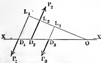
In every system of parallel forces we can substitute for the arms the distances  $OD_1, OD_2$ , etc., cut off from any oblique line by the directions of the forces. Since the intensity and direction of the resultant of a system of forces with different points of application is the same as that
