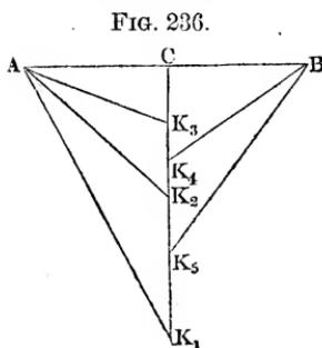
the hypotenuse  $AK_1$  will give the total tension  $S_1$  of the first portion of the rope, and the angle  $CAK_1$  the inclination of the same to the horizon. If, now, we lay off upon  $CK_1$  the weights  $G_1, G_2, G_3$ , etc., as the divisions  $K_1 K_2, K_2 K_3$ , etc., and draw the transverse lines  $AK_2, AK_3$ ,
