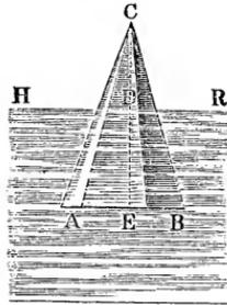
For a pyramid,  $A B C$ , Fig. 623, floating with its base under water, we obtain, on the contrary, the distance  $CD = y_1$  from the apex to the surface of the water by putting
