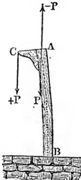
$P$  in the direction of the axis, and a couple  $(P, -P)$ , whose lever arm  $c$  is the distance  $CA$  of the point of application of the force  $P$  from the axis of the body, and whose moment is therefore  $= P c$ . The force  $AP = P$  in the line of the axis produces in all the fibres the constant strain  $S_1 = \frac{P}{F}$ , in which  $F$  denotes the cross-section of the body; the
