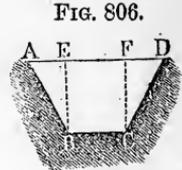
the bottom =  $b$ , the depth  $BE = a$  and the slope  $\frac{AE}{BE} = v$ , we have the wetted perimeter of the profile  $p =$
