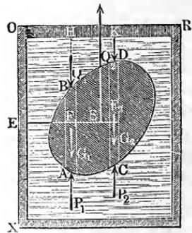
In order to find the *vertical pressure* of the water upon a body  $ABD$ , Fig. 617, immersed in it, let us imagine it to be decomposed
