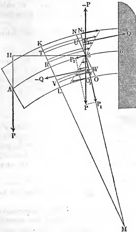
But this sum can only be  $= 0$ , when the point  $S$  of the axis coincides with the centre of gravity of the surface  $F = F_1 + F_2 + F_3 + \dots$ ; consequently the neutral axis of a bent body passes through the centre of gravity  $S$  of its cross-section  $F$ . The moment of the couple ( $Q, -Q$ ),
