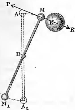
torsion-rod to vibrate, we can observe the period of the vibrations, and from it we can calculate the force of torsion. According to the foregoing paragraph, the period of a simple vibration is
