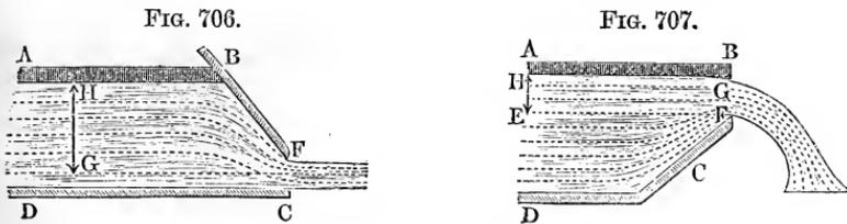
slope of one-half to one. For the overfall, represented in Fig. 707, where, as in Poncelet's sluice, contraction takes place upon one side only, the author found  $\mu = 0,70$  or  $\mu_1 = \frac{2}{3} \mu = 0,467$  for an inclination of  $45^\circ$ , and  $\mu = 0,67$  or  $\mu_1 = 0,447$  for an inclination of  $63\frac{1}{2}$  degrees.
