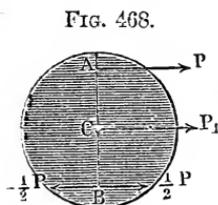
$\overline{AP} = P$  produces the same effect upon the rotation of the body about this axis  $C$  as a couple  $(\frac{1}{2} P, -\frac{1}{2} P)$  with the arm  $2 CA = 2 CB = 2a$ , or with the moment  $\frac{1}{2} P \cdot 2a = Pa$ ; for the remaining central force  $\overline{CP}_1 = P_1 = P$  is counteracted by the bearings of the axis (compare § 130).
