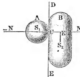
is central; for their centres of gravity  $S_1$  and  $S_2$  lie in the normal  $N\bar{N}$  to the tangent plane. In the case represented in Fig. 551 the impact of *A* is central and that of *B* eccentric; for  $S_1$  lies in and  $S_2$  without the normal line or *line of impact*  $N\bar{N}$ .
