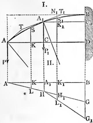
The inclination at  $S$  of this portion of the girder, due to the flexure produced by the moment  $(P + P_1) x_1$ , is measured by the arc
