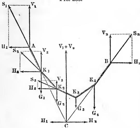
rope and from the angle of inclination  $S_1 A H_1 = a_1$ , we obtain the vertical tension  $V_1 = S_1 \sin a_1$  and the horizontal tension  $H_1 = S_1 \cos a_1$ .
