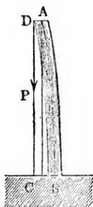
and that the deflection  $BC = a$  of the pillar is small, compared with  $c$ , we can consider the elastic curve formed by the axis of the pillar to be a circle, whose radius is  $r = \frac{l^2}{2a}$ . But now
