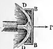
project beyond the surface struck by the water, the water will be deviated from its course at an obtuse angle as in the case of concave surfaces, and the impulse is greater than when the surface is plane. The action of this impact depends principally upon the height of the border and upon the ratio of the cross-section of the stream to that of the enclosed surface. In an experiment, where the stream was
