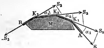
the foregoing decomposition of the force is repeated, so that in the knot  $K_1$  the tension  $S$  is changed into  $S_1 = S \cos. a_1$ , and in the knot  $K_2$  the tension  $S_1$  into  $S_2 = S_1 \cos. a_2 = S \cos. a_1 \cos. a_2$ , and in the knot  $K_3$  the tension  $S_2$  into
