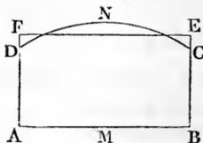
of which above each point of the base is equal to the force corresponding to that point of the path. If we transform the figure  $A B C N D$  in a rectangle  $A B E F$  with the same base and the same area, its altitude  $A F = B E$  gives the mean value of the force.
