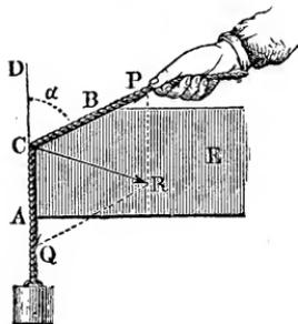
If a perfectly flexible cord stretched by a force  $Q$  is laid over the edge  $C$  of a rigid body  $ABE$ , Fig. 292, and is thus compelled to deviate from its original direction an angle  $DCB = \alpha^\circ$ , a pressure  $R$  is produced at this edge, which gives rise to a friction  $F$ , in consequence of which a force  $P$ , which is either greater or less than  $Q$ , is necessary to produce unstable equilibrium. The pressure is (§ 77)
