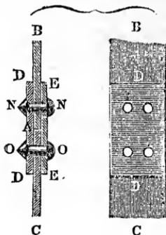
are two modes in which bodies may be fastened together in this way; either the plates  $A B$  and  $C D$  to be joined together are laid upon one another, as in Fig. 330, and then fastened together by the bolts or rivets  $N N$  and  $O O$ , or, as is represented in Fig. 331, the plates are butted together and covered with splicing pieces  $D D$  and  $E E$ , and they are then fastened together by means of the rivets  $N N$  and  $O O$ ,
