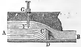
at the sluice gate, it is advisable to attach to the guides two brass scales *B C* and *D E*, Fig. 815, with the pointers *F* and *G* by means of which we are able to read off with more certainty the height of the orifice. It is always better, when measuring water, to employ a new sluice gate and new guides which are properly beveled outwards.
