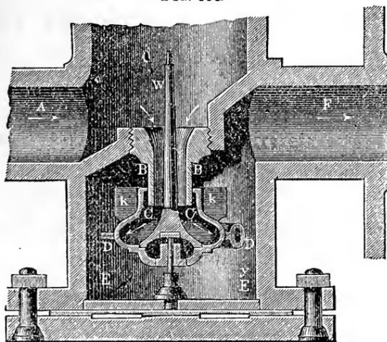
through the pipe  $B B$  into the wheel  $C C$  and is carried by the revolving tube  $D D$  into the case  $E E$ , from which it is carried off by the pipe  $F$ . The shaft  $W$  of the wheel passes upwards through a stuffing-box and sets a train of wheel-work in motion by means of an endless screw fastened to its end. The wings  $k, k$  upon the wheel assist in regulating its motion of rotation by the resistance which they experience in moving in the water.
