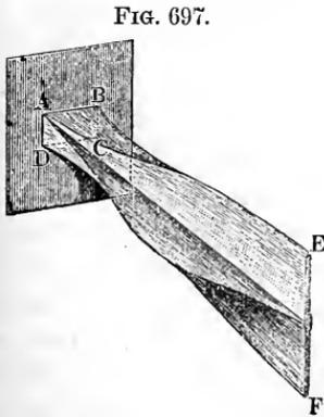
Bidone observed the discharge from various kinds of orifices; Poncelet and Lesbros have made the only accurate measurements of the stream issuing from square orifices (see the *Allgemeine Maschinenencyklopädie*, article "Ausfluss"). The last measurements have led to a small coefficient of contraction 0,563.
