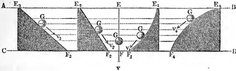
of the heights due to the velocities is always equal to the vertical height of descent. Bodies, which begin to describe the paths  $EF, E_1F_1, E_2F_2$ , etc., with equal velocities ( $c$ ), arrive at the end of these paths with the same velocity, although they require different times to acquire it.
