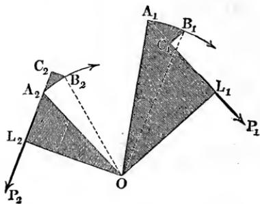
turn a very small distance about a point  $O$ , the principle of virtual velocities announced in § 83 and § 98 is applicable here also, as can be demonstrated in the following manner. According to § 89 the moment of the resultant  $P \cdot \overline{OL}$  =  $P a$  is equal to the sum of the moments of the components, or
