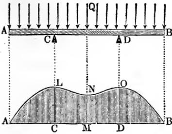
The moment of flexure is a maximum or minimum for  $x = \frac{l}{2}$  and is
