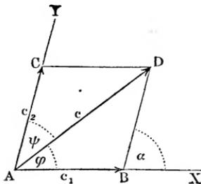
We can also determine, when one component ( $c_1$ ) and its angle of direction ( $\phi$ ) are given, the magnitude and direction of the other. Finally, if the three velocities  $c$ ,  $c_1$  and  $c_2$  are given, we can determine their angles of direction by the same method that we employ to find the angles of a triangle, when three sides are given.
