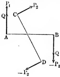
the two couples  $(P_1, -P_1)$  and  $(P_2, -P_2)$ , Fig. 117, are to be combined, we can replace the one  $(P_2, -P_2)$  by another which has the same arm  $AB = b_1$ , as the former couple  $(P_1, -P_1)$ , and can then add the forces thus obtained to the others, and thus obtain a single couple. If  $b_2$  is the arm  $CD$  of the one couple and  $(Q, -Q)$  the reduced couple, we have  $Q b_1 = P_2 b_2$ , and consequently  $Q = \frac{P_2 b_2}{b_1}$ , hence one component of the
