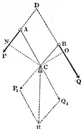
pressure  $R$  on the fulcrum is the diagonal  $R$  of the parallelogram  $CP_1RQ_1$ , constructed with the force  $P$ , the load  $Q$  and with the angle  $P_1CQ_1 = PDQ = a$  formed by their directions with each other.
