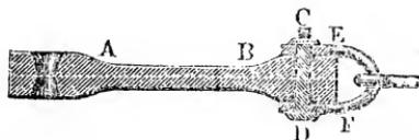
*experimenting upon rupture by extension* we employ bodies with large heads *A* and *B*, Fig. 320, through which holes are bored exactly in the axis. In the middle of each hole a circular
