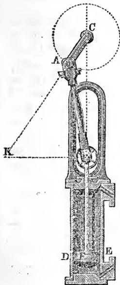
stant, while that of the connecting rod  $AB$  is variable; for its position is determined by the intersection  $M$  of the perpendicular  $BK$  to direction  $CB$  of the axis of the piston-rod and of the prolongation of the crank  $CA$  (see § 101).
