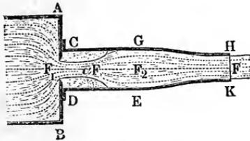
cross-section,  $v$  the velocity and  $p$  the pressure of the water at the outlet  $HK$ ,  $F_1$  the cross-section of the inlet,  $a F_1$  that of the contracted stream of water,  $v_1$  the velocity and  $p_1$  the pressure of the water in the latter; in like manner let  $F_2$  be the cross-section of the tube, where the stream of water again touches the wall,  $v_2$  the velocity and  $p_2$  the pressure of the water at that point. Then we have
