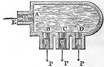
If the axes of the pipes  $B F, C G$ , etc., Fig. 576, are parallel to each other, the forces acting on the pistons can be combined so as to give a single resultant; if  $n$  is the number of the equally large pistons, the total pressure upon them will be
