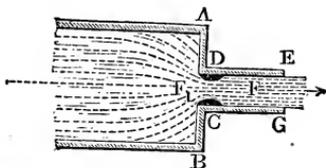
If the diaphragm is absent, we have a common short pipe, Fig. 743, and then  $F = F_1$  and
