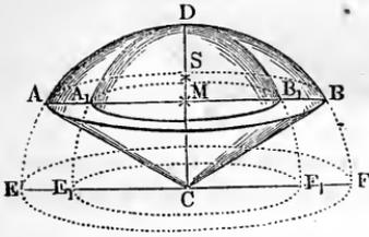
the moment of the segment equal to that of the spherical sector  $ADB C$  less that of the cone  $ABC$ . Denoting again the radius  $CD$  of the sphere by  $r$  and the altitude  $DM$  by  $h$ , we have the moment of the sector
