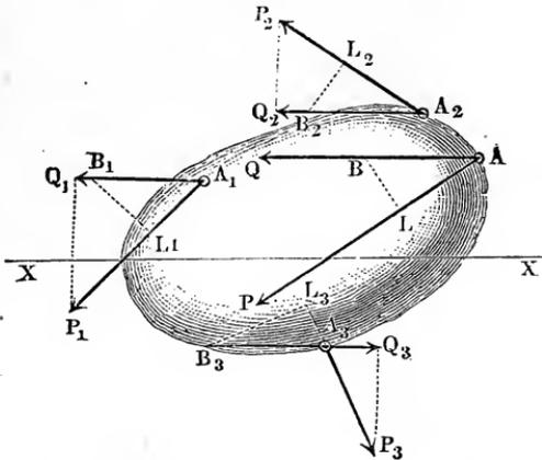
the sum of the work done by the components, and consequently, when the forces balance each other, this sum is  $= 0$ . If the projections of the common space  $A_1 B_1 = A_2 B_2$ , etc., upon the directions of the forces are  $A_1 L_1, A_2 L_2$ , etc.,  $= s_1, s_2$ , etc., the work done by the resultant is
