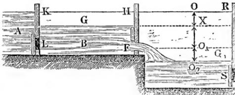
two kinds of locks, namely, the single and the double. The *single lock* consists of a chamber  $B$ , Fig. 790, which is separated from the water in the *head bay*  $A$  by the gate  $H F$  and from that in the *tail bay*  $C$  by the gate  $R S$ . The *double lock*, Fig. 791, on the contrary, consists of two chambers with an upper gate  $K L$ , a middle one  $H F$ , and a lower one  $R S$ .
