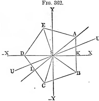
§ 230. **Polygonal Girders.**—The foregoing theory can be applied to a body with a regular polygonal cross-section  $ACDE$ , Fig. 362, whose neutral axis  $\bar{X} X$  is at the same time an axis of symmetry. Since such a polygon can be resolved into triangles, having a common vertex  $S$ , the determination of its moment
