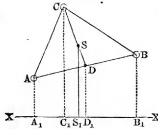
$NS = \frac{1}{3} CH$ ; the centre of gravity  $S$  is at a distance from the base of the triangle equal to one third of the altitude.
