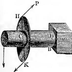
tion from the neutral axis, we have the maximum strain produced in the direction of the axis by the force  $Q$
