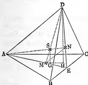
to the triangle  $DA S$ . In consequence of this similarity we have also  $MS = \frac{1}{3} DS$  or  $DS = 3 MS$  and  $MD = MS + SD = 4 MS$ , or inversely  $MS = \frac{1}{4} MD$ . The distance of the centre of gravity of a triangular pyramid from its base along the line joining the centre of gravity  $M$  of the base to the apex  $D$  of the pyramid is equal to one-fourth of this line.
