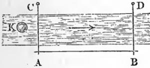
the other side of the river that the lines  $CA$  and  $DB$  shall be perpendicular to  $AB$ . Placing ourselves behind  $A$ , we note the instant the float  $K$ , which has been placed in the water some distance above, arrives at the line  $AC$ , and then passing behind
