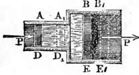
inwards, it presses the prism of water  $F s$  out of its tube, and the piston  $B E = F_1$  moves outwards the distance  $B B_1 = s_1$ , and leaves behind it the prismatic space  $F_1 s_1$ . Now as we have
