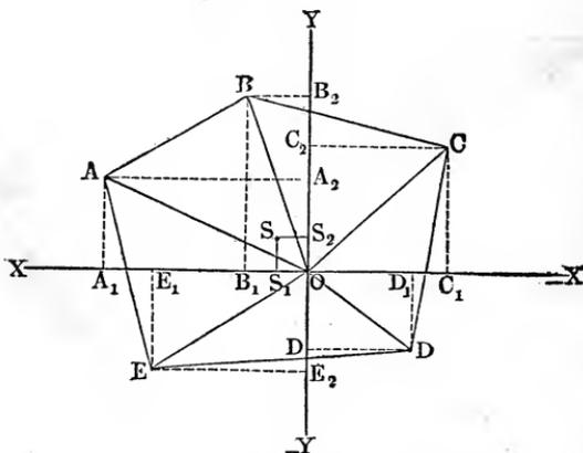
nates of its corners  $A, B, C$ , etc., and the co-ordinates of its centre of gravity are required.
