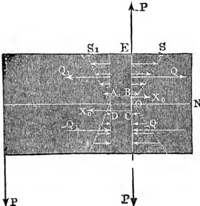
$C D$  remain free from the action of extraneous forces; for the neighboring elements of the body are subjected to the same axial strain as the supposed element  $A B C D$  itself. But the case is different when the body is bent; for on one side  $A B$  of the element  $A B C D$  a strain is produced which is opposite in direction to that upon the other side  $C D$  of the element, and in consequence of the cohesion
