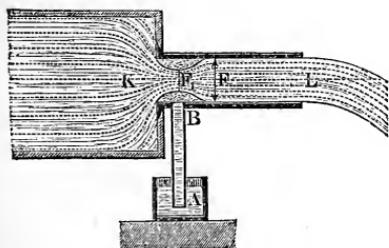
the water to the walls of the tube, which causes it to fill the end  $FL$  of the tube completely. The pressure of the water discharging from the tube is that of the atmosphere, but the contracted cross-section  $F_1$  is only  $a$  times as great as that  $F$  of the tube; the velocity  $v_1$  at that point is therefore  $\frac{1}{a}$  times as great as the velocity
