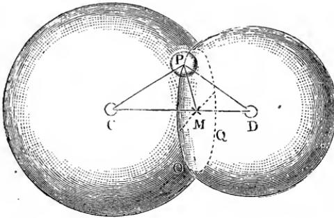
other point *P* of the body, when put in motion, will describe a path, which lies upon the surface of a sphere, whose centre is the fixed point *C* and whose radius is the distance *CP* of the other point from *C*. If, on the contrary, we fasten a body in two points *C* and *D*, the paths described by all other points in consequence of any possible motion would be circles; for the path of each point is the intersection *OPQ* of two spherical surfaces described from the two fixed points.
