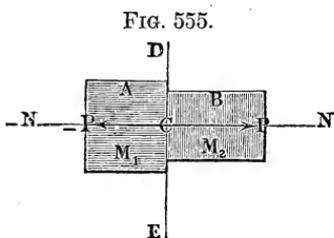
*B*, Fig. 555, be  $F_1$  and  $F_2$ , their length  $l_1$  and  $l_2$ , and their moduli of elasticity be  $E_1$  and  $E_2$ . If they impinge upon one another, the compressions produced are, according to § 204,
