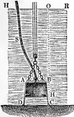
In the beginning the bell with its opening  $C D$  stands above the level of the water  $H R$ , so that the whole space  $V$  is filled with air at a pressure equal to that of a column of water, whose height is  $= b$ . If afterwards the bell sinks to a depth  $O C = x$  and a volume  $W$  of water is thus introduced into it, the volume of the inclosed air, when none is pressed back through the hose, becomes  $V - W$  and the height of the water barometer becomes  $b + x - y$ ; hence
