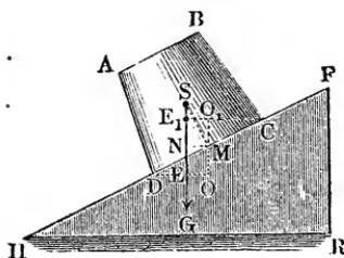
219, is different from that of a body upon a horizontal plane  $H R$ . If  $D M = e$  and  $M s = a$  are the rectangular co-ordinates of the centre of gravity  $S$ , we have for the arm of the stability
