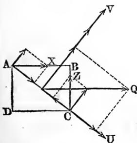
strains in an element  $A C$ , Fig. 425, of the surface, whose plane forms the variable angle  $B A C = \psi$  with the longitudinal axis of the body, we decompose the tensions in the projections  $A B$  and  $B C$  of this element of the surface into two components, one of which acts in the plane of  $A C$  and the other at right-angles to it, and we then combine the components in  $A C$ , so as to form a single shearing force, and the components, acting
