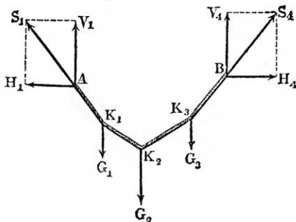
pounds; required the axial tensions, supposing the extremities  $A$  and  $B$  to have the same angle of inclination. The vertical tensions at the ends are equal and are
