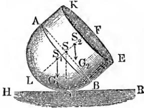
But if a body is supported in two points upon the horizontal surface of another body, the conditions of equilibrium require, that the vertical line of gravity shall pass through the line joining the two points of support. If, finally, a body rests upon three or more points on a horizontal plane, equilibrium exists, when the vertical line of gravity passes through the triangle or polygon formed by joining these points by straight lines.
