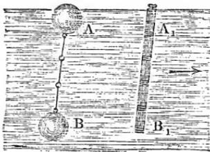
convenient, when it is used for measurements in canals and ditches, to have it made of short pieces which can be screwed together. The one used by the author is composed of 15 hollow pieces, each one decimeter long. In order to make it float nearly perpendicularly, the lower part is filled with enough shot to prevent more than the head from projecting above the water.
