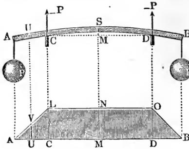
is supported at two points  $C$  and  $D$ , which are at the same distance  $AC = BD = l_1$  from the ends, the reaction of each of these points of support is equal to the force  $P$ , and for a point  $M$  upon  $CD$  the moment of flexure
