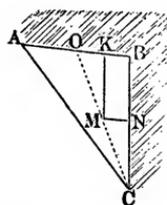
not reach the surface of the water, then, if the distance  $K L$  of the lower line  $C D$  from the surface of the water =  $l_1$ , and that  $K O$  of the upper one  $A B$ , =  $l_2$ , we have the distance  $K M$  of the centre of pressure from the surface of the water
