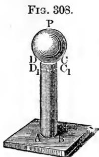
of course not necessary that both should be motive forces. The action is the same, when the body is firmly suspended or supported at one end and at the other end subjected to a pull or to a thrust. We can obtain an example of this case either by suspending to a prism  $A B C D$ , Fig.
