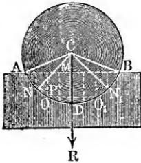
Let us divide the arc  $A D B$  along which the bearing and axle are in contact into very many parts, such as  $A N, N O$ , etc., whose projections upon the chord  $A B$  are equal, and let us suppose that each one of these parts transmits from the axle to the bearing equal portions  $\frac{R}{n}$  of the whole pressure  $R$ . Here  $n$
