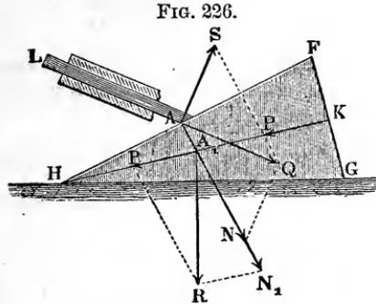
$\overline{KP} = \overline{A_1P} = P$  of the wedge to form a resultant  $\overline{A_1R} = R$ , whose direction must be perpendicular to the base  $GH$  of the wedge, in which case it will be transmitted completely to the support of the wedge. The parallelogram of forces  $A_1 P R N_1$  gives
