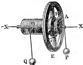
EXAMPLE.—Let the weight upon the wheel, Fig. 492, be  $P=60$  pounds and that on the axle,  $Q=160$  pounds; let the arm of the former be  $CA = a = 20$  inches and that of the latter  $DB = b = 6$  inches,
