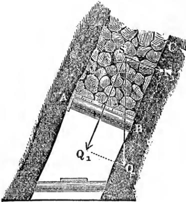
the loose masses of stone upon the floor and denoting the angle formed by the terminal surfaces of the prop with its cross-section by  $\delta$ , and the inclination of the floor  $BC$  to the horizon by  $\beta$ , we obtain  $Q_1 = Q \sin. \beta$  and
