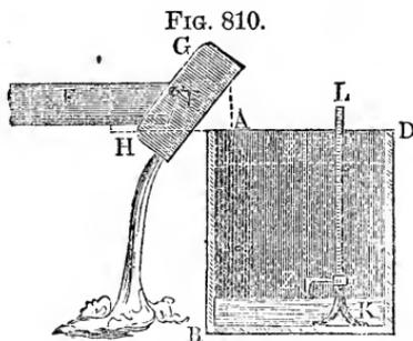
by means of which the water can be made to flow into the vessel or alongside of it. In order to determine accurately the depth of the body of water, we employ a scale *K L*. If, before we begin the measurement, we lower the pointer *Z* until it touches the surface of the water, which, perhaps, may only cover the bottom, and read off on the scale the depth of the
