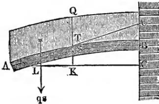
where  $Q = q x$ ), the curvature increases or diminishes with  $x$  and becomes with it a maximum and minimum. When, on the contrary, the cross-section  $F$  of the body is different in different points, then  $W = \Sigma (F' z^2)$  is also variable, the radius of curvature is proportional to the quotient  $\frac{W}{P x}$  and the curvature itself to
