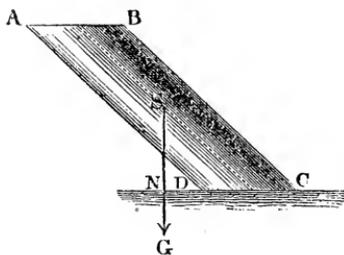
§ 142. **Formulas for Stability.**—A force  $P$  whose direction is not vertical tends not only to overturn, but also to push forward the body  $ABCD$ , Fig. 209. Let us suppose that there is an
