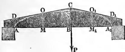
In like manner we can construct the girder  $ANA_1$ , Fig. 410, which is supported at its extremities  $A$  and  $A_1$ , of two portions, bounded by plane surfaces, which have a common height  $BC = h_1 = 1,0607 h$  at the point of ap-
