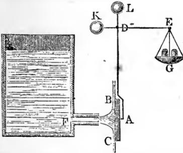
represented in Fig. 848. *BC* is the surface subjected to the action of the stream, *G* the scale-pan for receiving the weights, *D* the axis of rotation, and *K* and *L* are counter weights.
