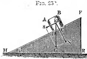
*A C*, Fig. 253, lies upon an inclined plane *F H*, whose angle of inclination is  $F H R = a$ , we can decompose its weight into the normal pressure  $N = G \cos. a$ , and into the force  $S = G \sin. a$  parallel to the plane. The first force causes the friction  $F = \phi G \cos. a$ , which resists every motion upon
