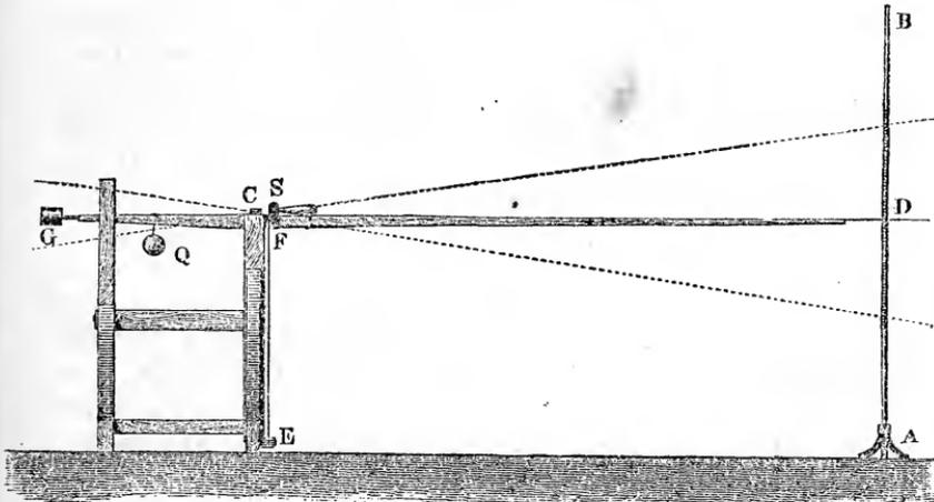
long, the counter-balance  $G$  and the sliding weight  $Q$ . The wire  $E F$ , which was about 4 feet long, was firmly fastened at one end  $E$  and the other was wound round a pin  $F$ , which was turned by the
