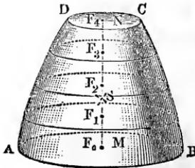
If the areas of the cross-sections are  $F_0, F_1, F_2, F_3, F_4$  and the total height or distance  $M N$  between the two parallel planes farthest apart =  $h$ , we have, according to Simpson's rule, the volume of the body
