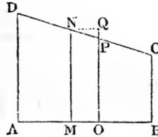
of velocity  $CD$  therefore a curve, the acceleration at every instant is different, and consequently it is not really the difference  $PQ$  of the velocities  $OP$  and  $MN = OQ$ , Figs. 60 and 61, which are those at times differing one second  $MO$  from each other, but it
