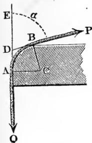
Here the angle of deviation is  $EDB = a^\circ =$  angle at the centre  $ACB$  of the arc  $AB$  of the cord; if we divide the same in  $n$  equal parts and regard the arc  $AB$  as consisting of  $n$  straight lines, we obtain  $n$  edges with the deviation  $\frac{a^\circ}{n}$ , and therefore the equation between the power and the load is as in the foregoing paragraph
