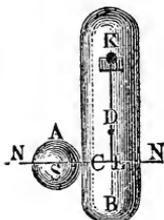
Fig. 562, which has a *motion of translation* and is *unretained*, impinges upon a body  $B C K$ , *movable around an axis  $K$* , we can find the velocities after impact by substituting in the formulas of the preceding paragraph instead of  $a_1 \varepsilon_1$  and  $a_1 \omega_1$  the velocities of translation  $c_1$  and  $v_1$  and instead of
