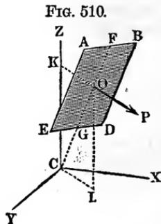
This formula holds good also for a *rectangular plate*  $ABDE$ , Fig. 510, which is divided into two similar rectangles by the axial plane  $COZ$ , and whose plane is at right angles to this axial plane; for the points of application of the centrifugal forces of the slices,
