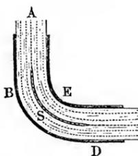
The resistance to water flowing through bends can be *diminished* by enlarging the cross-section of the pipe, as in  $B D E$ , Fig. 765, or by inserting in it a *thin partition*, like  $S$  in  $B D E$ , Fig. 766; for in the first case the velocity  $v$ , and in the second the ratio  $\frac{a}{r}$  is smaller, and consequently the coefficient of resistance  $\zeta$  is rendered less.
