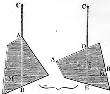
if it be suspended in another way we find a second line of gravity  $DE$ . The point of intersection  $S$  of the two lines is the centre of gravity of the whole body. If we suspend a body by means of an axis, or if we balance it upon a sharp edge (knife edge), the vertical plane passing through the axis or knife edge is a plane of gravity.
