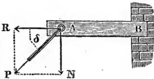
$R = P \cos. \delta$  acts as a tensile force and the other  $P \sin. \delta$  as a bending one upon the body, and the strain
