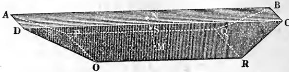
feet wide on top, what is the distance of its centre of gravity from its base? Here  $b_1 = 40$ ,  $l_1 = 250$ ,  $b_2 = 15$ ,  $l_2 = 400$ , and  $h = 20$ , and consequently the distance is
