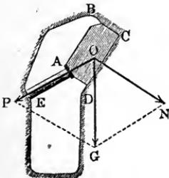
If the prop was horizontal, we would have  $\beta = -50^\circ$  and  $\text{tang. } \rho = 0,75$ , or  $\rho = 36^\circ 52'$ , from which we obtain
