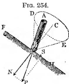
body counteracts not only the normal pressure  $N$  of another body *A B*, but also any oblique pressure  $P$  when the angle  $N B P = a$  formed by its direction with the normal to the surface does not exceed the angle of friction; since the force  $P$  gives rise to the normal pressure  $\overline{B N} = P \cos. a$ , and to the lateral or tangential pressure  $\overline{B S} = S = P \sin. a$  and since the normal pressure  $P \cos. a$  produces the friction  $\phi P \cos. a$ , which opposes
