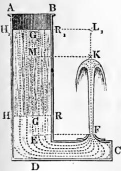
If above the level  $H R$  of the water  $H E R$  in a vessel  $A C D$ , Fig. 673, there is still a column of liquid  $H R_1$ , whose height  $G G_1 = h$  and whose heaviness  $= \gamma_1$ , while that of the water is  $= \gamma$ , we can replace the latter by a column of water whose
