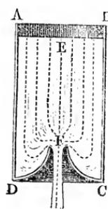
order to reach the orifice. Both cases are represented in Figures 704 and 705. In the first case the coefficient of efflux is nearly 1, viz.: 0,96 to 0,98, and in the second case, according to the measurements of Borda, Bidone and of the author, its mean value is = 0,53.
