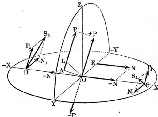
$D$ , is acted upon by a system of forces, in order to determine the conditions of its equilibrium we refer (according to § 97) the
