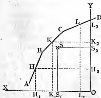
133, we first obtain the distances of the centres  $H, K, L$  of the lines  $A B = l_1, B C = l_2, C D = l_3$ , etc., from the two axes  $O X$  and  $O Y$ , viz.,  $H H_1 = y_1, H H_2 = x_1, K K_1 = y_2, K K_2 = x_2$ , etc. The distances of the centre of gravity from these axes are
