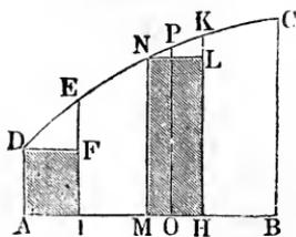
The first two of these lines denote the initial and final velocities, and the last one is determined by the extremities ( $N$ ) of the different lines representing the velocities corresponding to the intermediate times ( $M$ ). Accord-
