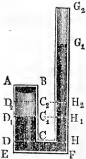
if we then compress it by pouring in quicksilver, until it occupies one-half, one-quarter, etc., of its original volume, we will find that heights  $G_1H$ ,  $G_2H_2$ , etc., of the surface of the mercury in the tube are equal to the height of the barometer  $b$  multiplied by one, three, etc. Consequently, if we add the height corresponding to the pressure of the atmosphere, we find that the tension is double, quadruple, etc., that of the original volume.
