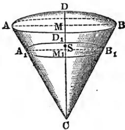
The centre of gravity of this curved surface is also that of the spherical sector; for the weights of the elementary pyramids are equally distributed over this surface, which is therefore everywhere equally heavy.
