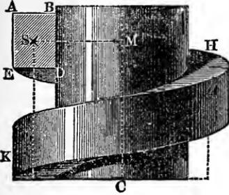
*A H K*, Fig 171, of a screw is determined by the product of its cross section *A B D E* by the circumference of the circle, whose radius is the distance *M S* of the centre of gravity *S* of the surface *A B D E* from the axis *C M* of the screw.
