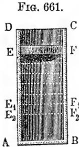
While the piston describes a very small portion  $E_1 E_2 = \sigma$  of the space, the tension  $p_1$  can be regarded as constant, and the work done is =  $F p_1 \sigma = \frac{F p s \sigma}{s_1}$ ,  $F$  denoting the area of the piston.
