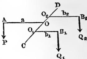
upon the axis takes place between the two points of support or bearings  $C$  and  $D$ . If we denote by  $l$  the length of the axis  $CD$  of the lever or the distance of the fulcrums from each other and by  $l_0, l_1, l_2, \dots$  the distances  $CO, CO_1, CO_2$  of the planes of revolution from the fulcrum  $C$ , the pressures  $R_2$  and  $R_1$  on the bearings at  $D$  and  $C$  are determined by the following formulas
