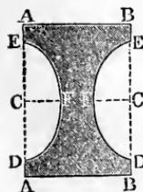
$b$  and  $h$  denoting the length  $A B$  and the height  $A A = B B$  of the rectangular cross-section  $A B B A$ , and, on the contrary,  $a_1$  and  $b_1$  the semi-axes  $C E$  and  $C F$  of the semi-elliptical hollow  $D F E$ .
