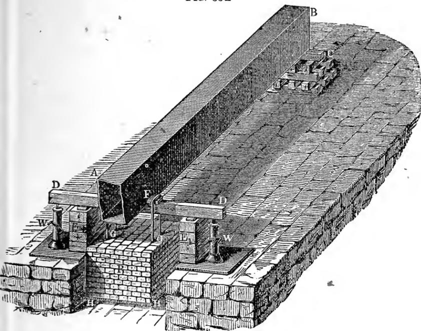
applied not to the centre of a girder supported at both ends, but to one end of a girder, which was supported in the middle and the other end of which was fastened by a bolt to the foundation.
