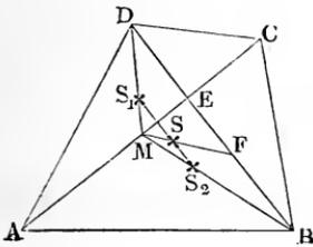
sided figure  $A B C D$ , Fig. 139, we can divide it by means of the diagonal  $A C$  into two triangles, and then determine their centres of gravity  $S_1$  and  $S_2$  by means of the foregoing rules; thus we obtain a line of gravity  $S_1 S_2$ . If we again divide the figure by the diagonal  $B D$  into two other triangles, and determine their centres of gravity, we obtain a second line of gravity, whose
