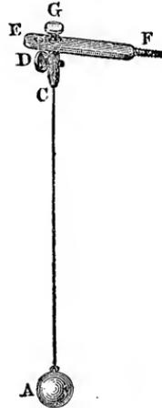
whose upper end is fastened into a ferrule  $D$  by a clamping screw. This ferrule has upon its end a screw, which passes through the arm  $E F$  and is made fast by a nut  $G$ , when the arm has been screwed into a door-frame or some other solid support. If the length is  $C A = 0,2485$  or nearly  $\frac{1}{4}$  meter, then this pendulum will beat half-seconds for almost an hour, although the arcs in which it oscillates will continually decrease.
