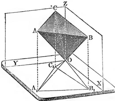
REMARK.—The determination of the volume of a triangular pyramid from the co-ordinates of its corners is very simple. If we pass through the apex  $O$  of such a pyramid  $A B C O$ , Fig. 154, three co-ordinate planes  $X Y, X Z, Y Z$ , and denote the distances of the corners  $A, B, C$  from these planes by  $z_1, z_2, z_3; y_1, y_2, y_3$  and  $x_1, x_2, x_3$ ,
