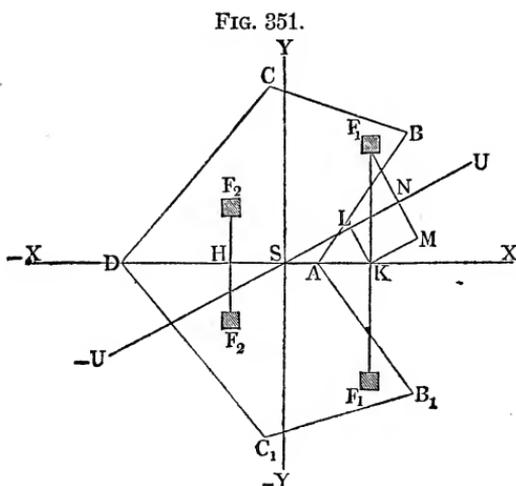
plane of flexure is an axis of symmetry of the figure, there will be still another relation between the moments of flexure of the body. Let  $SK = x$  and  $KF_1 = y$  be the co-ordinates of an element of the surface  $F_1$  in reference to the system of axes  $\overline{XX}$  and  $\overline{YY}$ , and let  $F_1N = v$  be the distance of the same element from the axis  $\overline{UU}$ ,
