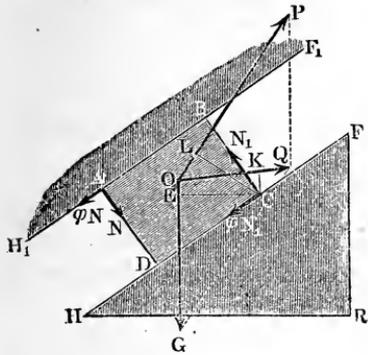
through the supporting surface  $C D$  of the body  $A C$ . Otherwise the body  $A C$ , Fig. 263, has a tendency to revolve or overturn about the outer edge  $C$ , and this tendency increases with the distance  $C K = e$  of this edge from the direction  $O Q$  of the resultant  $Q$ .
