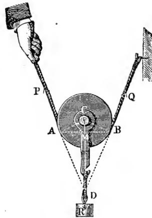
whose circumference a string is laid, the extremities of which are pulled by the forces *P* and *Q*. The block (Fr. chape; Ger. Gehäuse or Lager) of a fixed pulley (Fr. p. fixe; Ger. feste R.), in which the axles or journals rest, is immovable. That of a movable pulley (Fr. p. mobile; Ger. lose R.) on the contrary is free to move.
