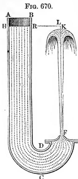
§ 398. **Velocities of Influx and Efflux.**—If the water flows in with a certain velocity  $c$ , we must add to the mechanical effect  $h Q \gamma$  the energy  $\frac{c^2}{2g} Q \gamma$ , possessed by the influent water and corresponding to the height  $h_1 = \frac{c^2}{2g}$ , due to the velocity; hence we must put
