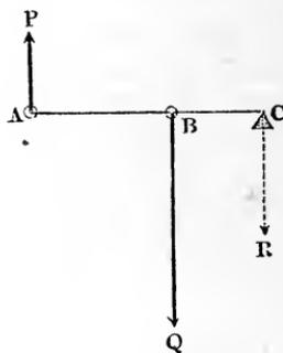
*the moment of the load*, or also  $P : Q = b : a$ , i.e. *the force is to the load as the arm of the latter is to the arm of the former*. The pressure on the fulcrum is  $R = P + Q$ .
