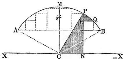
the arc into a very great number of parts and determine their statical moment in reference to an axis  $X\bar{X}$ , which passes through the centre  $C$  and is parallel to the chord  $AB = s$ . If  $PQ$  is a part of the arc and  $PN$
