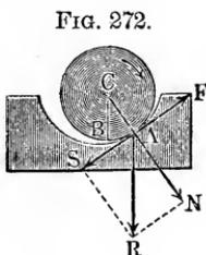
If no rotation takes place, the axle presses upon the point  $B$ , through which the direction of the resulting pressure  $R$  passes; if the shaft begins to rotate in the direction  $A B$ , the axle rises in consequence of the friction on its bearing, until the force  $S$  tending to move it down balances the friction  $F$ . The resultant  $R$  is decomposed into a normal force  $N$  and a tangential one  $S$ ,  $N$  is transmitted to
