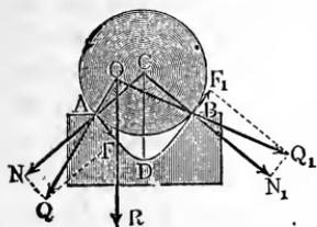
If the bearing  $ADB$ , Fig. 274, is triangular, the axle is supported at two points  $A$  and  $B$  and at both of them friction must be overcome. The resulting pressure  $R$  is decomposed into two components  $Q$  and  $Q_1$ , each of which is again decomposed into a normal stress  $N$  or  $N_1$  and into a tangential one, which is equal to the friction  $F = \phi N$  and  $F_1 = \phi N_1$ .
