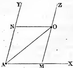
We can convince ourselves of the correctness of this proceeding by supposing the spaces  $x$  and  $y$  described not simultaneously, but one after the other. By virtue of one motion the body describes the space  $AM = x$ , and by virtue of the other from  $M$  in the direction  $AY$ , that is on a line  $MO$  parallel to  $AY$ , the space  $AN = y$ . If we make  $MO = AN$ , we obtain in  $O$
