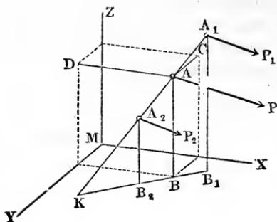
the whole system can therefore be turned about this point without its ceasing to be the point of application, as long as the forces remain parallel.
