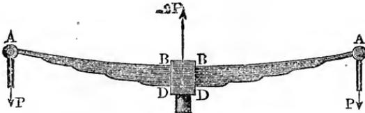
total proof load is  $2 P$ ; the length must not, however, be measured from the middle, but from the ends  $B D, B D$  of the fastening.
