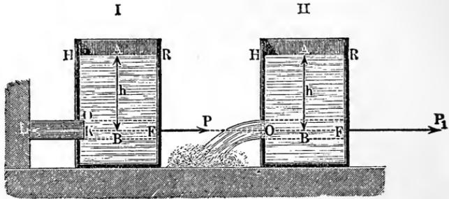
the stopper. If the stopper is removed and the water allowed to flow through the opening  $O$ , as in II, the reaction of the discharging water increases this pressure  $P$  from  $F h \gamma$  to  $P_1 = 2 F h \gamma$ , as will be shown hereafter.
