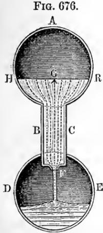
EXAMPLE—1) If the piston of a fire engine is 12 inches in diameter and it is pressed down in the cylinder with a force of 3000 pounds, and if there are no resistances in the pipes and hose, the water will
