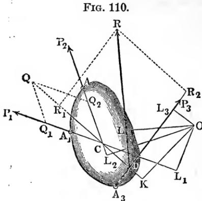
point (see § 80); the rules given in § 80 can be employed to calculate the first two elements of the resultant, but the third element, viz., the position of the resultant or its line of application, must be determined by means of the formula for the statical moments. If  $O L_1 = a_1$ ,  $O L_2 = a_2$ ,  $O L_3 = a_3$  and  $O L = a$  are the arms of the three component forces  $P_1$ ,  $P_2$ ,  $P_3$  and of their resultant
