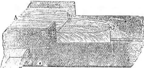
REMARK.—Such an apparatus for dividing the water was constructed of sheet iron for the *Wernergroben* at Freiberg by *Oberkunstmeister Schwamkrug*. It discharges through a rectangular orifice  $D$ , which is 5 feet long and 1 foot high, almost invariably 40 cubic feet of water per second, while the remaining water passes over the overfall, the sill of which lies 2 feet above the upper edge of the orifice, and flows on in the ditch to where it is wanted.
