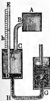
$S$ , the enclosed air will be compressed and the mercury will rise a certain distance  $h$  in the manometer, which distance can be read off upon the scale. If again  $V_0$  is the volume  $A B C D$  of the air,  $V_1$  the required volume of the body placed in it and  $V$  the volume of the mercury, which has been pressed into the air-vessel, we have in this case
