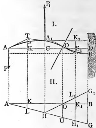
towards  $B$  the curvature of the girder gradually increases in the opposite direction. If in the second case, Fig. 342, the forces  $P$  and  $P_1$  are equal, for a point  $K_1$  between  $A_1$  and  $B$ ,
