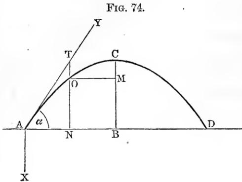
of elevation  $Y A D = a$ , Fig. 74, ascends to a certain height  $B C$ , which is called the *height of projection* (Fr. hauteur du jet, Ger. Wurfhöhe), and it reaches the horizontal plane from which it started in  $A$ , at a distance  $A D$  from it, which is called the *range of projection* (Fr. amplitude du jet, Ger. Wurfweite).
