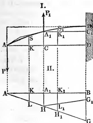
If, as in Fig. 340,  $P_1 l_1 < P(l + l_1)$ , the beam is bent in one direction only; but if  $P_1 l_1 > P(l + l_1)$ , there is no flexure at the point  $A$  and also at a point  $O$ , Fig. 343, where a point of inflection is formed (see Art. 14, *Introduction to the Calculus*), and from  $O$
