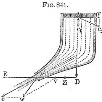
has an opening  $F$ , through which the water issues, this force undergoes a change not only because a portion of the wall of the vessel is absent, but also because the water, which issues from the orifice, like every other body, which changes its conditions of motion, reacts by virtue of its inertia. The change in the motion of a body may consist either of a change of velocity, or of a change of direction, and, there-
