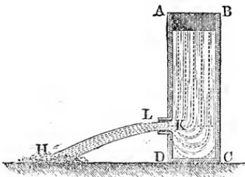
we can also see that the range  $ER$  is smaller than the range  $DH$ . This condition of efflux exists only when the length of the tube is the given one; if the tube is shorter, e.g. as long as wide, the vein  $KR$ , Fig. 717, does not touch the sides of the tube, the latter has then no influence upon the efflux, and the stream issues from it as from an orifice in a thin plate.
