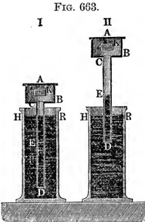
Now if  $V_0$  is the volume of the space  $ABC$ ,  $V_1$  the required volume of the body  $K$ , which is placed in it,  $V$  the volume of the column of air  $CE$ ,  $b$  the height of the barometer and  $h$  that of the column of mercury  $DE$ , we have,
