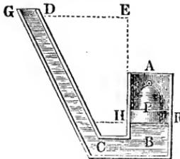
If *F* is the area of the cross-section *HR* of a piston, Fig. 637, in one leg *AB* of two communicating tubes and *h* the head of water or the height *EH* of the surface of the water in the second tube *CD* above *HR*, we have the pressure upon the surface of the piston
