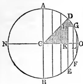
The sum of the moments of these slices gives the moment of flexure of the semi-cylinder  $A O B$ , and by doubling this moment we obtain the moment of flexure of the entire cylinder. If  $r$  denotes the radius  $C A = C O$  of the circular cross-section  $A O B N$ , a division  $D G$  of the arc =
