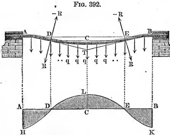
$D$  and  $E$ , Fig. 392, do not lie at the centres of the semi-girders; for the deflecting forces  $R, R$  of the portions  $AD$  and  $BE$  are
