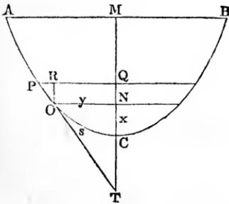
formed by the tangent  $OT$  to a point  $O$  of the catenary  $ACB$  with the horizontal co-ordinate  $ON$ , when the arc  $CO$  is denoted by  $s$  and the horizontal tension by  $H = c \gamma$ ,
