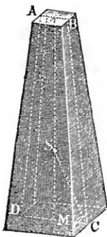
necessary to overturn, the granite obelisk  $ABCD$ , Fig. 214, when its height is  $h = 30$  feet, its upper length and breadth  $l_1 = 1\frac{1}{2}$  and  $b_1 = 1$  foot and its lower length and breadth  $l_2 = 4$  feet and  $b_2 = 3\frac{1}{2}$  feet? The volume of this body is
