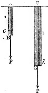
This hypothetical empirical quantity  $\frac{1}{\text{tang. } a} = \text{cotg. } a$  is called the *modulus of elasticity* (Fr. coefficient d'élasticité; Ger. Elasticitätsmodul) of the body or material and will hereafter be designated by the letter  $E$ .
