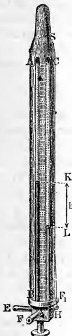
REMARK—1) Although Pitot's tube is not so accurate as the tachometer, yet, on account of its simplicity, it can be highly recommended. The author has discussed this instrument at length in the "Polytechnisches Centralblatt, 1847," and gives there a series of numbers, determined by experiment, and the values of the coefficient  $\psi$  deduced from them. With fine instruments, when the velocities were between 0,32 to 1,24 meters, we found  $\psi = 3,545 \sqrt{h}$  meters.
