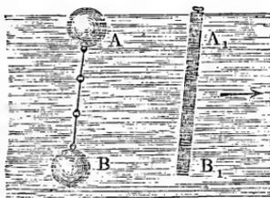
The two balls are united by a string, wire or thin wire chain. We first determine by a single ball the superficial velocity  $c_0$ , and we then determine the
