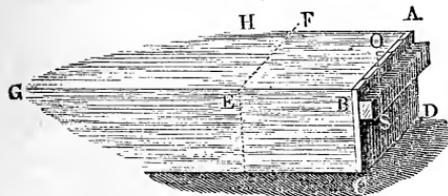
$F = ab$  and the head of water  $SO = \frac{a}{2}$ , and, therefore, the pressure of the water against it is
