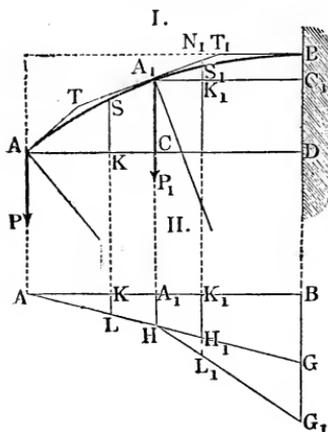
$P_1 l_1$ , and it is positive or negative as  $P(l + l_1)$  is greater or less than  $P_1 l_1$ . In both cases the moment of flexure decreases gradually from  $A_1$ , remaining in the first case, Fig. 340, positive, and,
