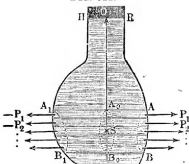
column of water, whose base is the vertical projection  $A_0 B_0$  of the surface at right angles to the given direction and whose height is the depth  $OS$  of the centre of gravity  $S$  of this projection below the surface of the water. The correctness of this assumption is shown directly by the formula
