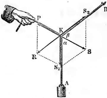
force *P* applied at the knot; for the tensions of the cord *S*<sub>1</sub> and *S*<sub>2</sub> produce the same effect in the knot *K* as two forces equal to them and acting in the same direction as they do, and the three forces are in equilibrium, when one of them is equal and opposite to the resultant of the other two (§ 87). In like manner the resultant *R* of the force *P* and of one of the tensions *S*<sub>1</sub> is equal and opposite to the second tension *S*<sub>2</sub>, etc. We can
