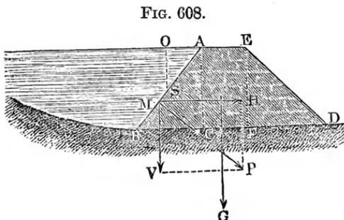
the water, we must consider the longitudinal elevation  $A C$ , and if the vertical pressure is to be determined, the horizontal projection  $B C$  of the surface  $A B$  must be considered as the surface pressed upon. Putting the length of the
