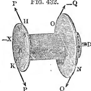
For a *cylindrical shaft* with circular cross-section  $A B$ , Fig. 432, whose radius is  $C A = r$ , the measure of the moment of flexure in reference to an axis  $\bar{X} X$  or  $\bar{Y} Y$  is (according to § 231)
