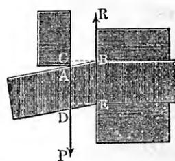
place between  $A$  and  $C$  in a surface  $DD$  at right angles to the axis of the body. The strength of shearing, like that of tearing and
