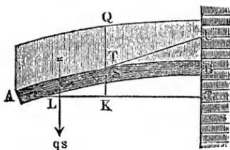
bears a weight =  $q$ , or the whole girder, whose length is  $l$ , bears the load  $Q = l q$ , and a portion of the girder  $A S = s$  the load  $q s$ , we must substitute, instead of the moments
