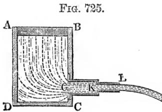
in Fig. 725, where the short tube  $KL$  is inserted into another short tube  $GC$ , and the latter into the vessel  $AC$ . Here, when the water enters the smaller from the larger tube, the stream is imperfectly contracted, and the coefficient of efflux is determined by the last rule. If we put the coefficient of resistance corresponding to this coefficient of efflux =  $\zeta_1$ ,
