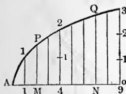
is made equal to the double acceleration ( $2g$ ) of gravity. We can therefore represent graphically the laws of the free fall of a body by the parabola  $APQ$  (Fig. 4), whose parameter  $p = 2g$ . The abscissas  $AM$ ,  $AN$ , of this curve are the space traversed by the body in its fall, and the ordinates  $MP$ , and  $NQ$ , the corresponding velocities.
