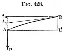
notes the modulus of the elasticity of shearing and  $F$  the cross-section of the beam, the inclination the beam  $A_1 B$  produced by the shearing force is  $\iota = \frac{X_0}{C}$ , and, therefore, the corresponding deflection of the end  $A_1$  of the girder, whose length  $A_0 B = l$ , is
