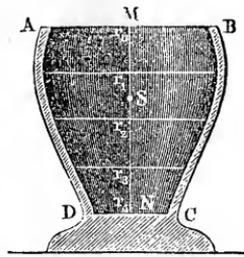
**EXAMPLE 2.** The mean half widths of the vessel  $ABCD$ , Fig. 164, are  $r_0 = 1$  inch,  $r_1 = 1,1$  inches,  $r_2 = 0,9$  inches,  $r_3 = 0,7$  inches, and  $r_4 = 0,4$  inches, and its height  $MN = 2,5$  inches; required the centre of gravity of the space within it. The cross sections are  $F_0 = 1 \pi$ ,  $F_1 = 1,21 \pi$ ,  $F_2 = 0,81 \pi$ ,  $F_3 = 0,49 \pi$  and  $F_4 = 0,16 \pi$ , and therefore the distance of its centre of gravity from the horizontal plane  $AB$  is
