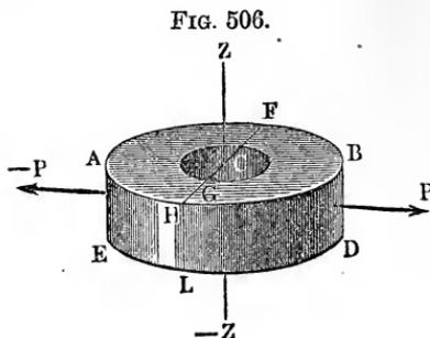
millstone =  $r_1$ , the radius of its eye =  $r_2$ , its height  $A E = H L = l$ , its heaviness =  $\gamma$  and the modulus of ultimate strength =  $K$ , we have the force necessary to tear the stone apart in a diametral plane
