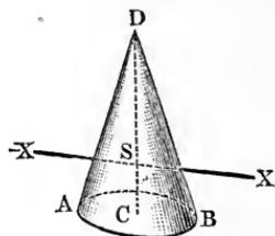
In like manner we find for the *right cone*  $A B D$ , Fig. 486, whose axis of rotation passes through its centre of gravity at right angles to its geometrical axis  $C D$ ,
