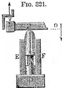
In *experimenting upon rupture by crushing*, the two bases of the body (*A*, Fig. 321) are made parallel, it is then brought between two cylinders *B* and *C*, whose bases are ground flat; while the rounded head of one of the cylinders is acted on by the compressive force, the other is supported by the large bed-plate *D*, and both slide in the interior of cylinder *EF*. The pressure *P* upon the head *H* of the cylinder is
