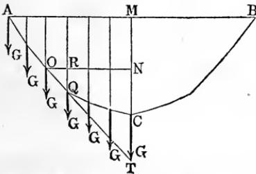
the cord  $A C B$ , Fig. 238, is stretched by the weights  $G_1, G_2, G_3$ , etc., hung at equal horizontal distances from each other. Let us denote the horizontal distance  $A M$  between the point of suspension  $A$  and the lowest point  $C$  by  $b$  and the vertical distance  $C M$  by  $a$ ; let us also put the similarly placed co-ordinates of a point  $O$  of the funicular polygon  $O N = y$  and  $C N = x$ . If the vertical tension in
