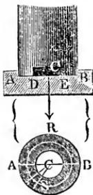
If the radii of the same are  $C A = r_1$  and  $C D = r_2$ , we have here to determine the centre of gravity  $S$  of a portion of a ring. Hence, according to § 114, the arm is
