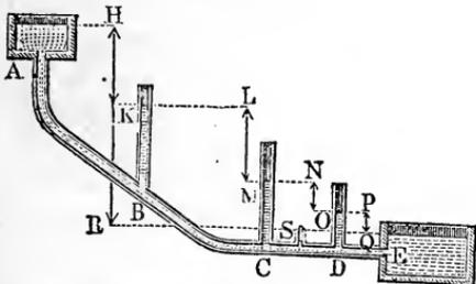
If *v* is the velocity of the water at the point *B*, Fig. 738, where a piezometer is inserted, *l* the length and *d* the width of the portion *A B* of the pipe, *h* the head of water or depth of the point *B* below the level of the water,  $\zeta_0$  the coefficient of resistance for the entrance of the water from the reservoir into the pipe and  $\zeta$  the coefficient of friction, we have the height of the piezometer, which measures the pressure in *B*,
