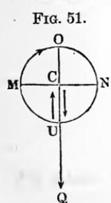
is, its diameter =  $2r$ , and the time equal to  $t$ , it follows that the mean velocity  $c_1 = \frac{2r}{t}$ . The crank in the same time describes a half circle  $\pi r$ , and its velocity is  $c = \frac{\pi r}{t}$ , and therefore the mean velocity of the load  $c_1 = \frac{2}{\pi} c = \frac{2t}{3,141} c$  is 0,6366 times as great as the constant velocity  $c$  of the crank.
