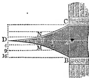
If the height is *constant*, we have  $\frac{u}{b} = \frac{x^2}{l^2}$ ; hence the horizontal section of the girder is a surface limited by the two inverted arcs of a parabola  $BD$  and  $CD$ , as is shown in Fig. 415.
