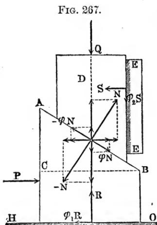
pressure of the block against the guide  $E E$  be  $= S$ . Then  $P$  must balance the forces  $R, \phi_1 R, -N$  and  $-\phi N$ , and  $Q$  the forces  $S, \phi_2 S, N$  and  $\phi N$ .
