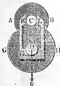
If we neglect the weight of the friction-wheels, the work done when these wheels are employed is  $\psi = \frac{r_1}{a_1 \cos. \frac{a}{2}}$  times as great as
