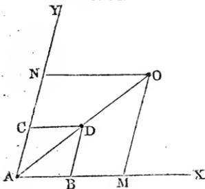
a peculiarity which is possessed only by the right line  $AO$ , Fig. 64. It follows therefore that the direction of the compound motion is always a straight line. If we construct with the velocities  $AB = c_1$  and  $AC = c_2$  the parallelogram  $ABCD$ , its fourth corner  $D$  gives the point where the body is at the end of the first second, but since the resulting motion is rectilinear, it
