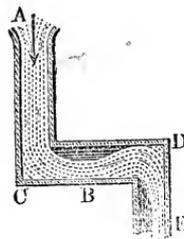
easily explicable, phenomenon of efflux is observed. The second elbow  $BDE$ , Fig. 756, which turns the stream to the same side as the first one  $ACB$ , produces no further contraction of the
