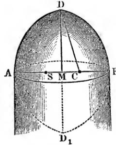
width  $MA = MB = a$  and the altitude  $MD = h$  are given. From the two given dimensions we obtain the radius  $CA = CD$  of the generating circle
