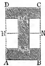
Fig. 355, is determined in exactly the same manner. If  $A B = b$  and  $B C = h$  are the exterior height and width, and if  $A B - A_1 B_1 = b_1$ , and  $B_1 C_1 = h_1$  are the sum of the widths and the height of the two cavities, we have by subtraction
