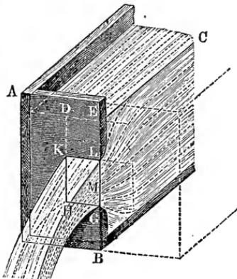
EXAMPLE.—If a rectangular orifice of efflux is 3 feet wide and  $1\frac{1}{4}$  feet high and the lower edge is  $2\frac{3}{4}$  feet below the level of the water, the discharge is
