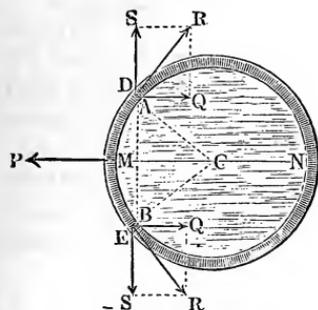
This force is held in equilibrium by the forces of cohesion  $R$ ,  $R$  in the cross-sections  $\overline{AD} \cdot l$  and  $\overline{BE} \cdot l = e l$  of the wall of the pipe; it is therefore equal to the sum  $2 Q$  of the components  $\overline{DQ} = Q$  and  $\overline{EQ} = Q$  of the latter forces, which are parallel to the line  $CM$ . Now if we put  $R = e l T$ , we obtain
