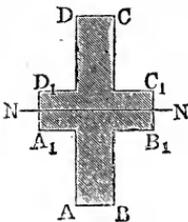
If  $A B = b$  and  $B C = h$  are the height and width of the central portion, and  $A_1 B_1 - A B = b_1$  is the sum of the widths, and  $B_1 C_1 = h_1$  the height of the lateral portions, we obtain by addition the measure of the moment of flexure
