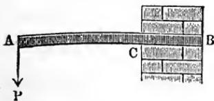
$e = \frac{1}{2} h$ , and, according to § 226,  $W = \frac{b h^3}{12}$ ; hence  $\frac{W}{e} = \frac{b h^2}{6}$ , the proof strength of the girder is  $P = \frac{b h^2 T}{l \cdot 6}$ , and its moment is  $Pl = b h^2 \cdot \frac{T}{6}$ .
