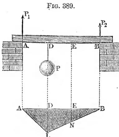
girder supported at both ends  $A$  and  $B$ , Fig. 389, is *not applied at the centre*, but at some intermediate point, situated at the distances  $DA = l_1$  and  $DB = l_2$  from the points of support, the proof load is greater than when the force is applied in the middle. Let us denote the forces, with which the points of support  $A$  and  $B$  react, by  $P_1$  and  $P_2$  and the entire length of the girder  $AB = l_1 + l_2$  by  $l$ . Now, if we put the moment of  $P_1$  in
