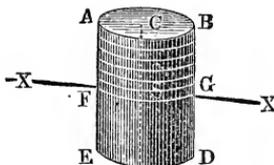
From this we can calculate the moment of inertia of a *cylinder*  $A B D E$ , Fig. 484, which revolves around its diameter  $F G$ , which passes through its centre of gravity  $S$ . Let  $l$  be the half height  $A F$  and  $r$  the radius  $CA = CB$  of the cylinder, then the volume of one half of it is  $= \pi r^2 l$ , and if we pass through it planes parallel to the base and at equal distances from each other, we
