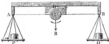
which he called a friction balance (Fr. balance de frottement, Ger. Reibungswage). Here *C* is an axle, which is kept in constant rotation, as, E.G., by a water-wheel, *D* is the bearing, and *A D B* is a lever of equal arms, which produces the pressure between the journal and its bearing by means of the weights *P* and *Q*. The pressure on the axle  $R = P + Q$  produces the friction
