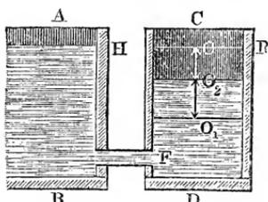
water is constant. If the cross-section of the communicating pipe or orifice =  $F$ ; that of the vessel to be filled =  $G$  and initial difference of level  $O O_1$  of the two surfaces of water =  $h$ , we have, since in this case the level of the water in the second vessel rises with a uniformly retarded motion, the time re-
