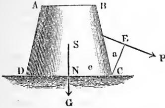
force and another perpendicular  $CN = e$  upon the vertical line of gravity  $SG$  of the body, we have then a bent lever  $ECN$ , to which the formula  $Pa = Ge$  or  $P = \frac{e}{a} G$  is applicable. If, therefore, the exterior force  $P$  is slightly greater than  $\frac{Ge}{a}$ , the body begins to turn around
