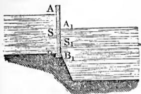
If  $F$  is the area of the portion  $AB$  subjected to pressure on one side of the surface, and  $h$  the depth  $AS$  of its centre of gravity below the surface of the water, and if  $F_1$  is the area of the portion  $A_1 B_1$  on the other side, which is subjected to the pressure of the water, and  $h_1$  the depth  $A_1 S_1$  of its centre of gravity below the corresponding surface of the water, the required resultant will be
