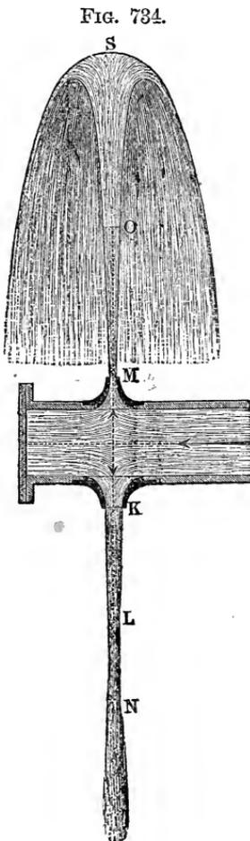
remains continuous and is not broken up by the air, its cross-section  $L$  decreases more and more as the distance  $KL = x$  from the orifice increases. If  $c$  is the velocity of efflux and  $v$  the velocity at  $L$ , we have
