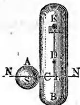
The extremity  $L$  of the distance or lever arm  $a = k_2 \sqrt{\frac{M_2}{M_1}}$ , which corresponds to the maximum velocity, or the point, where the latter line intersects the line of impact, is sometimes, though incorrectly, called the *centre of percussion*; a more correct term would be the *point of percussion*.
