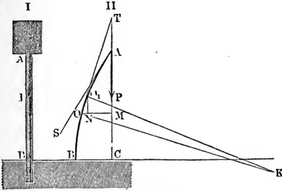
under these circumstances, are very different from what they are where the force acts, as we have seen in § 214, etc., at right angles to this axis. The neutral axis *A B* (*II*) assumes in this case another form; for the lever arm of the force *P* is represented by the ordinate  $MO = y$  and not by the abscissa  $AM = x$ , and its moment is not  $Px$ , but  $Py$ ; consequently the radius of curvature  $\overline{KO} = r$  is determined by the expression
