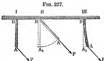
the direction of the force, and an elastic body  $AB$ , Fig. 227, III, resists the force  $P$  to a certain extent only, so that its axis undergoes a certain deflection. Cords, ropes, straps and in a certain sense chains are representatives of flexible bodies, although they do not possess perfect flexibility. These bodies will be the subject of the present chapter; elastic bodies, or rather the elasticity of rigid bodies, will be treated of in the fourth section.
