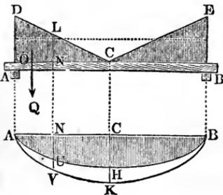
of the planes  $CD$  and  $CE$ , which bound the load, we have the weight of the prism  $ACD = BCE$  of the load, sustained by one point of support,
