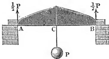
has the form of a parabola, whose vertex  $E$  coincides with the extremity or point of application of the load  $P$ .
