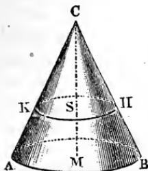
weight of a column of water, whose base is the base of the cone and whose height is two-thirds the length of the axis  $CM$ ; for the horizontal projections of the surface of a right cone, as well as the surface itself, can be decomposed into elementary triangles, and the centre of gravity  $S$  of the surface of the cone is at a distance from the apex of the cone equal to two-thirds of its height  $h$  (§ 116). If  $r$  is the radius of the base and  $h$  the height of the cone, we
