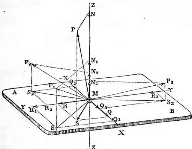
form the edges of a rectangular parallelepipedon (parallelepipedon of forces):
