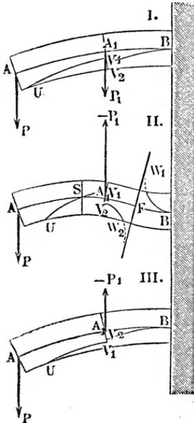
REMARK.—If the girder, as, E.G.,  $A A_1 B$ , Fig. 444, I, II, III, is acted upon by two forces, two or even three displacements of the neutral axis from the centre of gravity may take place. If the two forces act in the same direction as represented in Fig. 444, I, this displacement on one side of the cross-section  $A_1$  is determined by the formula
