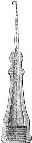
Hence  $l_1 = 51,54$  and  $l_2 = 20,46$  lines and the width at  $B$ , where the conical surfaces meet each other, is  $d_3 = d_2 + 2 l_1 \tan \delta = 7 + 2 \cdot 51,54 \cdot 0,04362 = 11,53$  lines. Since this place is rounded off, we can put  $d_3 = 13$  lines; hence for the outlet piece
