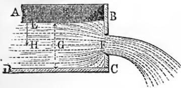
In the experiments made by the author with Poncelet's orifices the head of water was measured 1 meter back from the plane of the orifice; they gave
