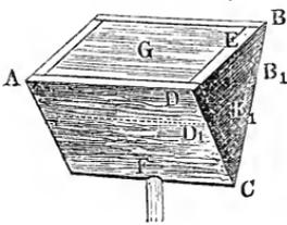
a horizontal *triangular prism*, the time in which it will empty itself is found in the following manner. If we divide the height  $C E = h$  into  $n$  equal parts and pass horizontal planes through the points of division, the whole mass of water will be divided into equally thick horizontal layers, whose common length is  $A D = l$  and whose width diminishes from the surface downwards.
