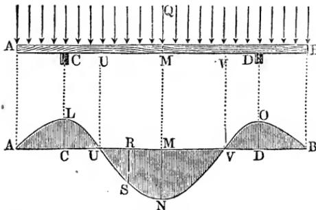
397, with  $q$  per running foot, under certain circumstances the moment of flexure for some points is positive, and for others negative, and therefore at two points  $U$  and  $V$  it is equal to zero.
