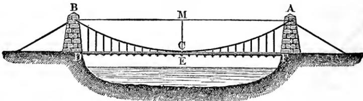
without weight or very light in proportion to that of the loaded bridge  $DE F$ , the latter weights alone would have to be considered, and the chain  $ACB$  would form a parabola.
