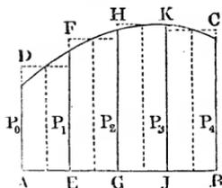
In every case it is necessary to divide the space  $A B = s$  (Fig. 88), in  $n$  (as many as possible) equal parts, such as  $A E = E G = G J$ , etc., and to determine the forces  $E F = P_1$ ,  $G H = P_2$ ,  $J K = P_3$ , etc., at the ends of these portions of the path. If we put the initial force  $A D = P_0$  and the final one  $B C = P_n$  we have the *mean force*  $P = (\frac{1}{2} P_0 + P_1 + P_2 + P_3 + \dots + P_{n-1} + \frac{1}{2} P_n) : n$ , and consequently its work
