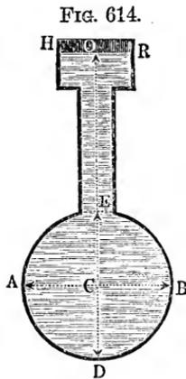
broken, their *walls* must be made of a *certain thickness*, which depends upon the head of water and the internal diameter of the vessel. The rupture of the pipe may be caused either by a transverse or by a longitudinal tearing. The latter form of rupture is most likely to occur, as will appear from the following discussion.
