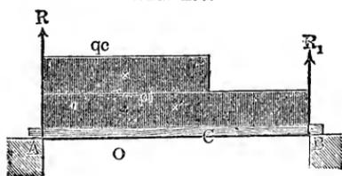
If, finally, the girder  $AB$ , Fig. 427, bears a load  $p l$  equally distributed over its entire length  $l$  and a load  $q c$  equally distributed over the length  $AC = c$ , the reactions of the points of support are
