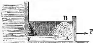
but a portion of the periphery; it limits, moreover, both the stream and the impinging surface. The impinging stream is turned in the direction of the portion of the periphery, which has no border, and is therefore deviated  $90^\circ$  from its original direction;
