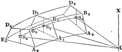
$= F_2$  and the distances  $C S_0 = r_0, C S_1 = r_1$  and  $C S_2 = r_2$  of the centres of gravity  $S_0, S_1$  and  $S_2$  of these cross sections from the central axis  $C X$ . The volume  $V$  of the body is determined by the formula
