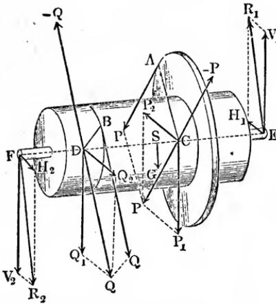
The horizontal pressures  $H_1$  and  $H_2$  are found, as follows, from the horizontal forces  $P_2$  and  $Q_2$ .
