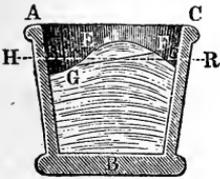
If a vessel  $A B C$ , Fig. 585, is moved forward with the constant acceleration  $p$ , the free surface of the water forms an inclined plane  $D F$ ; for in this case every element  $E$
