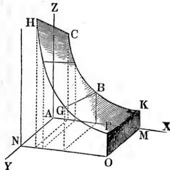
sure  $x$ ,  $AN$  or  $MO$  the temperature  $y$ , and  $OP$  the corresponding volume  $z$ : the co-ordinates of the curve  $PGH$  give the volumes for a temperature  $AN = y$ , and those of the right line  $KP$  the volumes for the same pressure  $AM = x$ .
