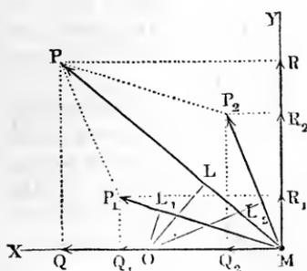
direction of one axis  $Q_1, Q_2$  and  $Q$ , and those in the direction of the other  $R, R_1$  and  $R_2$ , and we have  $Q = Q_1 + Q_2$  and  $R = R_1 + R_2$ . If from any point  $O$  in the axis  $MX$  we let fall the perpendiculars  $OL_1, OL_2$  and  $OL$  upon the directions of the forces  $P_1, P_2$  and  $P$ , we obtain the right-angled triangles  $MO L_1, MO L_2$ , and  $MO L$ , which are similar to the triangles formed by the three forces, viz.,
