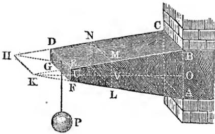
imum of  $\frac{v^2}{x}$  in order to determine the section of rupture. Putting the height  $D G = E F$  of the end  $= h$  and the height  $K U$  of the truncated portion  $H K U = c$ , and assuming, as previously, that
