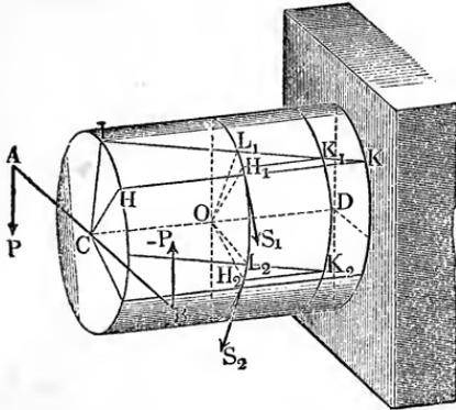
but, in order to avoid any complex change of form, we must assume that the free end is acted upon by a couple  $(P, -P)$  whose plane  $AHB$  coincides with the plane of rotation of the axis  $C D$ . Let us imagine the body to be composed of long fibres, such as  $H K$ , which, in consequence of the torsion, assume the form of a helix, by which  $H K$  comes into the position  $L K$  and the
