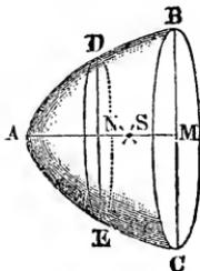
EXAMPLE 1. For the parabolic conoid  $A B C$ , Fig. 162, formed by the revolution of a portion  $A B M$  of a parabola about its axis  $A M$ , we obtain, when we make but one section  $D N E$  through the middle, the following.
