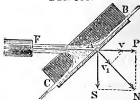
But if the impinging plane  $BC$ , Fig. 853, has a border upon two opposite sides only, the stream divides itself into two unequal parts, the angle of deviation  $a$  of the larger part  $Q_1$  is less than that  $180^\circ - a$  of the smaller part  $Q_2$  and the total impulse in the direction of the stream is
