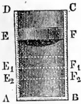
ordinary atmospheric air, which in the beginning acts with a pressure of 14,7 pounds upon each square inch, it will act with a pressure of 29,4 pounds, when we move the piston to  $E_1F_1$  and thus compress the inclosed air into one-half its initial volume; the pressure will become  $3 \cdot 14,7 = 44,1$  pounds, when the piston in passing to  $E_2F_2$  describes two-thirds of the entire height.
