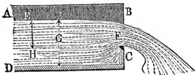
section  $F'$  of the stream passing over the sill  $C$  is a notable fraction of the cross-section  $G$  of the approaching water. The overfall may extend over but a portion or over the whole of the canal or ditch. In the
