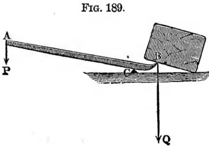
down with a force  $P$  of 60 pounds, and if the arm  $C A$  of the power is 12 times as great as the arm  $C B$  of the load, then the latter, or rather the force  $Q$  developed in  $B$ , is 12 times as great as  $P$ , and we have
