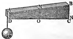
Instead of the parabolic girders, Fig. 405, we generally make use of girders, Fig. 409, with plane surfaces. In order to economize as much material as possible the girder is made in the middle  $M$  of the same height  $MO = h_m = h \sqrt{\frac{1}{2}}$ , as the parabolic girder would have been, and the limiting plane surface  $CD$  is made tangent to the corresponding parabolic surface. We have
