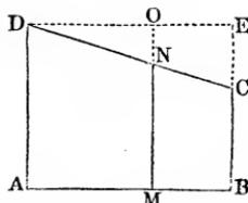
cities, the equal portions  $B E$  and  $M O$ , which are equal to the line  $A D$  representing the initial velocity, there remain the pieces  $C E$  and  $N O$ , which represent the increase or decrease in velocity; for these we have from what precedes the proportion
