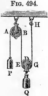
work done is therefore  $P s - (Q + G_1) \frac{s}{2}$ . Now if in sinking the weight  $P$  has acquired the velocity  $v$ ,
