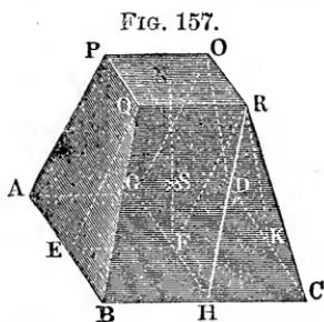
contents of the parallelepipedon are then =  $b_2 l_2 h$ , and its moment is  $b_2 l_2 h \cdot \frac{h}{2} = \frac{1}{2} b_2 l_2 h^2$ . The contents of the two triangular prisms are
