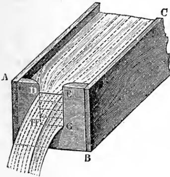
which the efflux takes place, is rectangular; let us denote its width  $D E = G H$  by  $b$  and its height  $D H = E G$  by  $h$ . If we decompose this surface  $b h$ , by horizontal lines, into a great number  $n$  of horizontal strips of equal width, we can consider the velocity to be constant for each of them. Since, if we proceed from above downwards, the heads of water of these strips are
