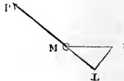
through the space  $MO = x$ , we call the projection  $ML = s$  of this space  $x$  upon the direction of the force  $MP$  the *space described* by the force  $P$ , and the product  $Ps$  of the force by the space is the
