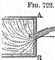
when they are inserted into the vessel at right angles or cut off at right angles to their axis; for in this case the direction of the water is changed. The author's extended experiments upon this subject have led to the following conclusions. If  $\delta$  denotes the angle  $LKN$ , formed by the axis of the tube
