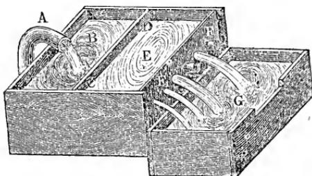
is discharged from the pipe *A* into a box *B*, from which it passes through holes, made in the partition *C D* below the level of the water, into the box *E*; from it the water is discharged through circular orifices *F* one inch in diameter, which are cut out of sheet iron, into the
