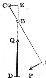
chinery. The knee lever  $ABCD$ , Fig. 188, which is sometimes cited as a peculiar sort of lever, is simply a bent lever. The arm, which is movable around an axis  $C$ , is acted upon by a force at its
