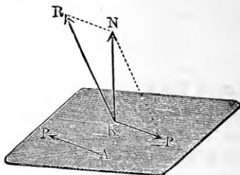
a resultant  $R$ , Fig. 123, and a couple  $(P, -P)$  by decomposing the resultant  $N$  of the parallel forces into the forces  $-P$  and  $R$ , one of which is equal, parallel and opposite to the resultant  $P$  of the forces in the plane.
