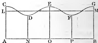
drawn parallel to  $AB$ , cuts off the same space as the serpentine line, then  $LM$  is also the axis of  $CDEF G$ , and the distance  $AL = BM$  between the two parallels  $AB$  and  $LM$  is the mean velocity of the periodic motion, and, on the contrary,  $AC$ ,  $OE$ ,  $BG$ , etc., are the maximum, and  $ND$  and  $PF$  the minimum velocities of a period  $AO$ ,  $OB$ , etc.
