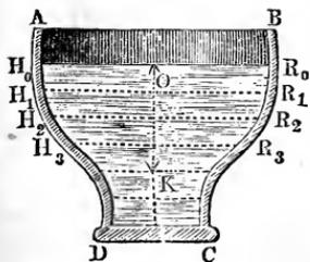
that the area of the surface  $H_0 R_0$  of the water is  $F_0$  and that a pressure  $P_0$  is exerted uniformly upon it, e.g. by the atmosphere lying above it or by a piston, and let us imagine the entire mass of water to be divided by very many horizontal planes, such as  $H_1 R_1, H_2 R_2$ , etc., into equally thick layers.
