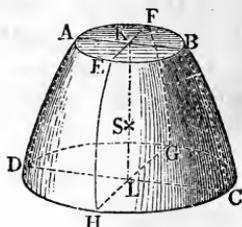
tion of two planes of symmetry  $ABCD$  and  $EFGH$ .
