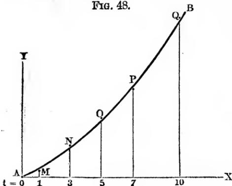
If we consider the times ( $t$ ) as abscissas, and lay off the calculated as well as the observed spaces ( $s$ ) as ordinates, we can draw a curve through the extremities of the calculated ordinates, which will pass between the points  $M, N, O, P, Q$ , determined by the observed co-ordinates, so that the sum of the squares of the deviation of the curve from these points shall be as small as possible.
