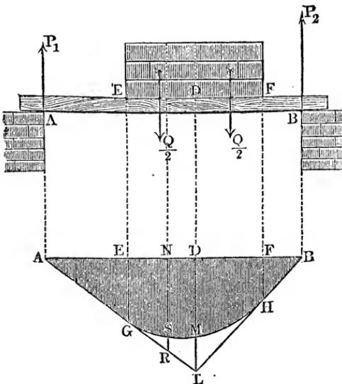
Another case which often occurs in practice is, when the weight is *equally distributed* over a portion  $EF = c$  of the entire length  $l$  of the girder  $AB$ , Fig. 390. Let us again denote the distances of the middle  $D$  of this weight from the points of support  $A$  and  $B$  by  $l_1$  and  $l_2$  and the reaction of the abutments by  $P_1$  and  $P_2$ , then we have again
