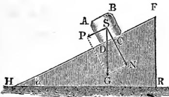
the inclined plane  $F H R$  to the horizon, according to § 146 the normal force is
