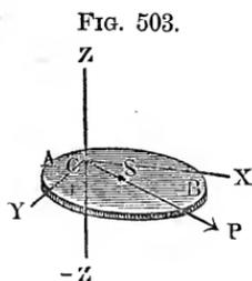
Fig. 503, the centrifugal force is also  $= \omega^2 Mr$ , if  $M$  denotes its mass and  $r$  the distance  $CS$  of its centre of gravity from the axis. If the centres of gravity of the elements of the mass of a body lie in a plane of rotation, or if this plane is a plane of symmetry of the body  $ADFF_1$ , Fig. 504, the centrifugal forces of the elements of the mass of the body can be combined so as to give a
