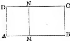
**§ 23.** While in uniform motion the velocity ( $MN$ ) at any moment ( $AM$ ) is the same, in variable motion it is different for each instant; therefore this motion can only be represented by a four-sided figure,  $ABCD$ , Fig. 53, the base of which  $AB$ , denotes the time ( $t$ ), the other boundaries being the three lines,  $AD$ ,  $BC$ , and  $CD$ .
