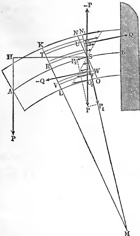
Now if  $x$  is the distance  $SH$  of the cross-section  $NO$  from the point of application  $A$  of the force  $P$ , we have also  $M = P x$ , and consequently
