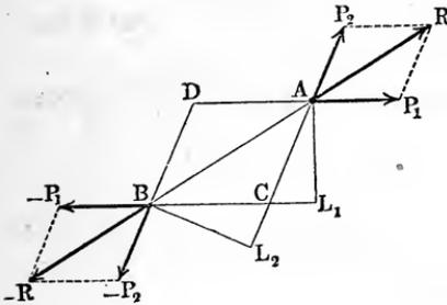
we can combine  $P_1$  and  $P_2$  as well as  $-P_1$  and  $-P_2$  by means of the parallelogram of forces and obtain the resultants. If the directions of these resultants lie in the prolongation of the line  $A B$ , then these forces, and consequently the corresponding couples  $(P_1, -P_1)$ , and  $(P_2, -P_2)$ , balance each other.
