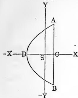
For a *symmetrical parabolic surface*  $A D B$ , Fig. 369, whose cord  $A B = s$  and whose altitude  $C D = h$ , we can put the measure of the moment in reference to the axis of symmetry  $\bar{X} X$
