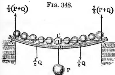
pressure or reaction  $\frac{P+Q}{2}$  at the extremity  $A$ , instead of  $Q$  the load  $-\frac{Q}{2}$ , which is equally distributed upon one-half  $BA$ , and instead of  $l$  half the length of the girder  $\overline{BA} = \frac{1}{2} \overline{AA} = \frac{1}{2} l$ .
