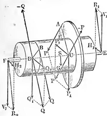
of two pulleys or wheels movable about a common axis. The smaller of these wheels is called the axle (Fr. arbre, Ger. Welle), and the larger the wheel (Fr. roue, Ger. Rad). The rounded ends  $E$  and  $F$ , upon which the apparatus rests, are called the journals (Fr. tourillons, Ger. Zapfen). The axis of revolution of a wheel and axle is either horizontal, vertical or inclined. We will now discuss only the wheel and axle, movable around a horizontal axis. We
