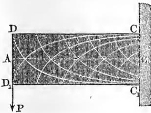
can be represented by two systems of lines, which cut the neutral axis at an angle of  $45^\circ$ , and the outer fibre and each other at an angle of  $90^\circ$ . The curves, which are concave downwards, correspond to the tensile forces, and those which are concave upwards to the compressive forces. The steeper end of any curve corresponds to the minimum and the flatter end, on the contrary, to the maximum forces.
