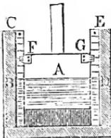
The most simple way of measuring the water in a trough is to place a board *C F*, Fig. 701, beveled at the top, across it and to measure the overfall which is produced. If the ditch or trough is long and nearly horizontal, considerable time will elapse before the flow becomes permanent, and it is, therefore, advisable before beginning
