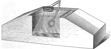
Fig. 1-Dissecting Microscope.
