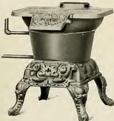
THESE are quick and powerful water heaters. Recommended where it is desirable to use a coal stove for heating water and for laundry purposes; and especially desirable in connection with a gas range. The fire pot is double and the water circulates around it. Connections with the pressure boiler can be made from the back.
