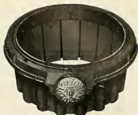
Illustration showing slots which feed air to edges of fire and Hot Blast Ring which supplies oxygen above fire, resulting in the coking of the coal and perfect combustion.
