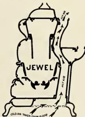
Sectional View Showing the Plan of the Jewel Double Heating Flue
