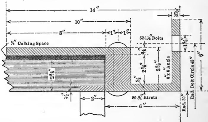
FIG. 66.—Riveted steel coupling collar to connect wood stave pipe with steel pipe. From Bull. No. 155, U. S. Dept. of Agr.
