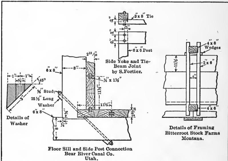
FIG. 38.—Details of framing for wooden flume box.
