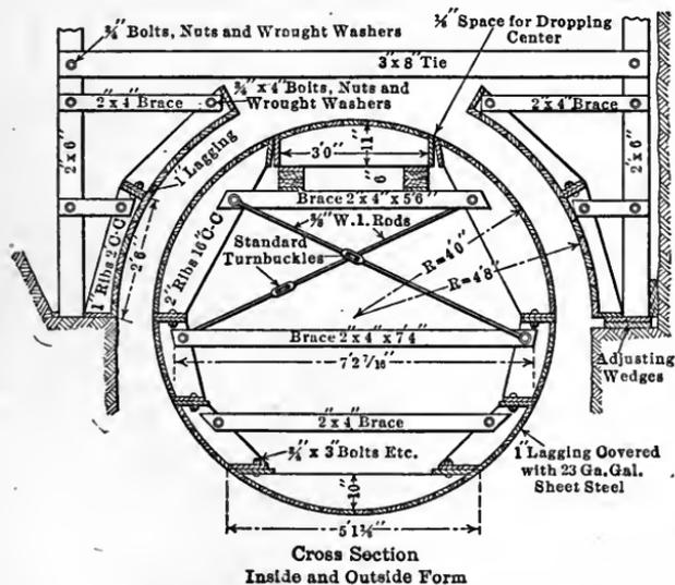
FIG. 72B.—Collapsible inside and outside forms for the construction of Anderson Siphon. Belle Fourche Project, S. D.
