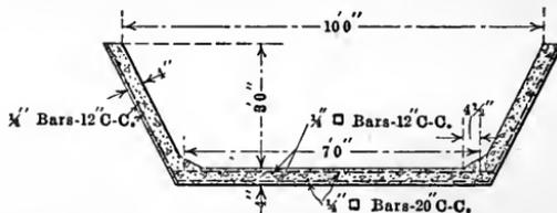
FIG. 23.—Reinforced concrete lining. Yakima Valley Canal, Wash.
