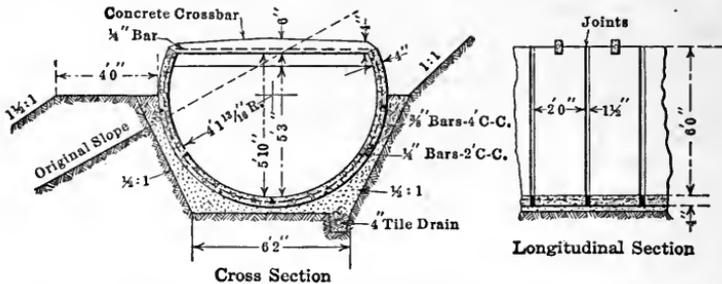
FIG. 24.—Reinforced concrete sectional lining. Tieton Project, Wash.
