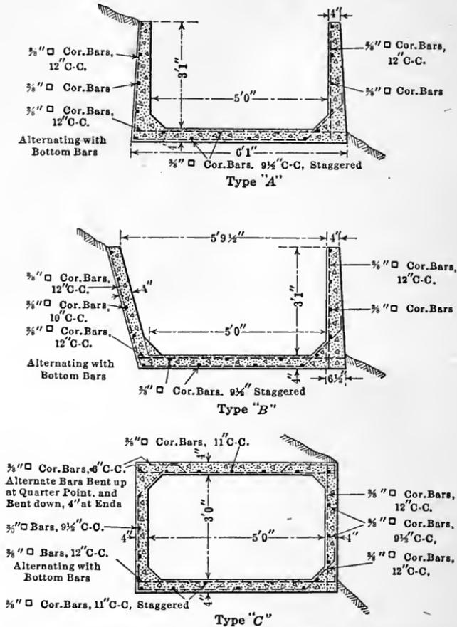
FIG. 30.—Reinforced concrete bench flumes. Yakima Valley Canal Co., Wash.
