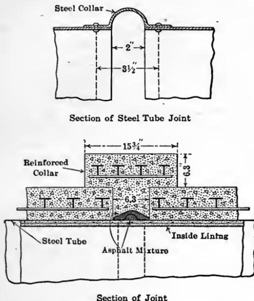
FIG. 75.—Joint of pipes for Sosa Siphon.
