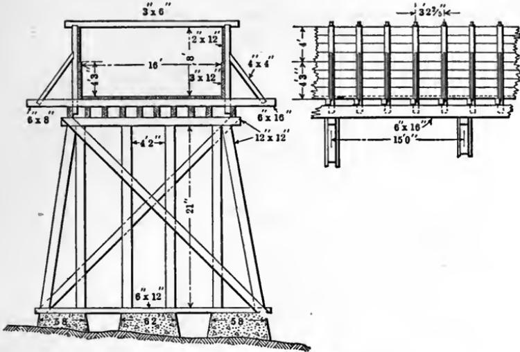
FIG. 35.—Flume of Kern River Power Co., Calif.
