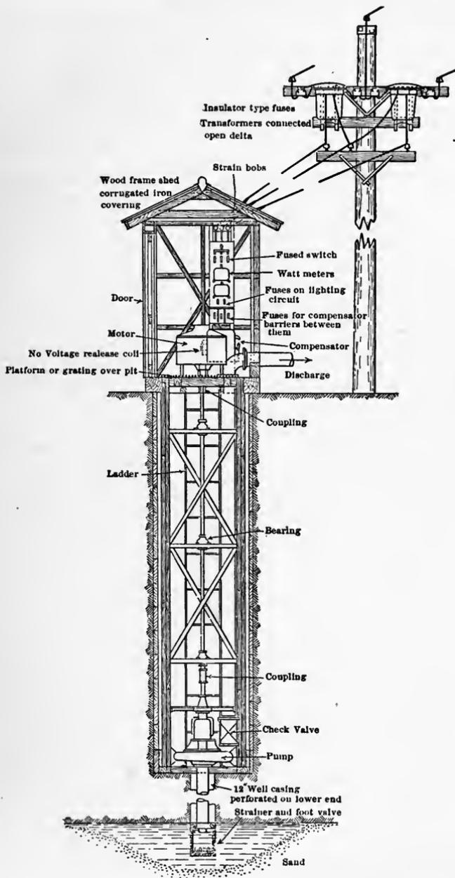
FIG. 71.—Details of vertical pump installation.
