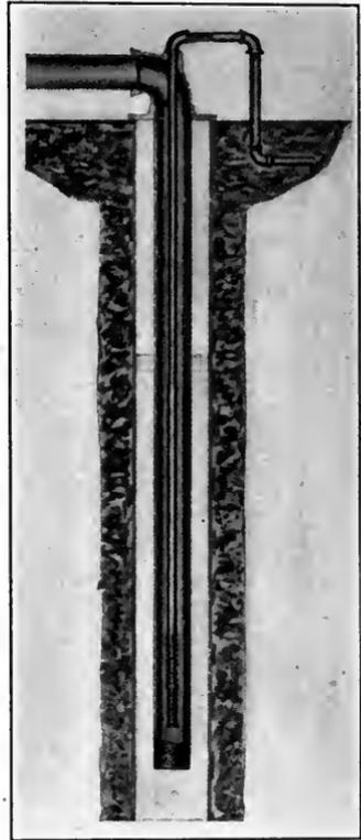
FIG. D.—Air lift pump.
