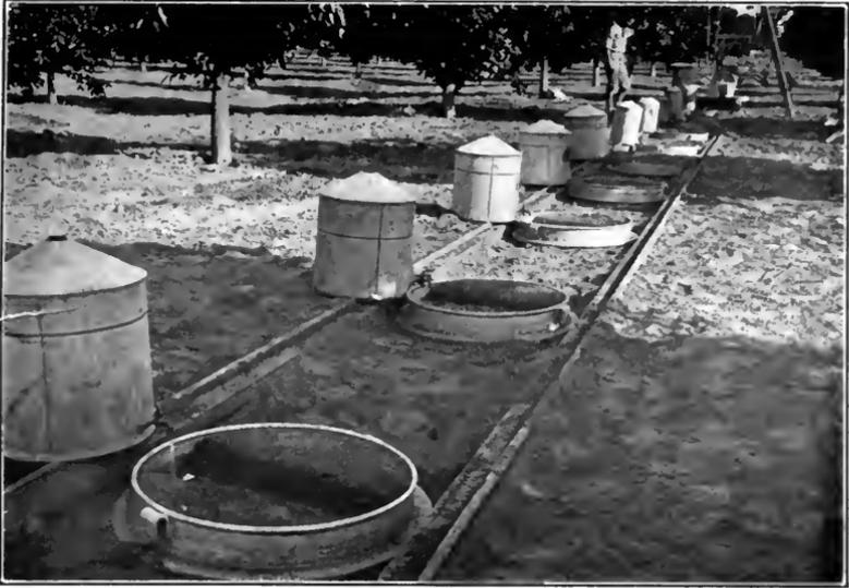
FIG. A.—Tanks used for experiments on soil evaporation.
