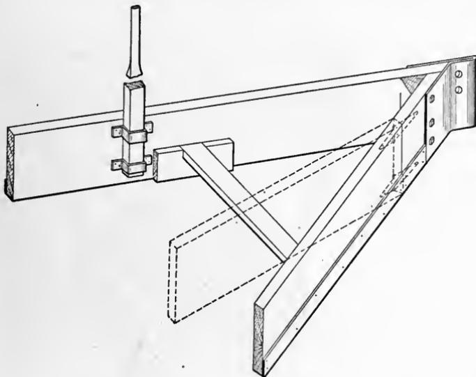
FIG. 52.—V-crowder for making field ditches.
