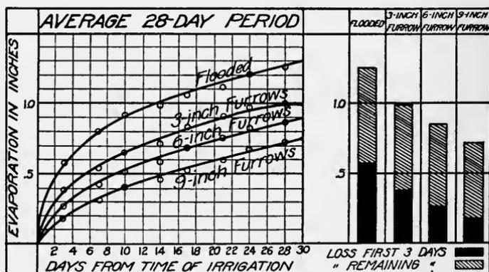
FIG. 4.—Evaporation loss from soils irrigated by flooding and by furrows of different depths. The results are the average obtained at two stations.
