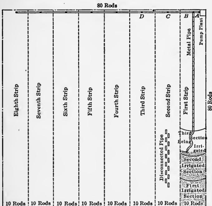
FIG. 47.—The use of slip-joint pipe in applying water to land. From Farmers' Bull. 392, U. S. Dept. of Agriculture.
