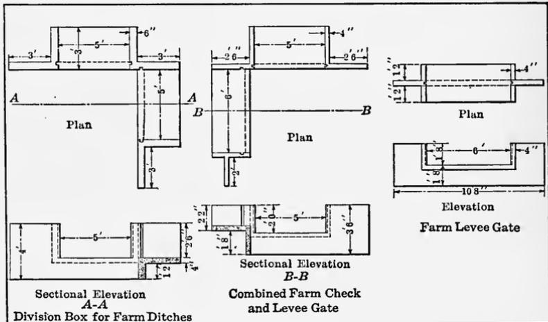
FIG. 63.—Structures on farm distribution system for alfalfa irrigation by border method. University Farm, Davis, Cal.
