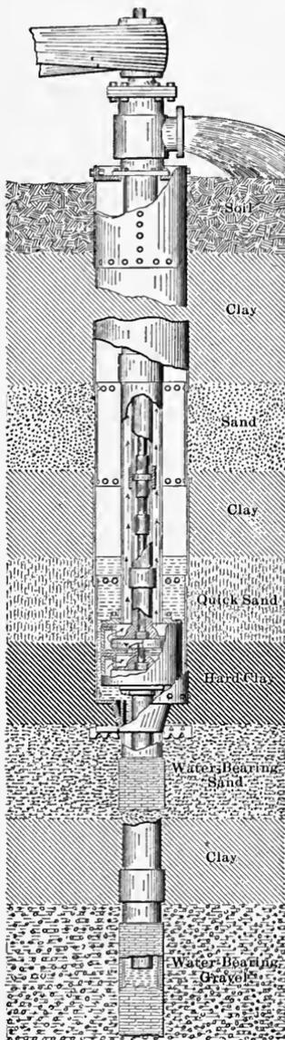
FIG. 72.—Deep well turbine centrifugal pump.
