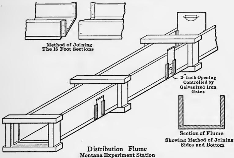
FIG. 41.—Head flume for furrow irrigation.
