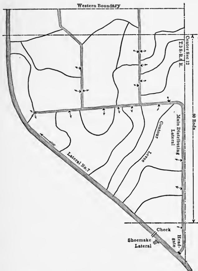
FIG. 32.—Irrigation by contour check system. From O. E. S. Bull. 158, U. S. Dept. of Agriculture.
