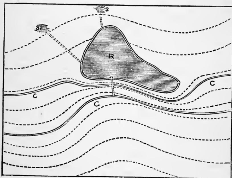
Fig. 54.—THE SPRINGS COLLECTED INTO A POOL.
