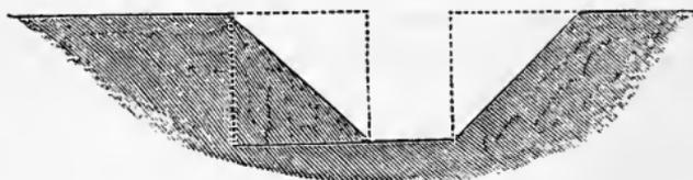
Fig. 123.—SLOPE OF "ONE FOOT IN ONE."
