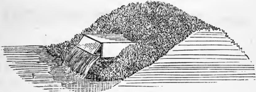
Fig. 59.—SELF-ACTING WATER GATE.
