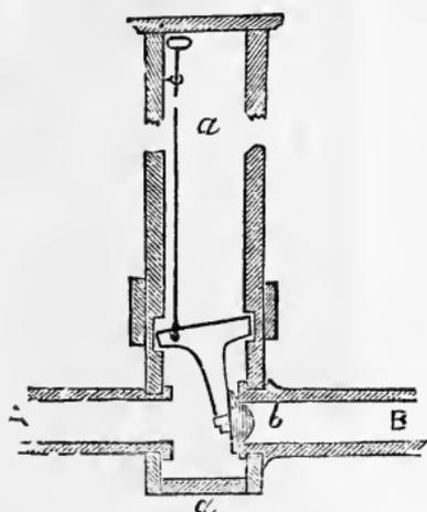
Fig. 76.—PLUG FOR CLOSING DRAIN.
