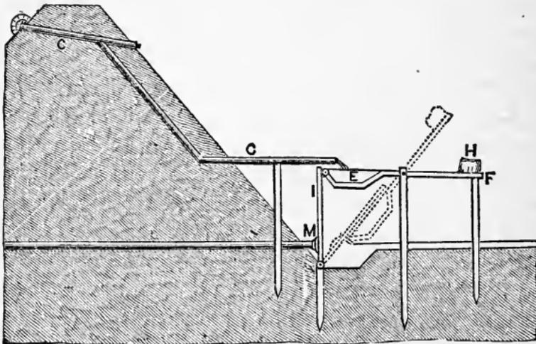
Fig. 46.—TRAP FOR DISCHARGING RESERVOIR.
