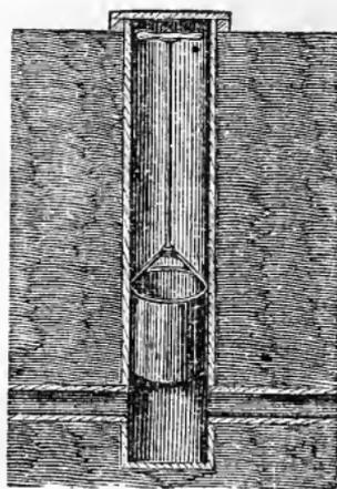
Fig. 77.—A CURVED DRAIN-STOPPER.
