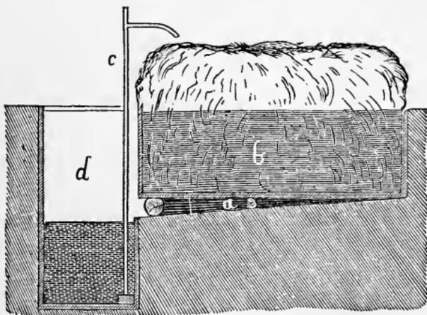
Fig. 30.—LIQUID MANURE TANK.
