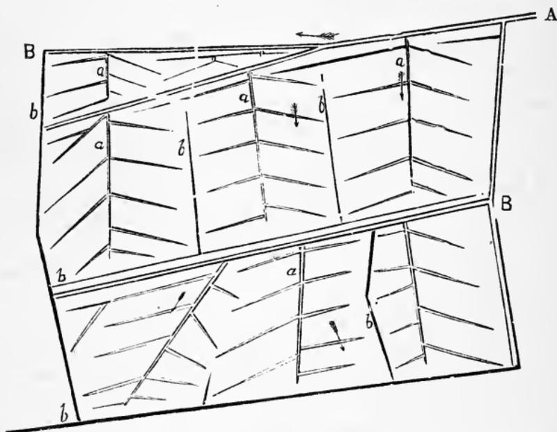
Fig. 70.—FURROWS AND DRAINS FOR IRREGULAR SLOPES.
