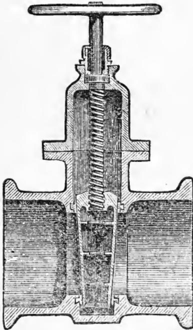
Fig. 115.—DISCHARGING PIPE VALVE.
