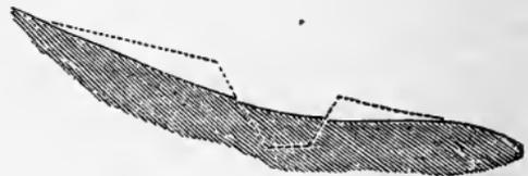
Fig. 135.—CANAL ON A HILL-SIDE.
