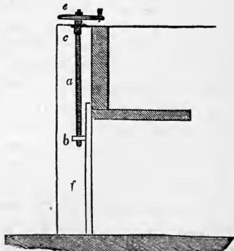
Fig. 130.—SECTION OF GATE.
