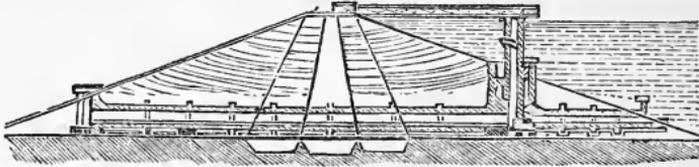
Fig. 114.—DAM WITH CULVERT AND TOWER.
