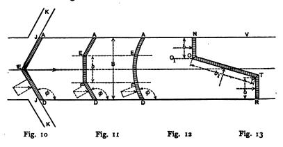
2. The weir is like the preceding but the two diagonal sections are separated by a central portion  $\overline{EF}$  normal to the direction of flow, as in Fig. 11.
