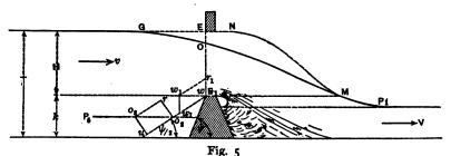
velocity v; that all the water in the channel must flow over the weir; that the weir is horizontal and has an inclined upstream face;
