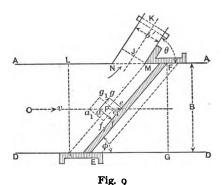
The water over the weir crest, having a depth H, quantity BHv, and a velocity of approach v exerts an hydrodynamic pressure against the weir section equal to
