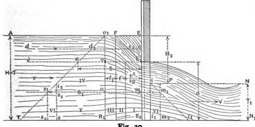
approach impinging on the discharge area and on the wing walls and upper portion of the gate. Hence, the expressions just found will apply to the present case when k = o is introduced.
