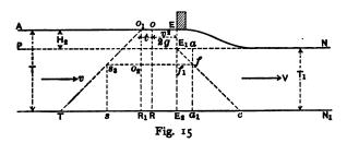
The hydrodynamic pressure, due to velocity of approach and deflected into the discharge area by the piers, is represented by the rectangle  $\overline{OO_1R_1R}$ , the width of which is
