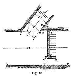
In Fig. 26, let  $\overline{EF}$  represent a spillway, with regulating gate at  $\overline{GM}$ , both normal to the flow of the river.  $\overline{JK}$  is a lateral diversion channel making the angle  $\theta$  with the axis of the river.
