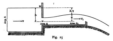
at such a point where the parallelism of the filaments of flow is again established. Taking areas, velocities and heights as indicated in the figure, then from the principle of the conservation of energy, the following equation may be written out:
