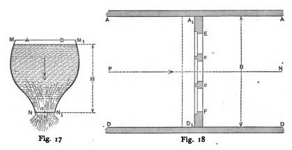
ally contracted into a conical shape, so that the velocity V, in the enlarged section  $\overline{M_1M}$ , is gradually accelerated toward the opening  $\overline{N_1N}$ . The water in falling, through the height H, acquires a certain vis viva, none of which is supposed to be lost in the production of acceleration.\*
