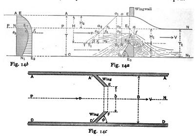
Fig. 14a represents the longitudinal section of a river or canal, obstructed by a submerged weir and wing walls  $\overline{A'E}$  and  $\overline{D'F}$ , shown in plan Fig. 14c. All dimensions are indicated on the two figures.
