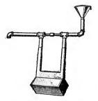
The Minnetonna Ripening Coil enables you to get this ripening process done just right. First clean and scald out the barrel of the Minnetonna Home Creamery thoroughly. After having cleaned the barrel thoroughly, pour in the cream, first having taken out the shelf—put in the ripening coil, and fill it with hot water, not too hot, but about 90 degrees.
