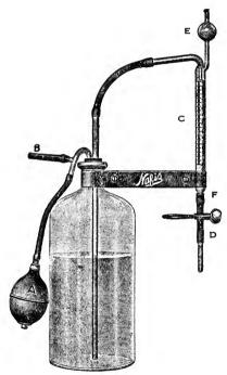
The pinchcock (D) when pressed between the fingers, allows the neutralizer to run out of the burette as slow or as fast as desired.
