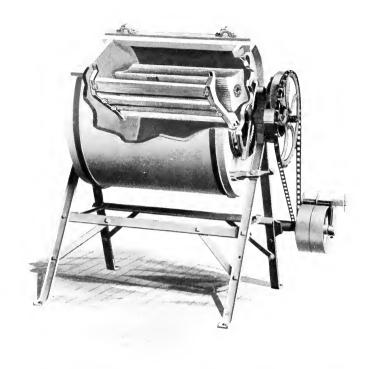
No. 2C Minnetonna Home Creamery, with part of side and one end cut away to show the position of shelf and working roll inside of ALL Minnetonnas. Churning capacity (barrel half full), 22 gallons. Working capacity, 5 to 50 pounds.
