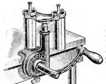
One of the several styles of Babcock Testers sold by the Minnetonna Company. The hand-operated testers are also made for 4 bottles. Electric-operated testers made for 2 to 12 bottles. See Dairy Supply catalog of the Minnetonna Company.
