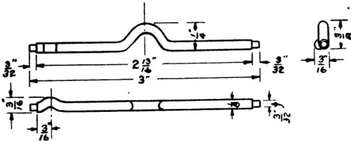
FIG. 148.—Details of the Shaft.
