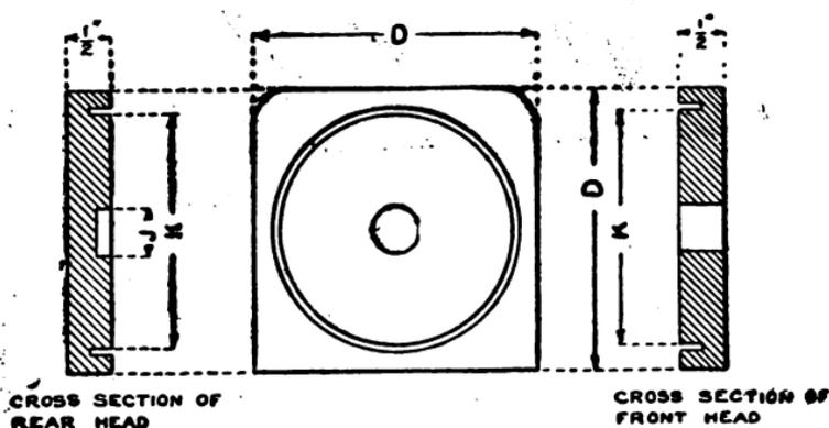
FIG. 113.—Details of the Wooden Coil Heads.
