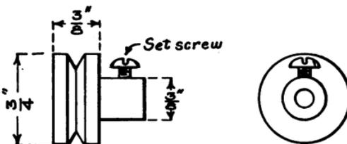
FIG. 130.—The Pulley.
