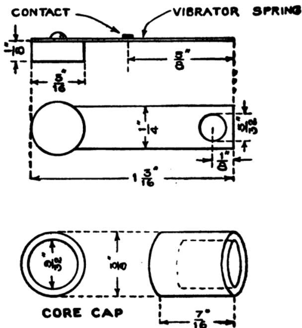
FIG. 101.—Vibrator Parts and Core Cap.
