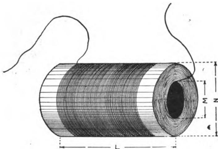
FIG. 111.—The Secondary Winding.
