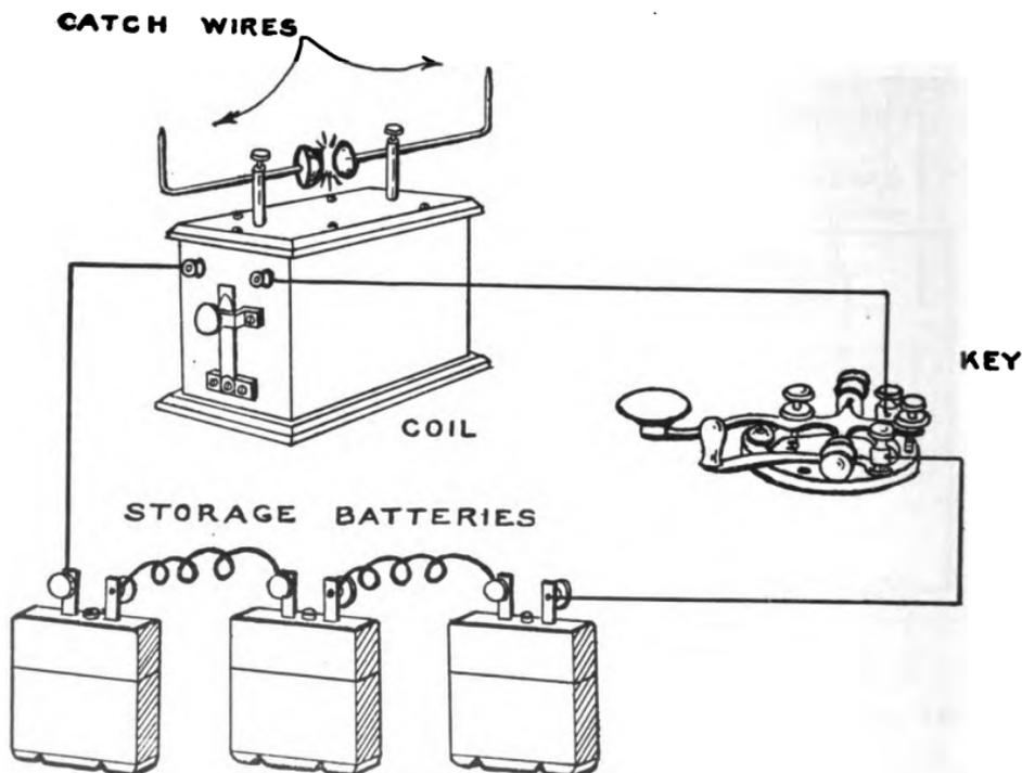
FIG. 167.—How the Transmitter is Connected.
