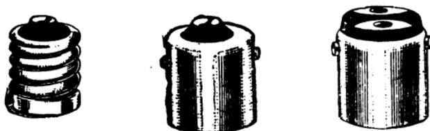
FIG. 154.—Showing the differences between the Candelabra, Single Ediswan and Double Ediswan Types of Lamp Bases.
