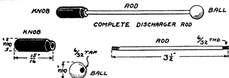
FIG. 12.—Details of the Discharger Rods.
