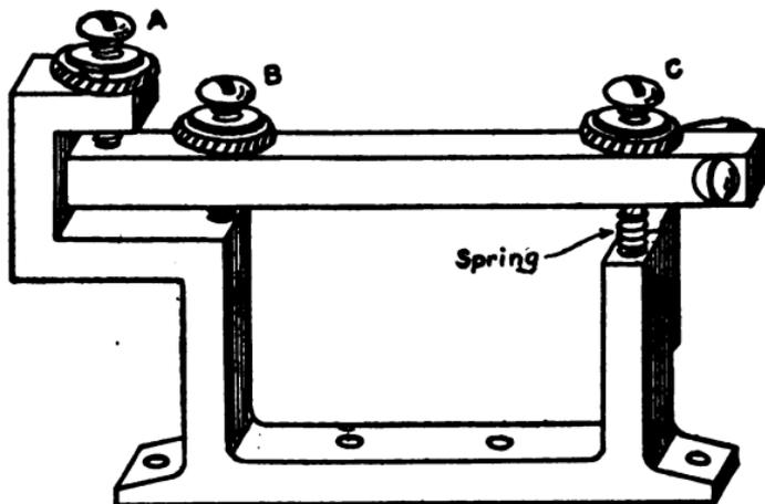
FIG. 87.—Sounder Frame with Lever in Position.
