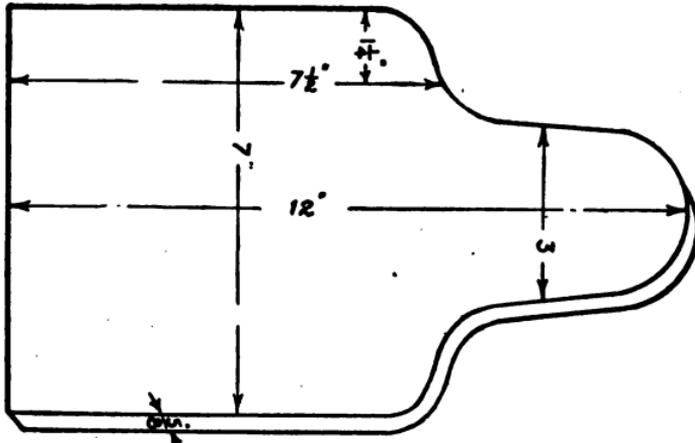
FIG. 93.—The Wooden Back for the Telephone.
