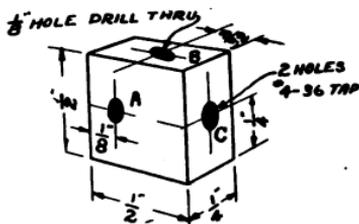
FIG. 142.—The Fibre Block for supporting each Brush.
