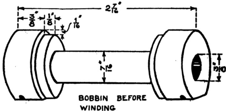
FIG. 98.—Bobbin for Medical Coil.
