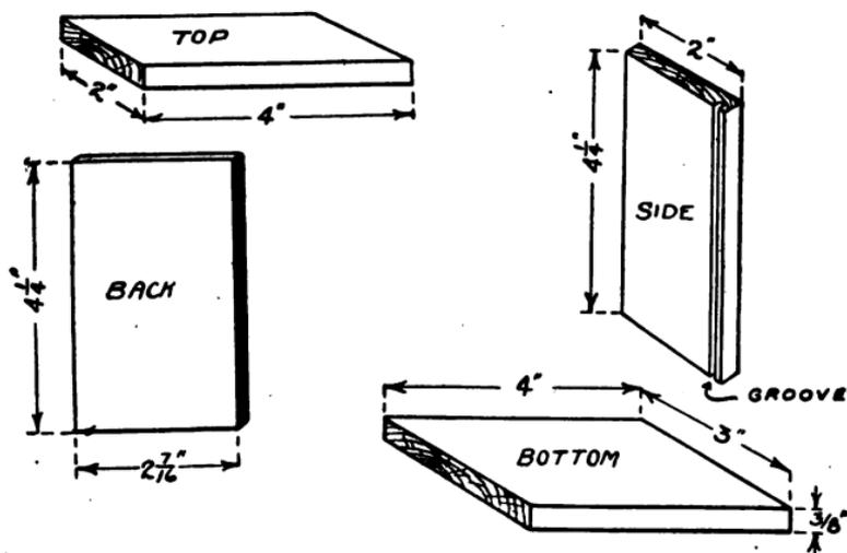
FIG. 73.—Details of the Wooden Parts which form the Case.
