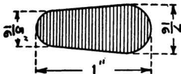
FIG. 3.—The details of the Tinfoil Sector. Sixteen are required for each plate. They are stuck to the plates with shellac.
