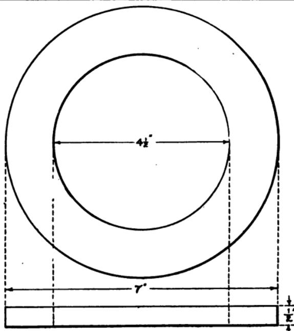
FIG. 173.—Details of the Primary Head.
