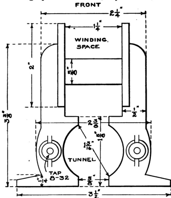
FIG. 123—Front view of the Field Casting.
