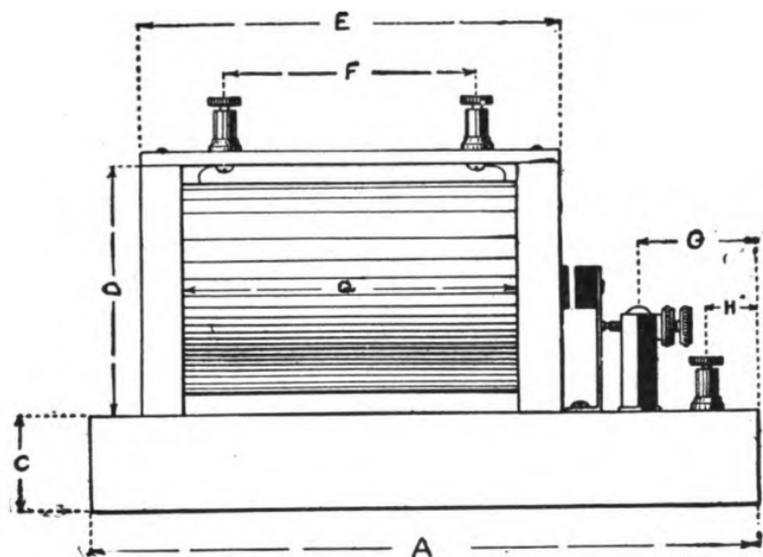
FIG. 120.—Side View of the Completed Coil.
