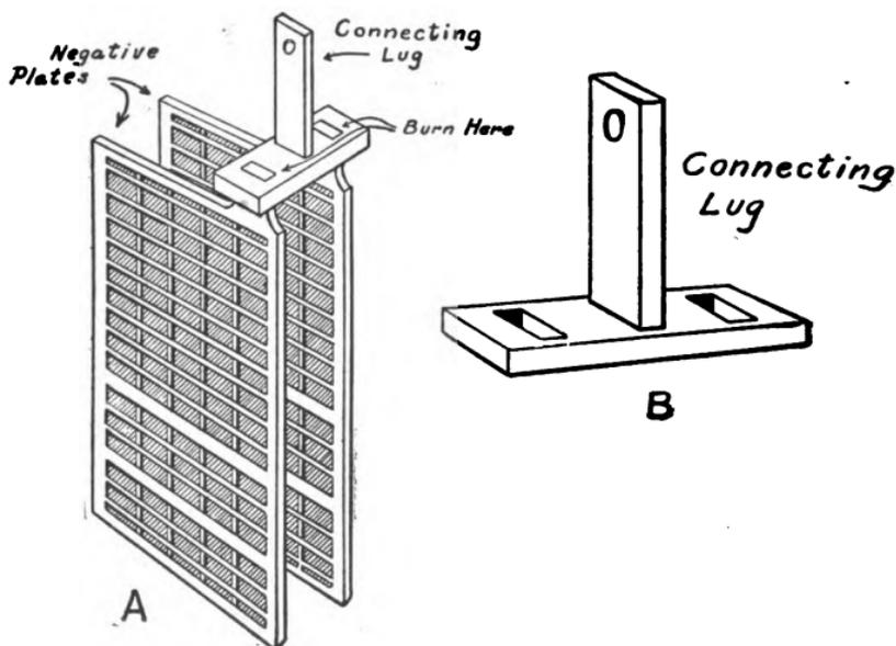
FIG. 43.—Two Negative Plates "burned" together and the Connecting Lug used.
