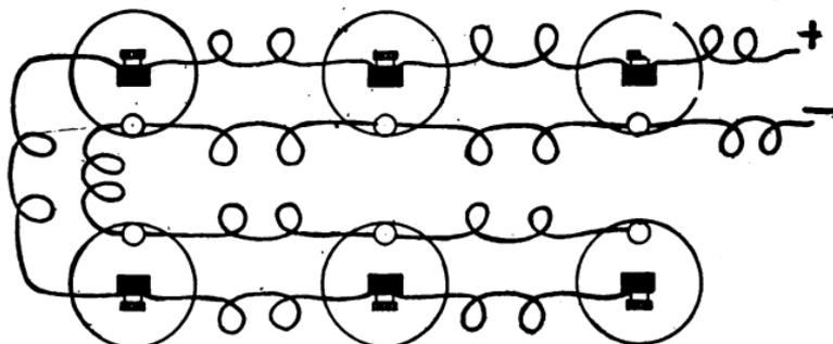
FIG. 34.—Showing Six Dry Cells connected in Multiple. The Voltage of such an arrangement would only be 1.5, but the Amperage available would be six times that possible from Cells connected as in Figure 33.
