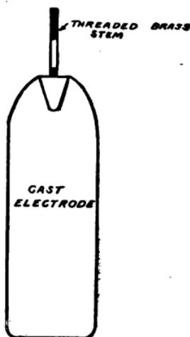
FIG. 51.—A Cast Electrode will last much longer than one cut from Sheet Metal. Cast Electrodes like that above are on the market and can be purchased very reasonably.
