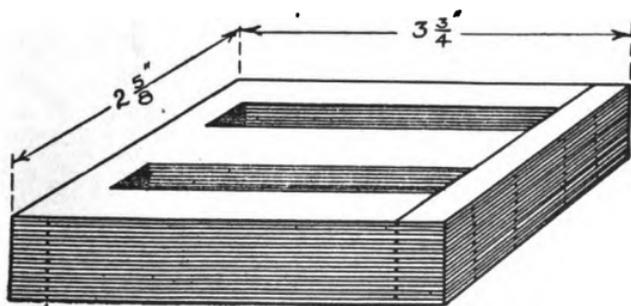
FIG. 60.—Assembly of the Core.
