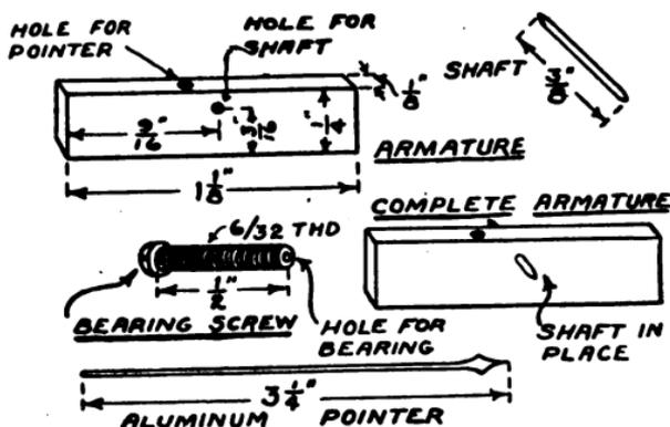
FIG. 69.—Details of the Armature, Bearings and Pointer.
