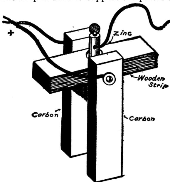
FIG. 29.—A Home-made Battery having two Carbon Plates with a Zinc Rod between.
