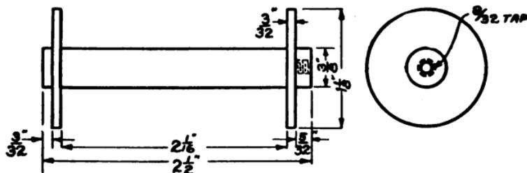
FIG. 145.—Details of the Electromagnet Bobbin.
