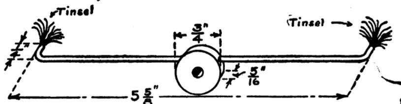
FIG. 14.—The Neutralizers. Two are required. They are bent out of Brass Rod and fitted with a Tinsel Tuft at each end. The centre piece upon which the Rod is mounted should be of Hard Rubber.
