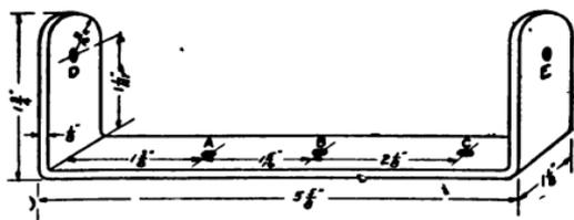
FIG. 146.—Details of the Engine Frame.
