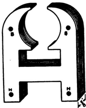
FIG. 135.—The Assembled Field ready for Winding.
