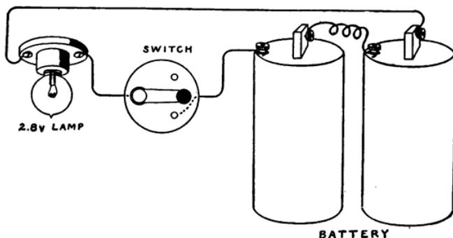
FIG. 156.—Connections for a 2.8 Volt Lamp.
