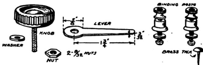
FIG. 81.—The Lever, Knob, Binding Posts, etc.
