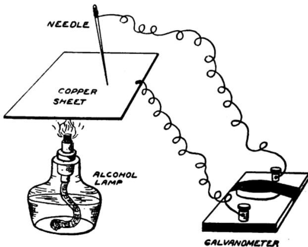
FIG. 187.—Generating Electric Current by Heat.
