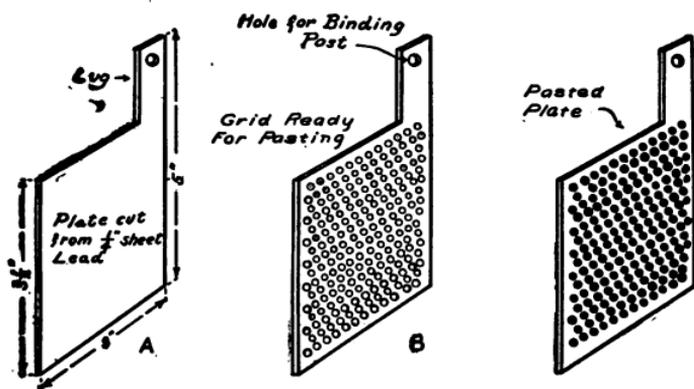
FIG. 39.—Showing how the Plates for a Storage Cell may be made from Sheet Lead by boring it full of holes and filling with paste.
