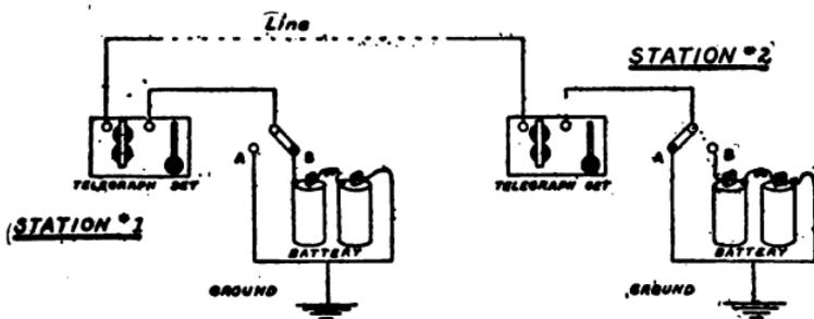
FIG. 92.—Circuit for Two Instruments.
