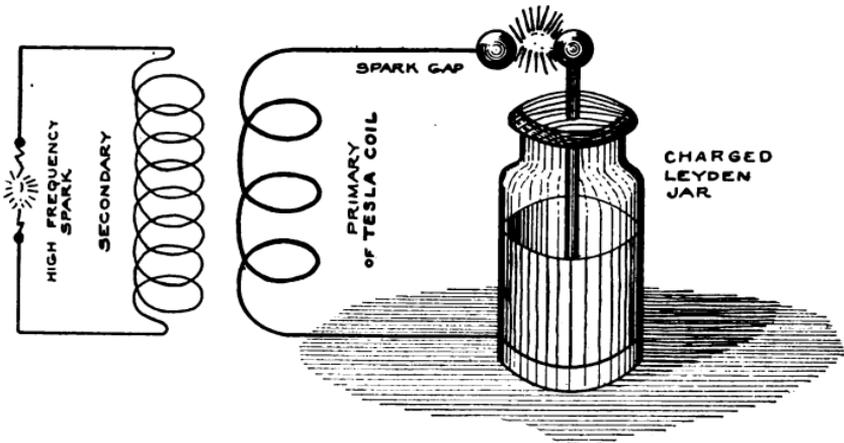
FIG. 170.—Telsa Coil Circuits.
