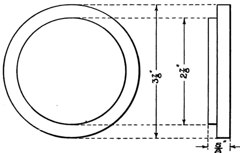
FIG. 172.—Details of the Secondary Heads.
