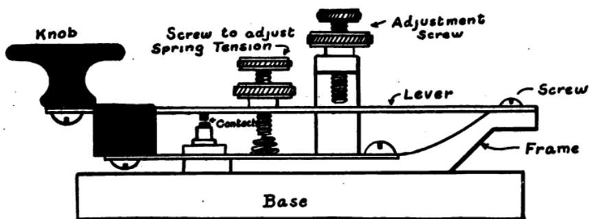
FIG. 89.—Side View of Key.
