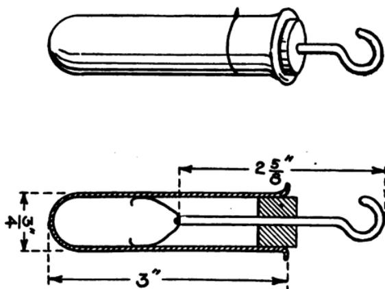
FIG. 15.—Details of the Leyden Jars. They are simply small Test Tubes, coated inside and outside with tinfoil for about two-thirds their height and fitted with a Brass Rod connected with the inside coating.
