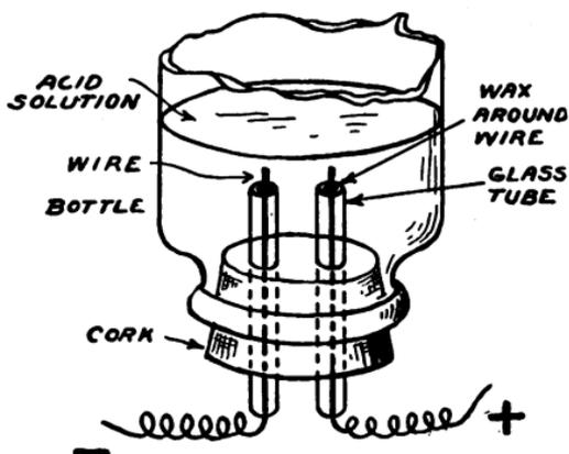
FIG. 185.—Apparatus for Electrolysis Experiment.
