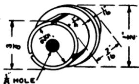
FIG. 138.—The Commutator.
