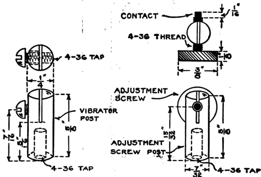
FIG. 106.—Vibrator Parts.
