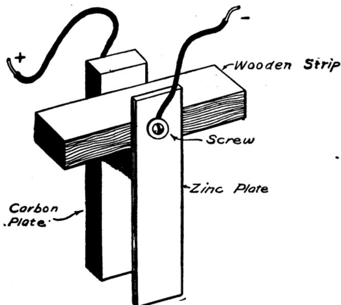
FIG. 28.—A Simple Home-made Cell.
