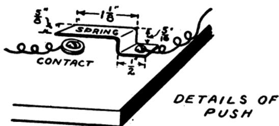
FIG. 96.—Showing how the Push Button is arranged.
