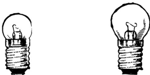
FIG. 152.—Small Tungsten Battery Lamps.
