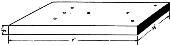
FIG. 144.—The Engine Base.
