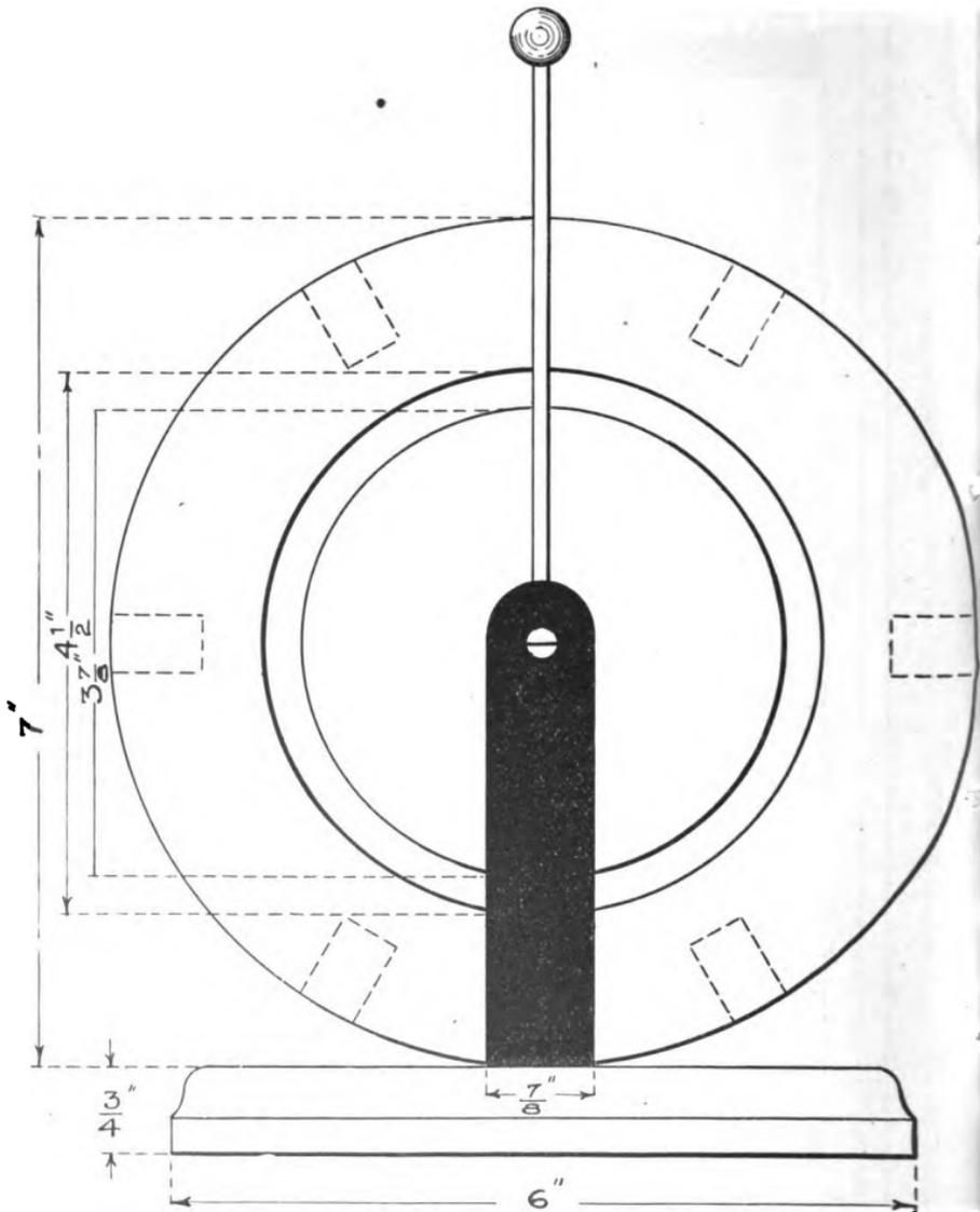
FIG. 176.—Side View of the completed Tesla Coil.
