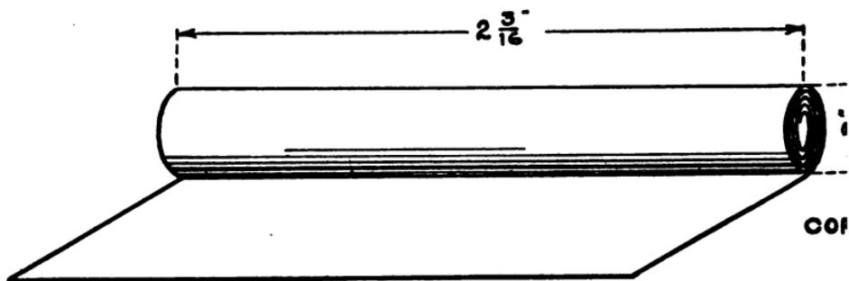
FIG. 100.—Construction of the Core.
