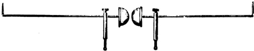
FIG. 168.—The Complete Spark Gap.
