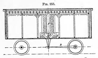
Refrigerating apparatus for transport cars according to Trapp. A, axle; B, belt; C, driving pulley; D, ventilator; E, receptacle for calcium chlorid; F, air shaft; G, ice chest.
