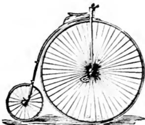
The Hecla Bicycle is the latest and most approved boys' and youths' machine now on the market. The wheels have steel wire spokes and flat iron tires. Front forks are made of solid malleable iron with steel handle rods, hollow tapered back bone, malleable iron hub, and solid steel axle, spring leather seat, no brakes, all main bearings are adjustable. In general appearance it resembles the high priced machines.
