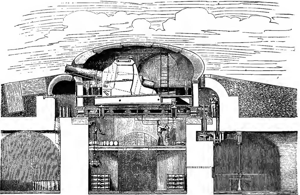
The dome-shaped cupola rests on a wrought iron sub-structure, which rotates on a live roller ring running on a roller path fixed to the foundation, and is protected from shot by a glacis armour.
