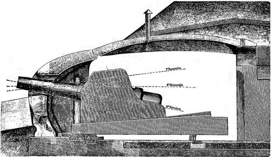
As will be seen from this, an armoured battery forms a spacious structure, which is connected in the rear to the casemates by means of wide passages.
