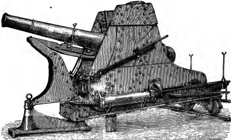
In the smaller carriages the hydraulic ram which elevates the gun is worked by hand-pumps; with the larger ones accumulators are used.
