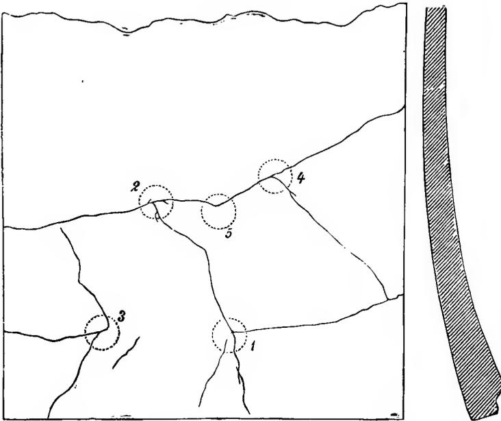
Five hits in all were made ; of these the two first only starred the surface, the third cracked the plate as shown, the fourth cracked the plate into two parts, the fifth made no new crack but extended the previous ones to the under surface, and from crack 4 broke off a piece weighing about 2.2 lb. which fell through.
