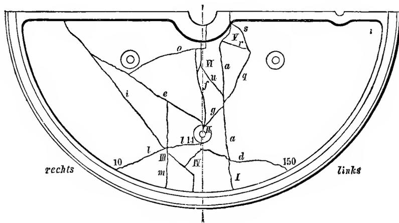
New cracks *n*, *o*, *p*, *d* to the edge of the plate, *h* lengthened to hit 1. The piece of plate bounded by crack *b* was thrust up about 1.4 in.
