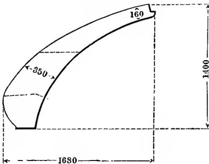
The trial of the Schumann turret had given comparatively favourable results, and as Gruson had offered to construct at less cost one of his turrets of equal resisting powers, it seemed desirable to adopt not only the same programme of trial, but also to follow the thickness given to the wrought-iron plates. In accordance with this, the port plate of the chilled iron turret was given a maximum radial thickness of 13.8 in. (see figure 10), which,
