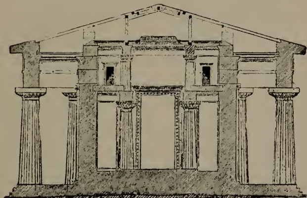
FIG. 13.—SECTION OF THE GREEK DORIC TEMPLE AT PÆSTUM. AS RESTORED BY BÖTTICHER.
