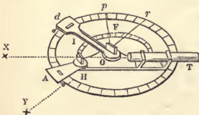
given inclination, and thus at once to bring two objects into contact roughly. The divisions of the finder are reckoned in both directions from the *o*; and when the vernier I, is set to this *o*, the index-glass and horizon-glass are parallel. The telescope-bar can be clamped at pleasure to the circle; so also the index-bar may be clamped either
