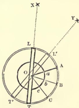
ABC, and carry the telescope round to the other object Y. The index-arm, being clamped to *abc*, is thus carried over an arc AB, which measures the angular distance (XOY) of X and Y. Let it be clamped to
