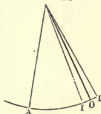
**Index Error.**—The index error of reflecting astronomical instruments, such as the sextant, is the difference between the zero point of the graduated limb, and where the zero point ought to be as shown by the index when the index-glass is parallel to the horizon-glass.
