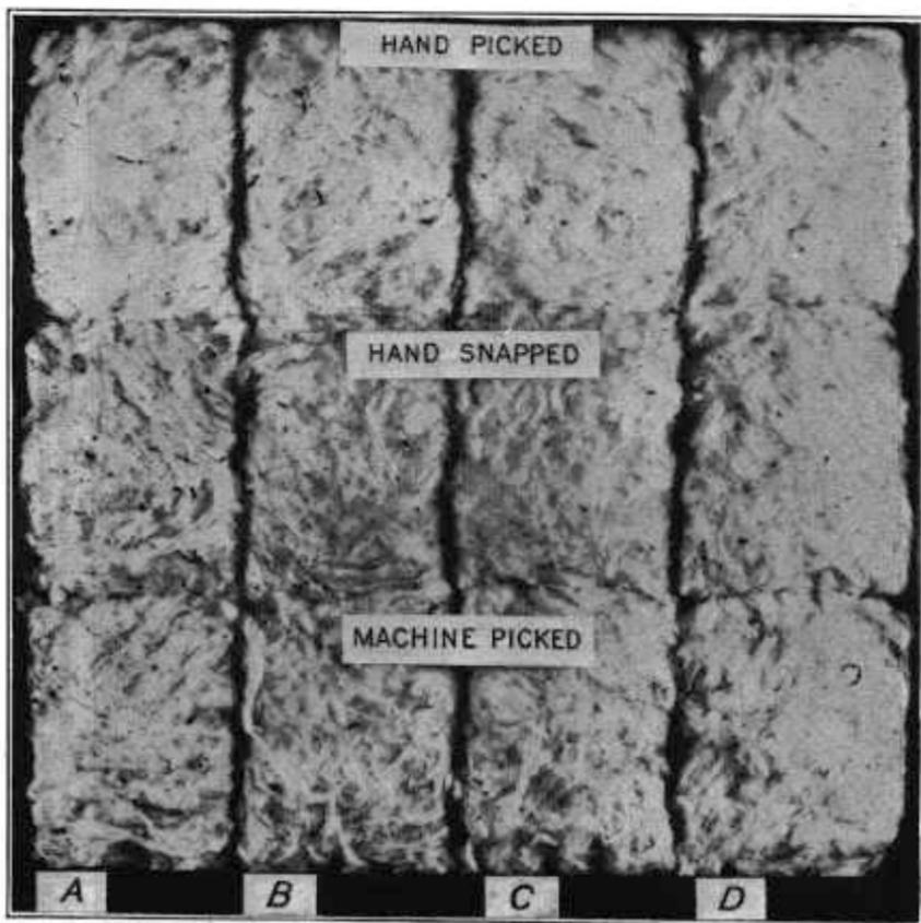
FIGURE 15.—Lint ginned from Mississippi long-staple seed cotton variously harvested, cleaned by different processes: *A*, By revolving-screen separator only; *B*, by revolving-screen separator and 4-cylinder spider-arm cleaner; *C*, by 6-cylinder air-line cleaner, revolving-screen separator, and 4-cylinder spider-arm cleaner; *D*, by 6-cylinder air-line cleaner, revolving-screen separator, 4-cylinder spider-arm cleaner, and unit cleaner-extractor-feeder.
