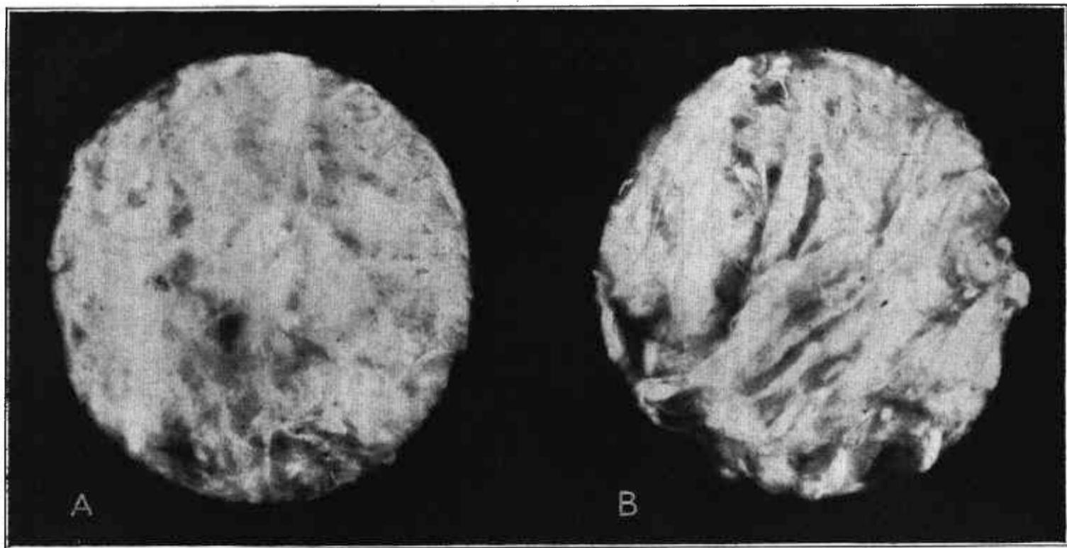
FIGURE 27.—Lint samples of long-staple cotton ginned at a saw speed of 600 revolutions per minute: *A*, With loose seed roll; *B*, with tight seed roll.
