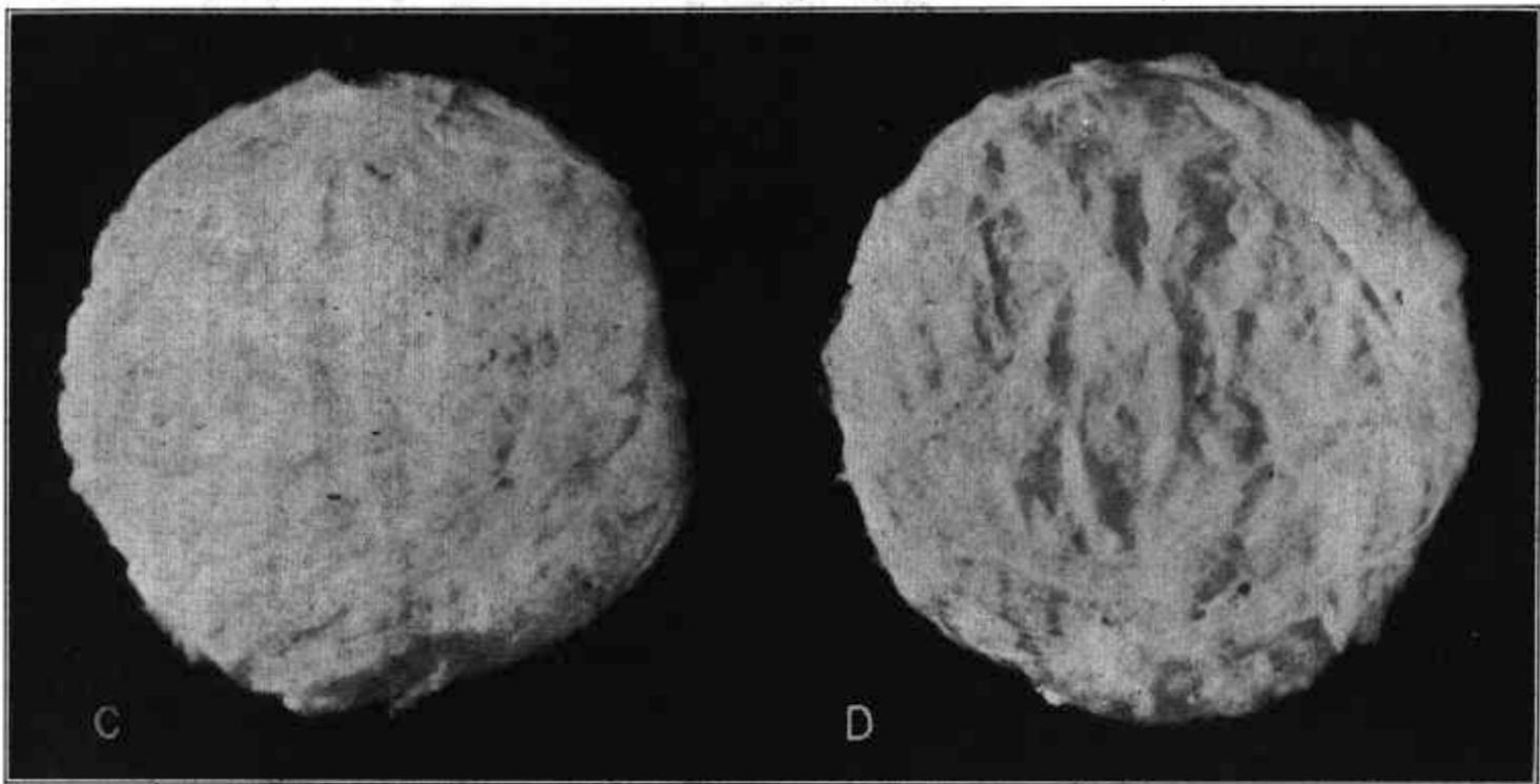
FIGURE 14.—Lint ginned from long-staple seed cotton cleaned by different processes: *A*, By cleaner-separator only; *B*, by 6-cylinder air-line cleaner and cleaner-separator; *C*, by cleaner-separator and unit cleaner-extractor-feeder; *D*, by 6-cylinder air-line cleaner, cleaner-separator, and unit cleaner-extractor-feeder.
