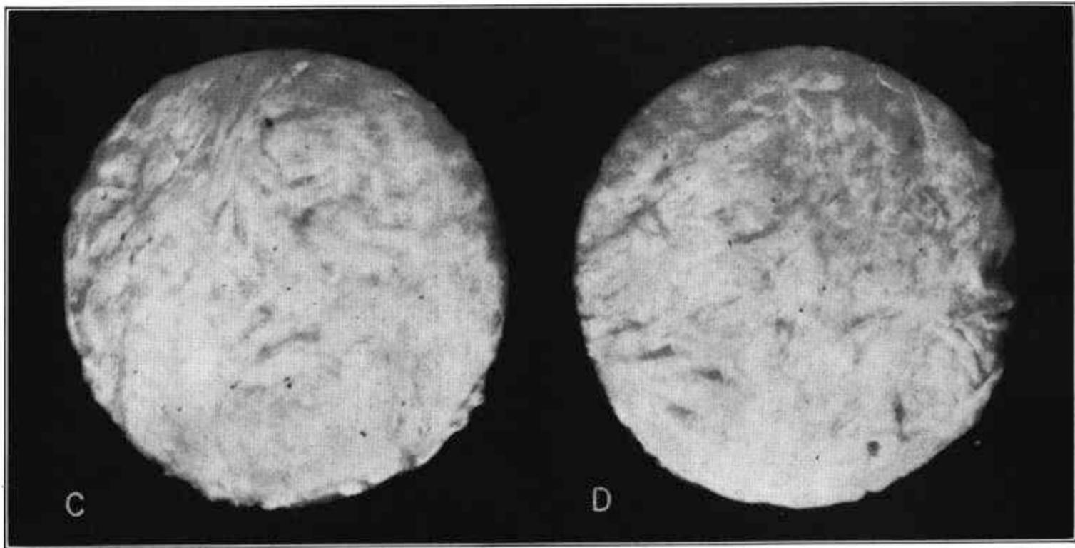
FIGURE 13.—Lint ginned from short-staple seed cotton cleaned by different processes: *A*, By revolving-screen separator only; *B*, by 6-cylinder air-line cleaner and revolving-screen separator; *C*, by revolving-screen separator and unit cleaner-extractor-feeder; *D*, by 6-cylinder air-line cleaner, revolving-screen separator, and unit cleaner-extractor-feeder.
