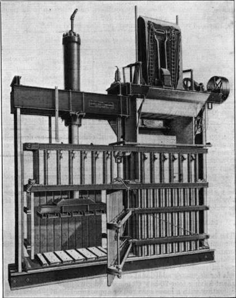
FIGURE 29.—Down-packing single-story double-box all-steel hydraulic cotton press.
